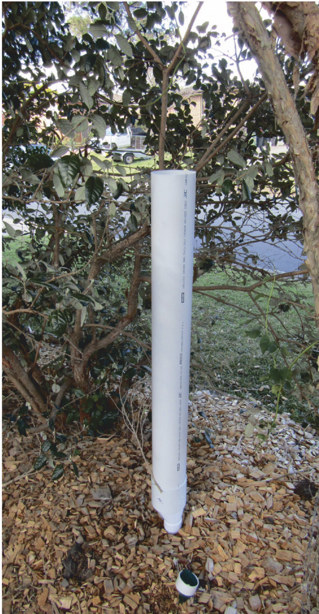
The large diameter PVC pipe will hold lots of grey water and means you don't need to stand around for 15 minutes filling up the deep pipe irrigator you built after Nev's previous story.
