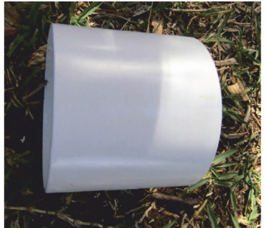
A 100mm PVC straight coupling keeps the taper level invert and the PVC pipe together.
