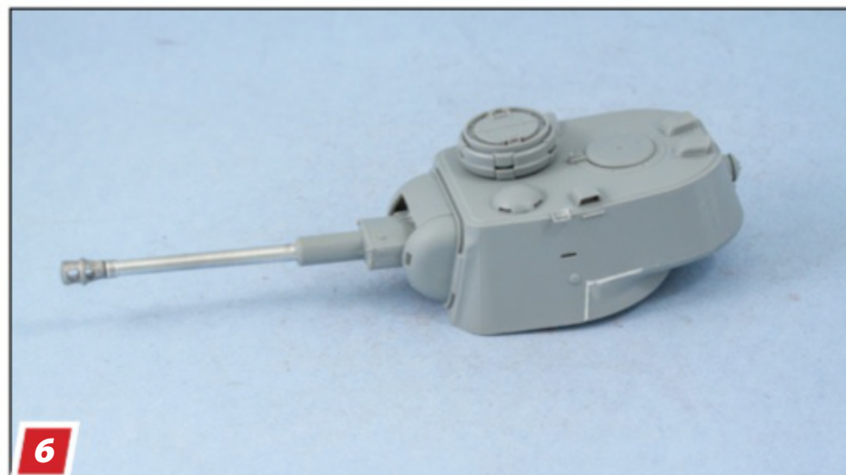
6 Turret assembled with the raised casting seam added.
