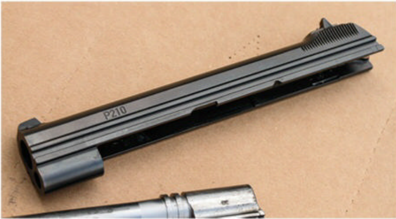
All P210, or M49s, modern or classic, have slide and frame rails that extend the full length of the slide and frame.
