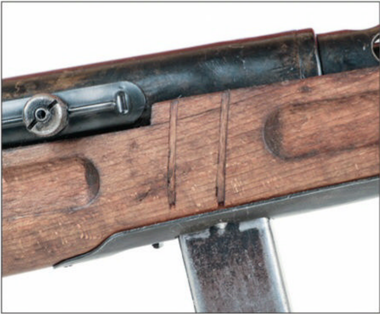
We used to repair things more than we do today. The stocks on this Beretta 38A submachine gun and this DCM M1 have both been repaired by ripping the wood crosswise and then gluing shims in place. Sanding the shims smooth leaves a strong repair that does not interfere with use.
