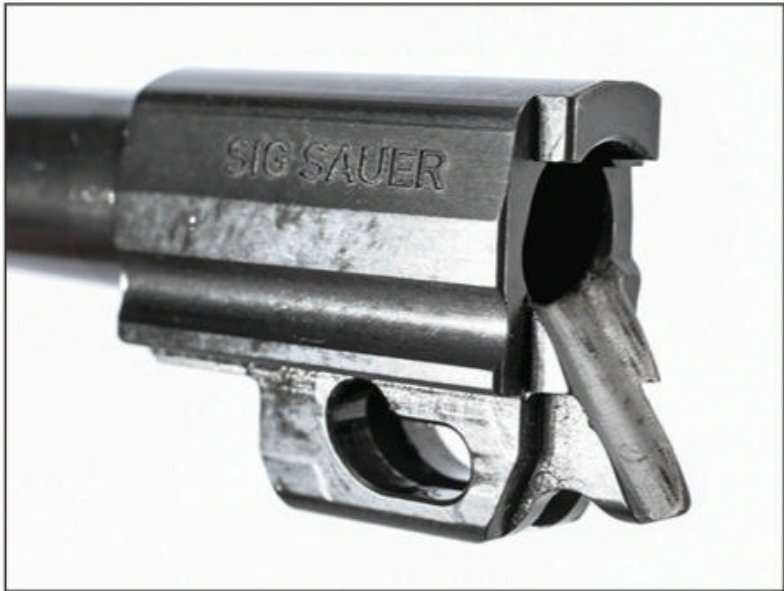
The barrel has an integral feed ramp, and this allows for full case support in the chamber.
