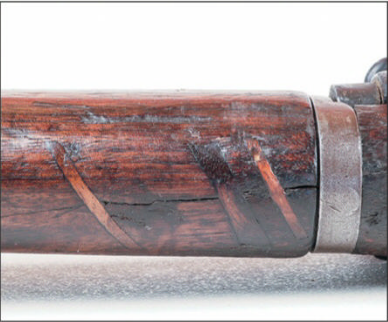
We used to repair things more than we do today. The stocks on this Beretta 38A submachine gun and this DCM M1 have both been repaired by ripping the wood crosswise and then gluing shims in place. Sanding the shims smooth leaves a strong repair that does not interfere with use.
