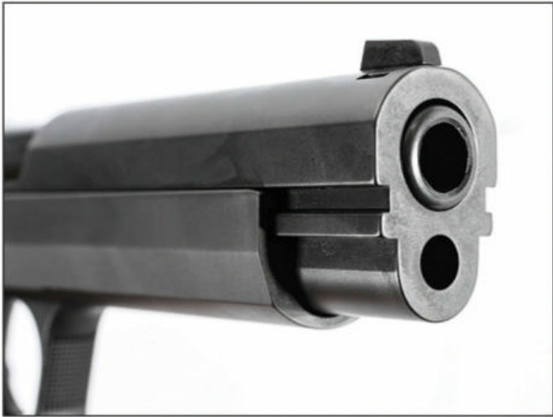
No barrel bushing here. The Swiss didn't see the need for the extra parts and machining operations.
