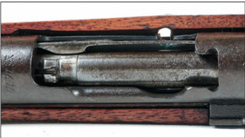
The geometry of the bullet track would have taken it through the rifle's extractor. The lack of associated damage leads me to believe it was hit with the bolt open. When I bought the gun it did not have a bolt.
