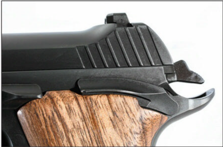
To disassemble you have to hold the slide back a quarter-inch or so. The exact location will vary a bit, it will take some practice to hit the right spot.
