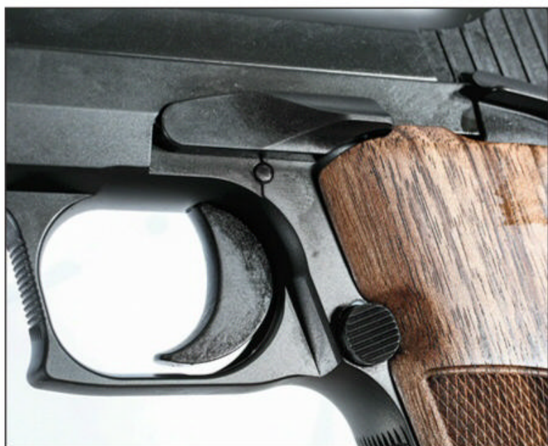
The trigger pivots, attested to by the pivot pin in the frame above the trigger.
