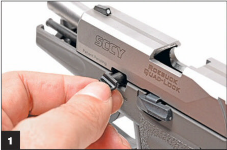
1 Stripping the SCCY pistols is very simple. Start by verifying the pistol is unloaded, remove the magazine and lock the slide back. Then remove the disassembly pin.
