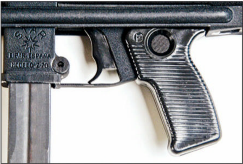
View of the Z-70's magazine release button, two-position trigger, and cross bolt safety; note the "F" for "FIRE" indicating that when the safety button is pushed through from that side the SMG is off safe.
