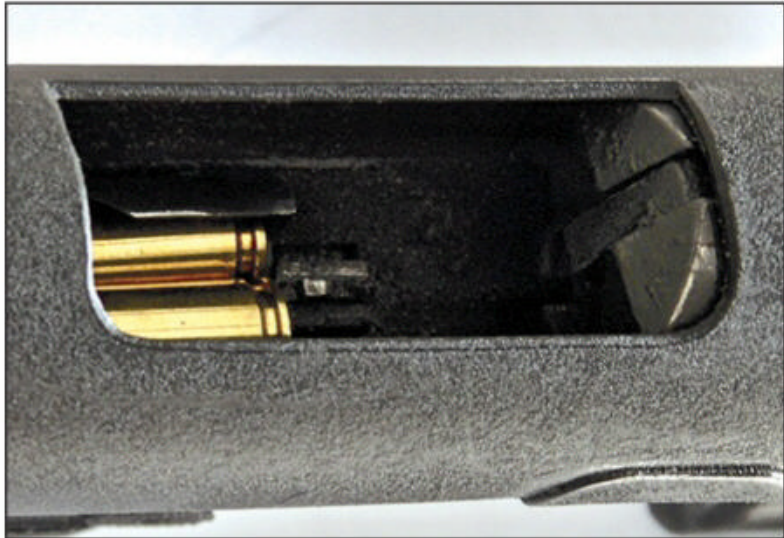
The Z-70 fires from an open bolt.
