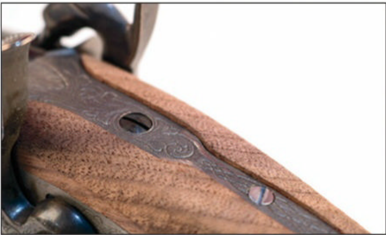
The stocks are left oversized so they can be sanded to suit.
