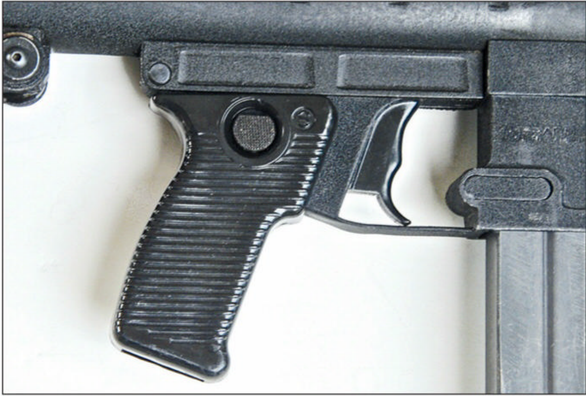
Close-up showing the Z-70's cross-bolt safety and trigger offering two finger positions for full- or semi-auto.
