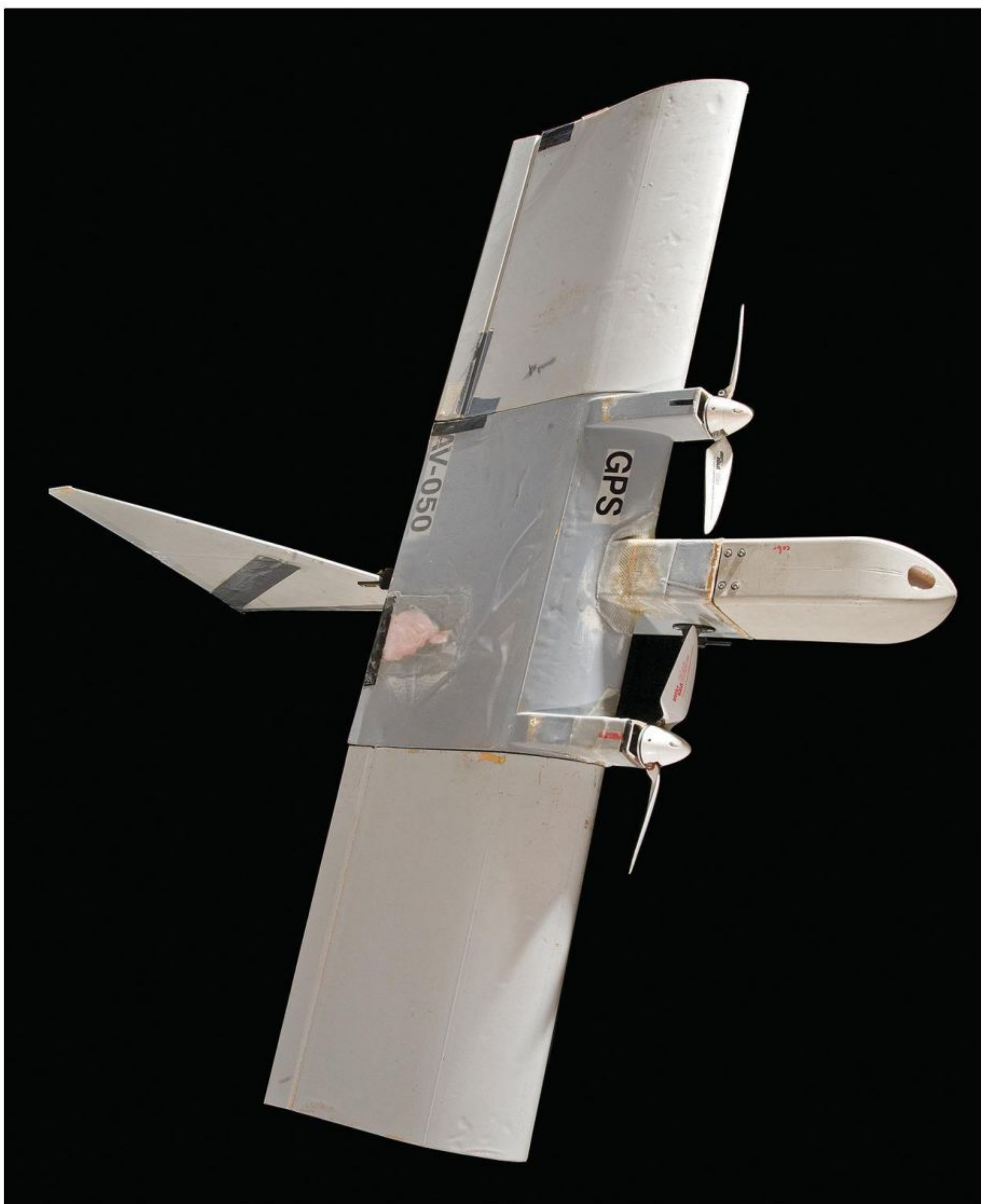
The RQ-14 Dragon Eye in the National Air and Space Museum's collection reveals ample evidence of its service overseas, including a bullet hole patched with epoxy and structural reinforcement using duct tape.
