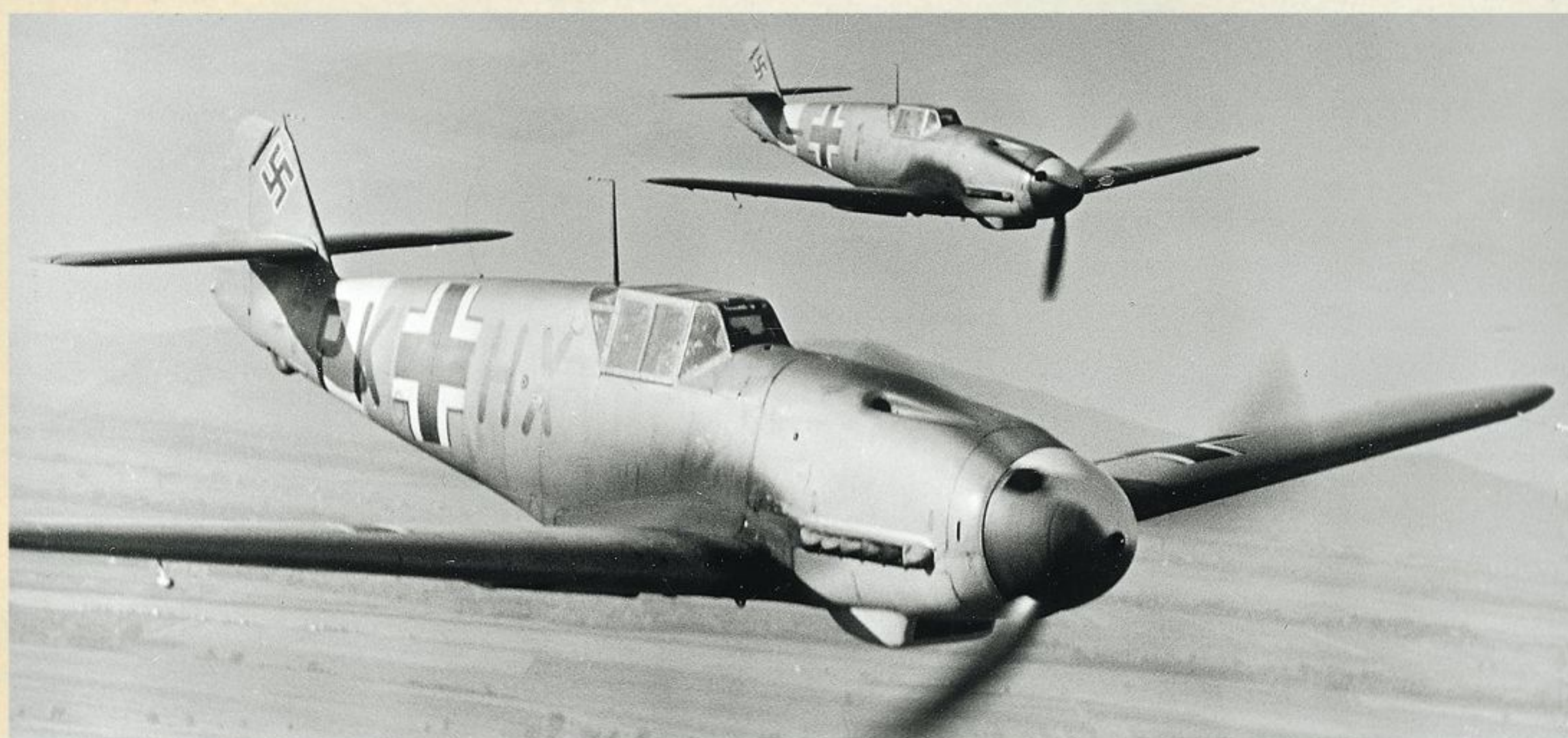
The Bf 109F was fitted with a more powerful DB601 engine in a new symmetrical cowl, and modifications were also made to the supercharger and radiator intakes. The 109F was also fitted with a new cantilevered tailplane, rounded wingtips, a smaller rudder and a fully retractable tailwheel (courtesy of Warren M. Bodie).
