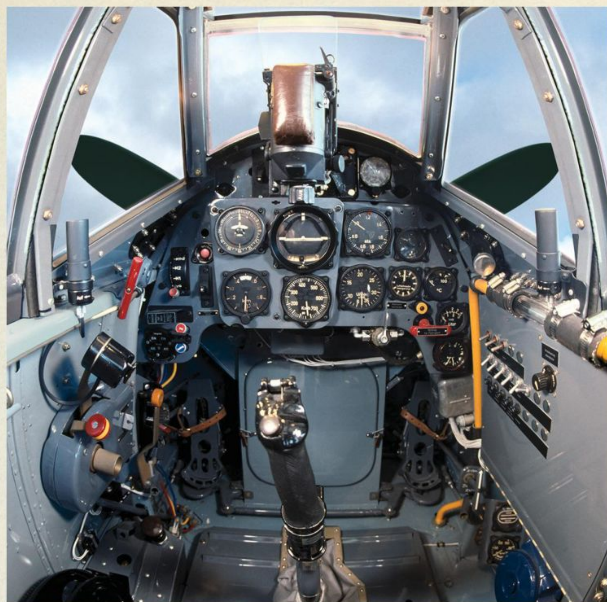
“Utilitarian” best describes the 109’s cockpit. As the heavily framed enclosure is lowered over your head, the feeling of claustrophobia is apparent. Power and flight controls within easy reach afford the pilot simplicity of form and function. The pilot’s legs straddle the MG 151 20mm cannon breech. photo by Brian Silcox)
