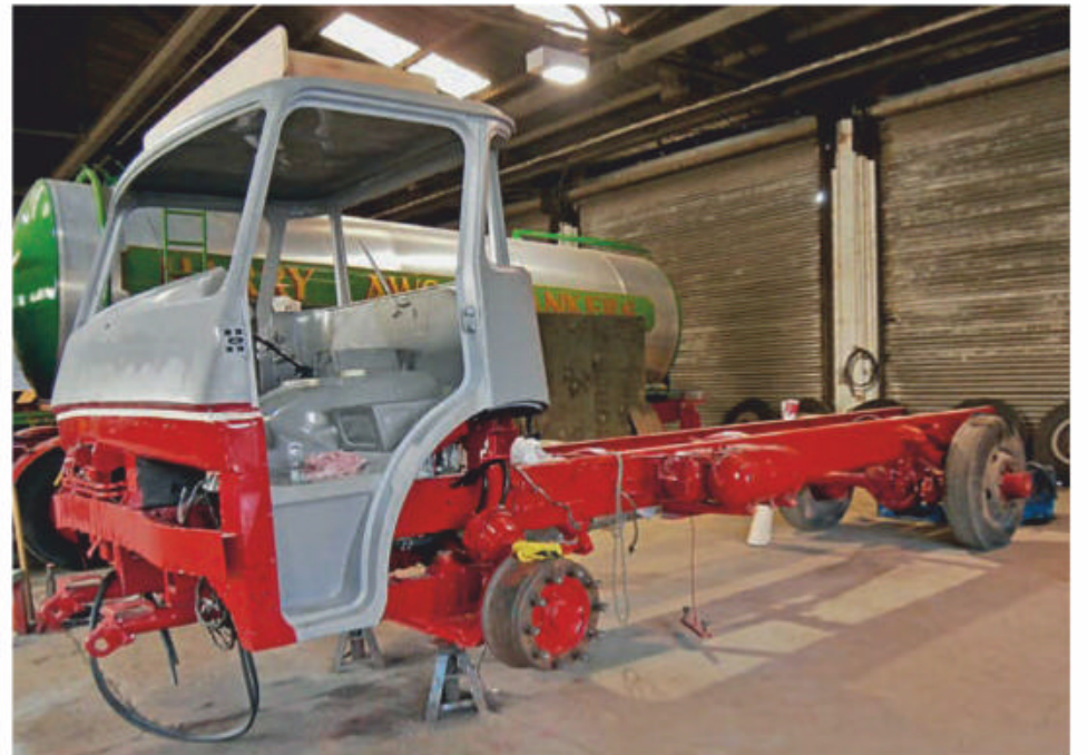
▲ The Motor Panels cab required attention to the rot in its floor pan and strange accident damage to both its front corners. Photo: Dave Watson Collection
