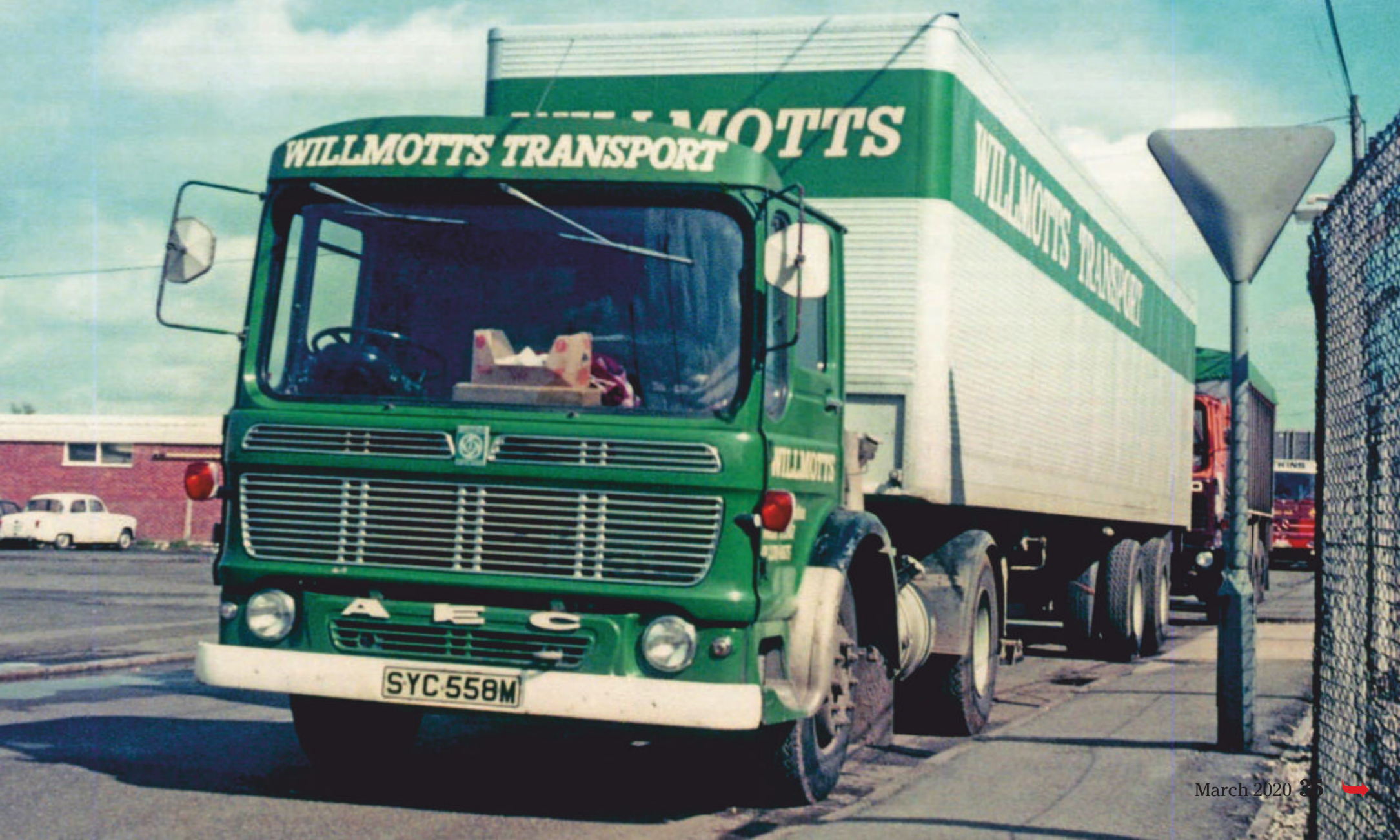
▼ Representative of the many AEC Mandator artics and Crane Fruehauf trailers, the standard outfit that Willmotts Transport operated in the 70s, is SYC 558M, seen parked at its home base in Princes Road. New in August 1973, she was powered by the lusty AV760 diesel and supplied by Arlingtons of Bristol.
