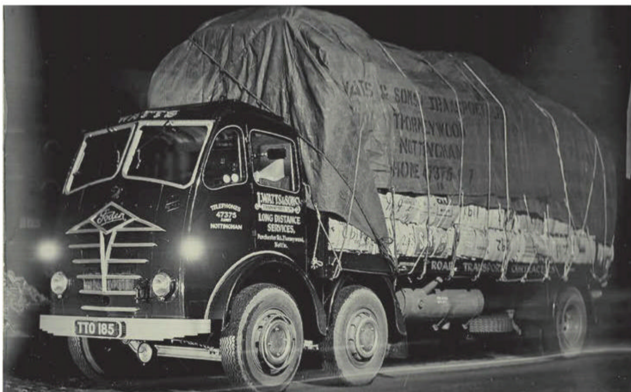
▲ It's believed that Foden were to fit an engine driven pump to their vehicles to assist in giving extra pressure to their hydraulic braking systems. Photo: Roger Kenney.
