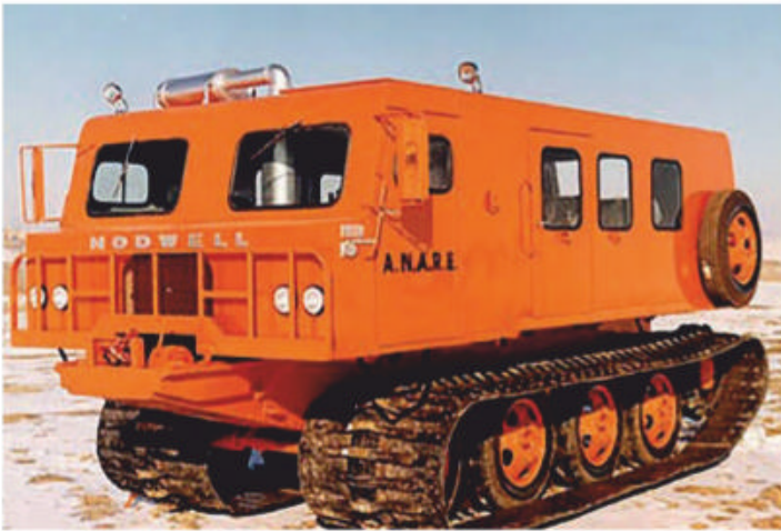
▲ The Nodwell 110 began life as a five-tonner in 1957. Over six decades on, Foremost's present evolution carries a 10-ton payload.
