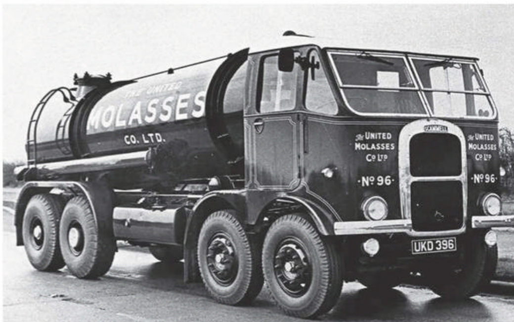
◀ When Scammell joined the rigid eight-wheeler field in the late 1930s they fitted air brakes as standard to their R8s.
