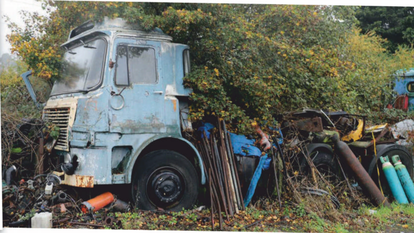
▲ An A-series ERF tractor unit with a converted 'pigeon loft' sleeper cab. These were a common sight in the mid-1970s as hauliers modified day cabs to have the most basic of bunks.
