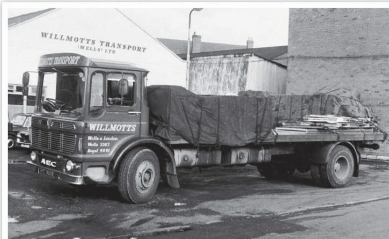
▲ HYC 960D, was an early example of the new tilt cab range offered by AEC using the Leyland Group 'Ergomatic' cab. New in July 1966 this Mercury and sister vehicle HYC 955D, were the last AEC rigids to join the Willmott fleet. Both were fitted with the AV505 diesel. Seen outside the Princes Road garage, note the twin diesel tanks.
