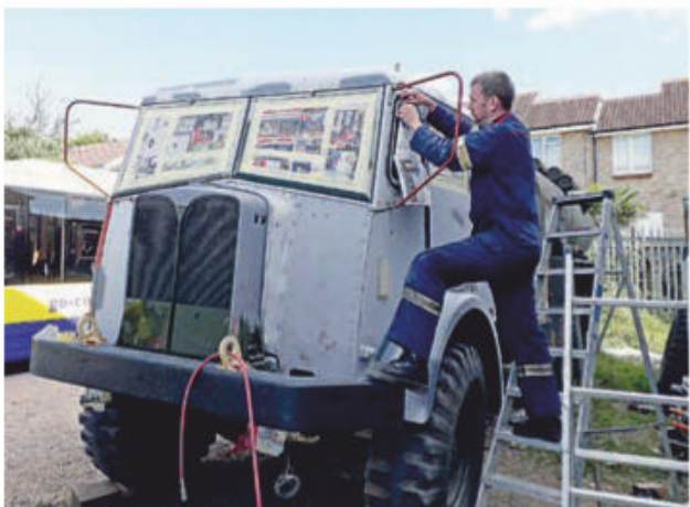
▲ Rob's son Stuart, a well-qualified Scania Truck technician by trade, starts the monumental task of masking up the Militant Tanker with last week's newspapers and a lot of tape.
