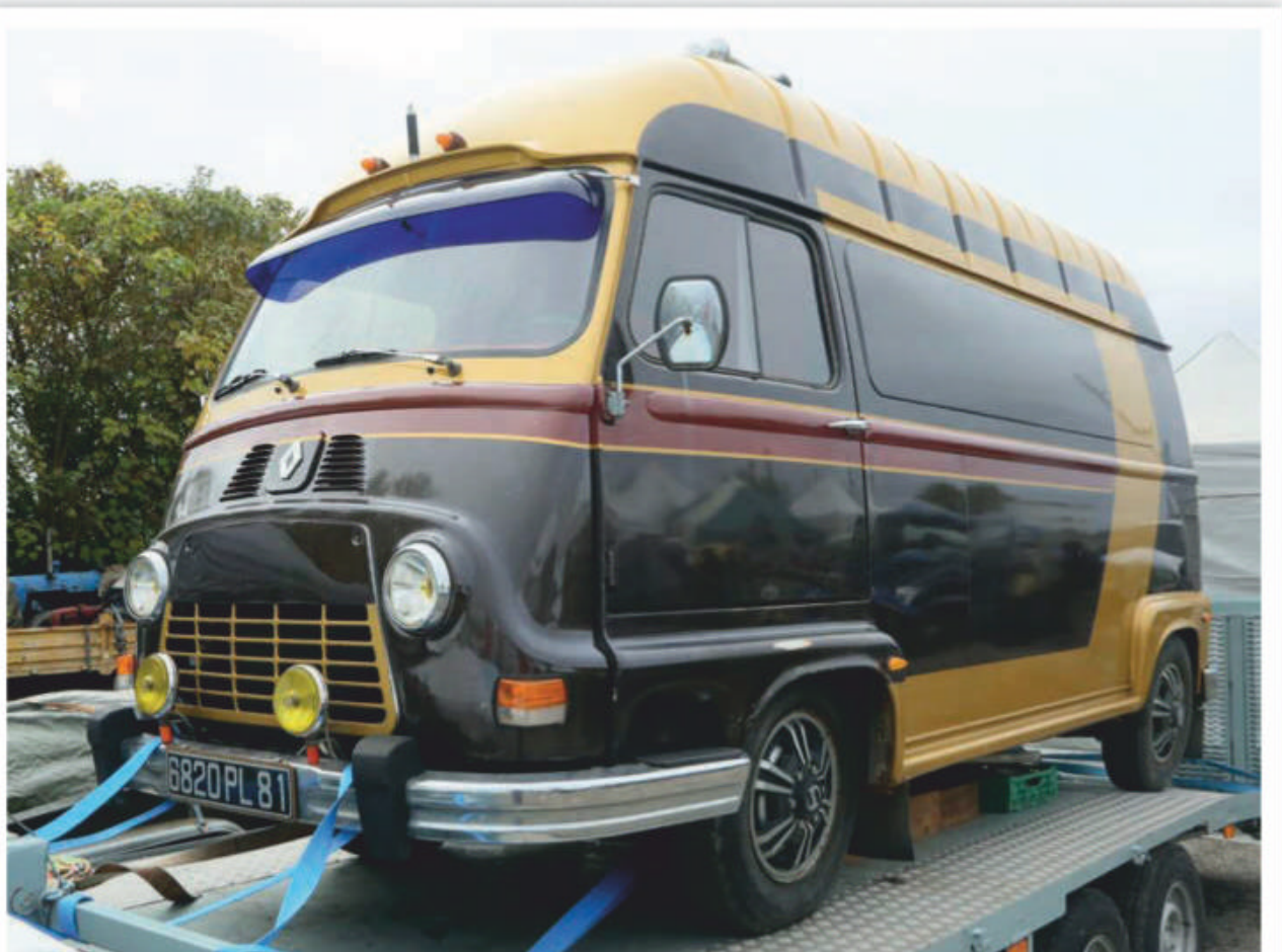
▲ Looking good the front-wheel drive Renault Estafette 12cwt panel van. It was to be the first Renault FWD vehicle. It came on the scene in 1959 as part of an initial six model range with the 845cc Dauphine petrol engine that later went to 1.3 litres with four-speed transmission and independent suspension all-round and was made successfully to 1980.
