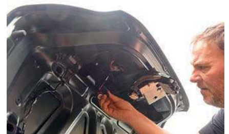
BELOW: Paul removes the four bolts that hold the plinth in place by using a 10mm socket
