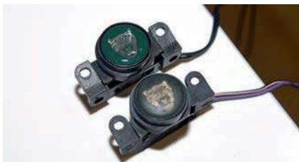
Adamesh's shiny new button release (top) with the faded, dirty original
