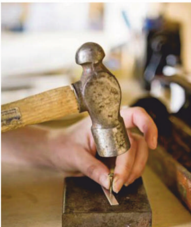
Tools used include tweezers for manipulating the components, pliers and a hammer to punch strips of metal to mark the position of the holes.
