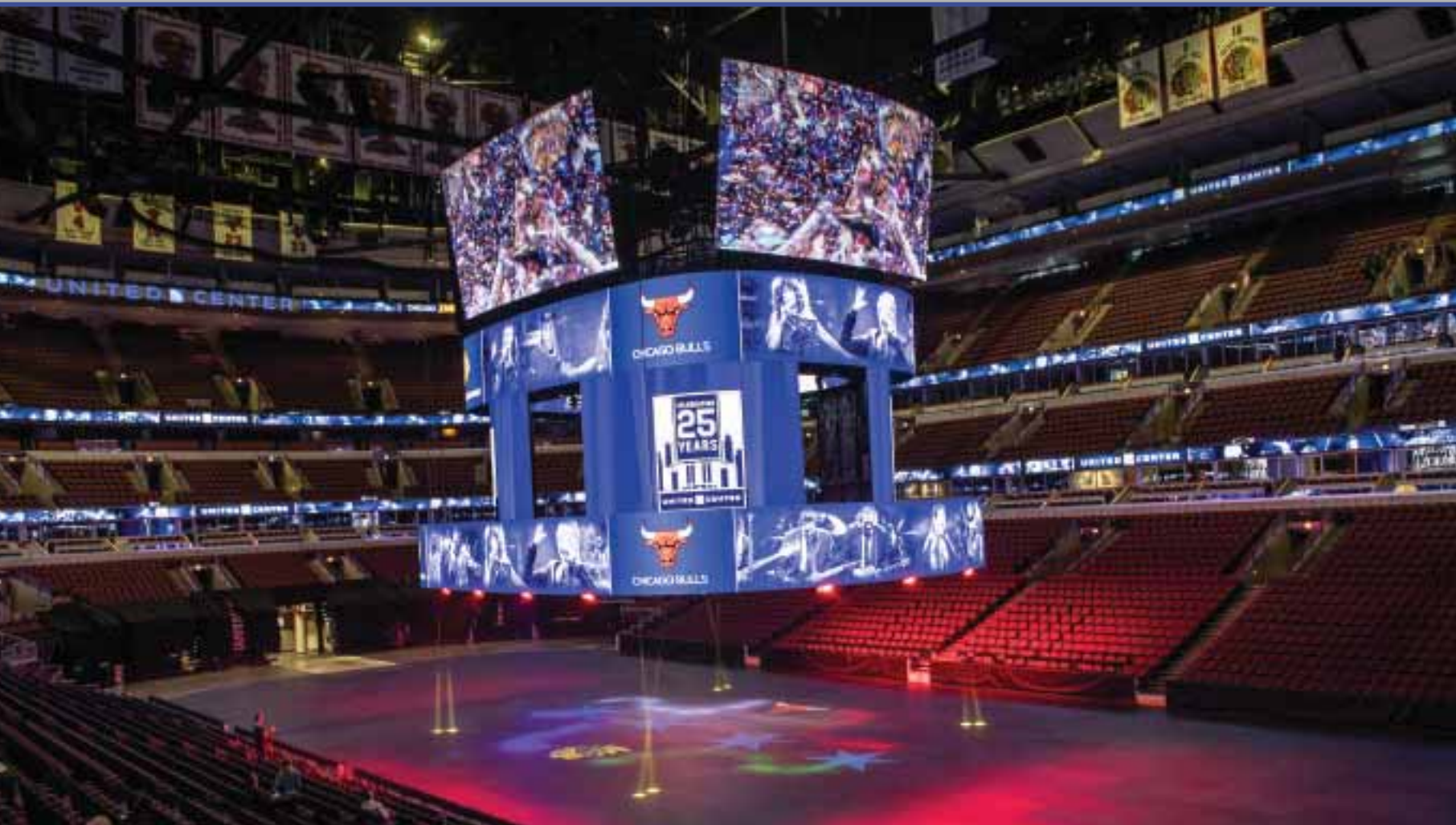
“The center-hung screen is composed of Mitsubishi XL-Series of ultra-lightweight, high-brightness SMD LEDs with true 4mm pitch,” notes video designer Barry Otto.
