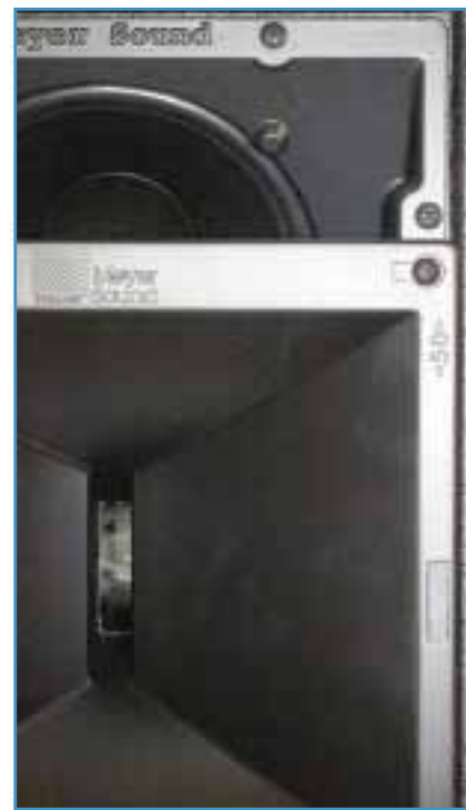
Horn orientation and indication for 50° vertical coverage.
