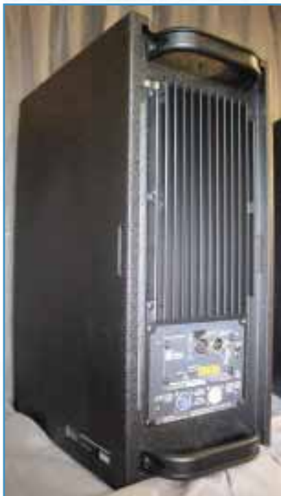
ULTRA-X40 rear. (Note handles at top and bottom and the water drainage slots back-mid of the cabinet, on either side of the amplifier.)
