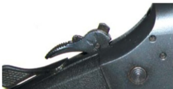
Close-up of the simple yet elegant hammer mounted barrel selector. Push forward for the rifle barrel and back for the shotgun barrel.
