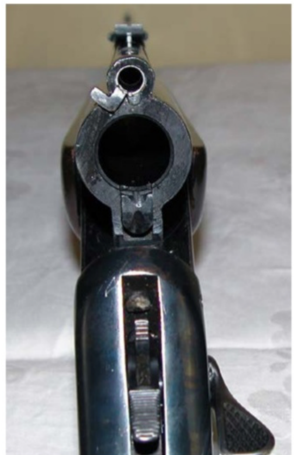
The separate extractors mounted on the earlier models. Note the rifle barrel extractor is a simple spring-driven affair.
