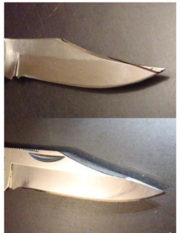
Marking the drop point; and the blade after grinding.
