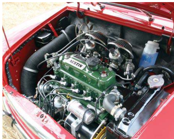
GP team Cooper carefully tuned Mini engine. Note modern aftermarket filters
