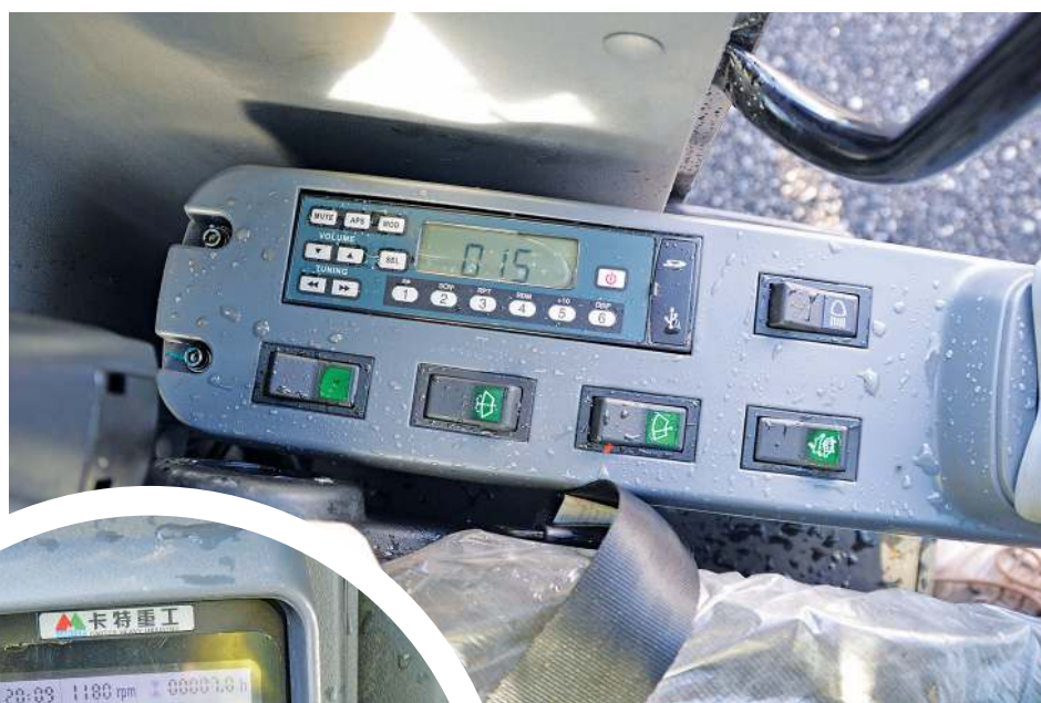
Left and above: The controls may be a little basic, but the speed and response to inputs are good, thanks to Japanese-inspired hydraulic systems.
