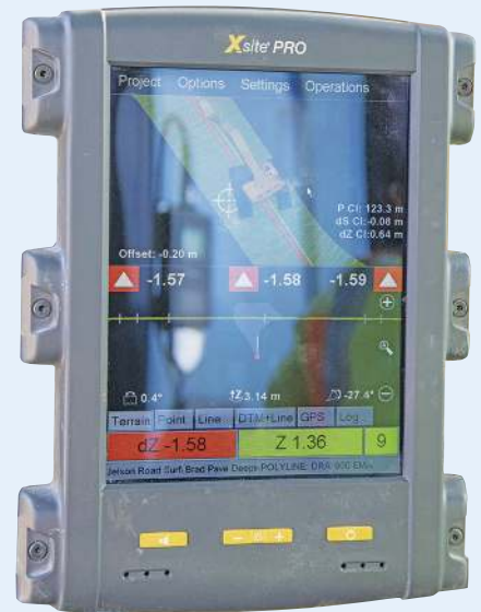
Above and below: Paul has equipped both front-line excavators with a Moba X-Site 3D machine guidance system, which he says is easy to use and cost-effective.
