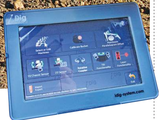
Above and below: The 2D iDig system is extremely powerful, providing the opportunity to work with dual grades and attachments such as tilting buckets and lasers.
