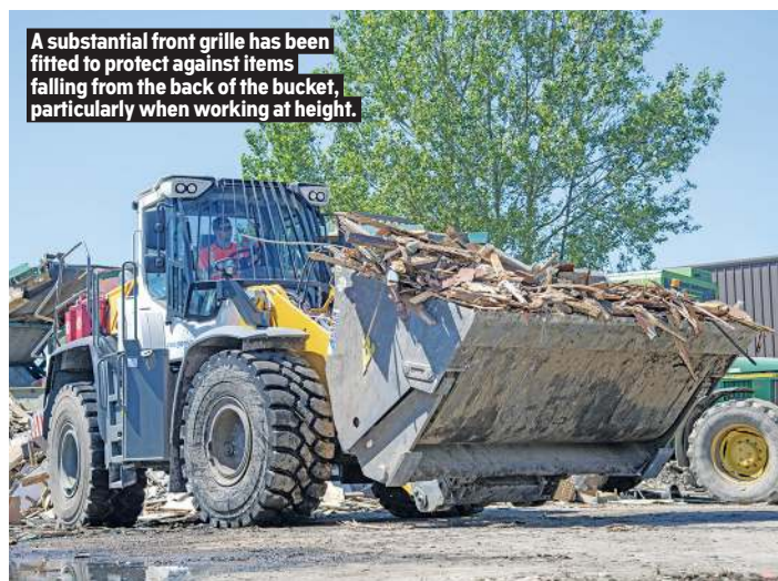
The loaders are expected to be capable of working with a variety of materials; the new Liebherr is usually tasked with household or green waste jobs.
