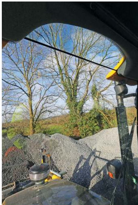
Below and inset: The sloping bonnet provides a decent view of the bucket on the ground, while the unique top glazing panel provides a great view when loading trucks.
