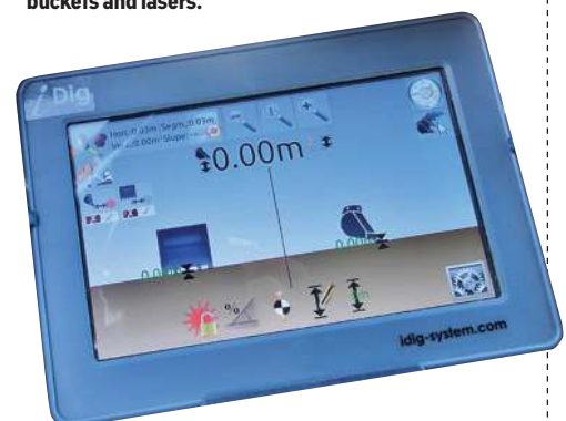
Above and below: The 2D iDig system is extremely powerful, providing the opportunity to work with dual grades and attachments such as tilting buckets and lasers.
