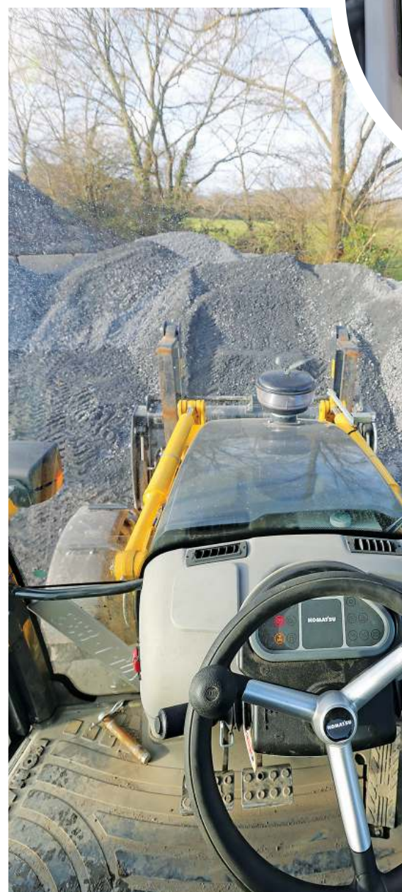
Below and inset: The sloping bonnet provides a decent view of the bucket on the ground, while the unique top glazing panel provides a great view when loading trucks.
