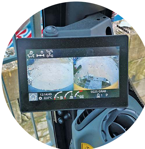
Below and right: Visibility is good, assisted by exceptionally clear camera feeds, and the hydraulically raising cab enables high-sided trucks and skips to be loaded with ease.
