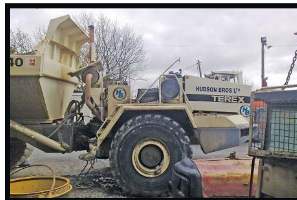
← An open-top version of a Terex ADT, at least on a temporary basis as the cab was removed to sort out a hydraulic issue.
