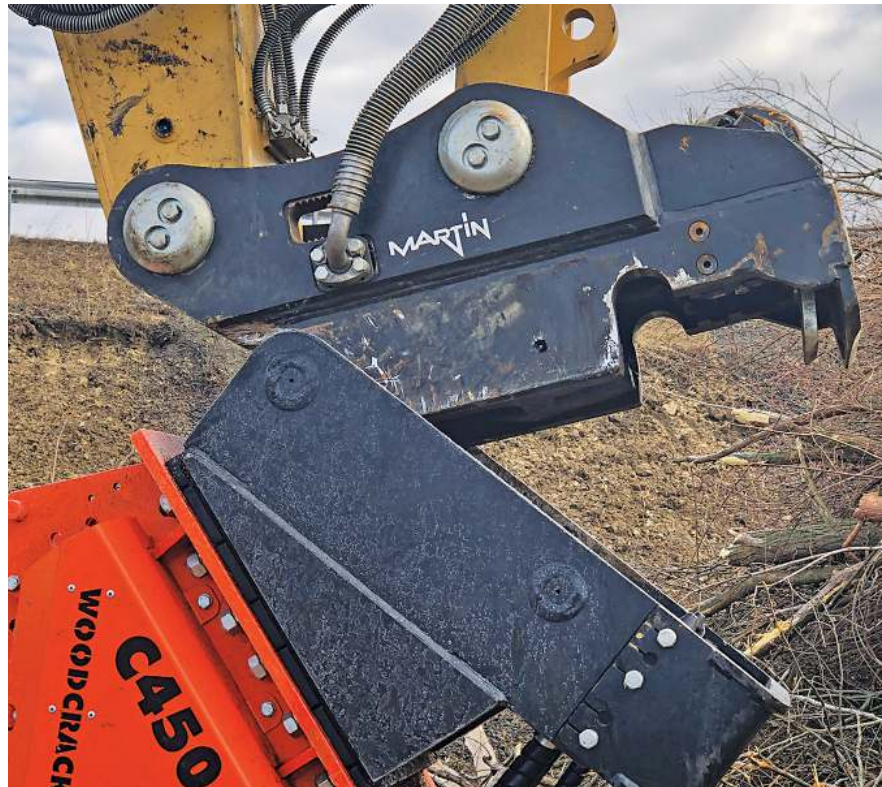
Above: Austria-based manufacturer Martin produces a range of heavy-duty automatic hitches, many supplied with auto hydraulic service line connections.
