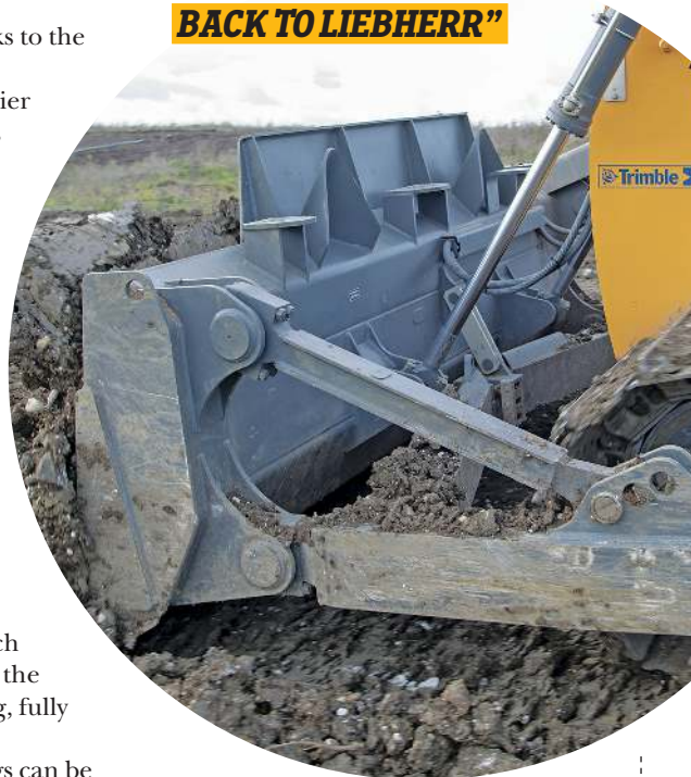
Above: The low ground pressure dozer has 914mm-wide double grouser pads and a 4.1-cubic-metre, outside mounted straight blade.
