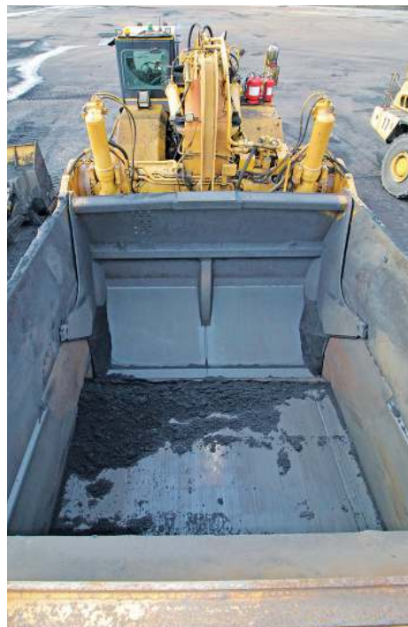
Above: Tyres last well on this site, and the cutting edge of the bowl only needs to be replaced every few weeks. The bowl itself has been armoured with additional Hardox steel.
