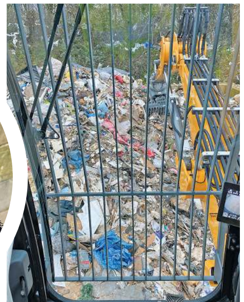
Below and right: Visibility is good, assisted by exceptionally clear camera feeds, and the hydraulically raising cab enables high-sided trucks and skips to be loaded with ease.
