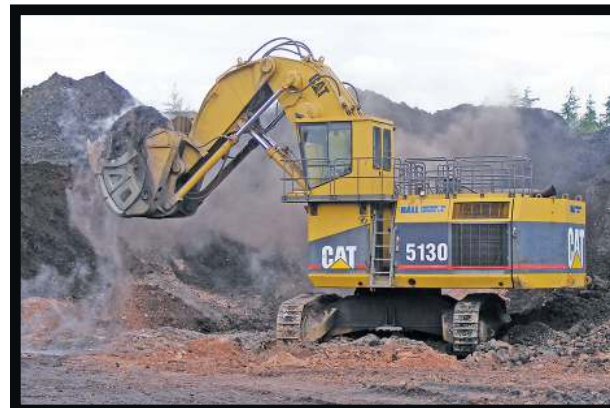
← A Cat 5130 with a hot load: digging out burning colliery material at the former Damside opencast coaling site.
