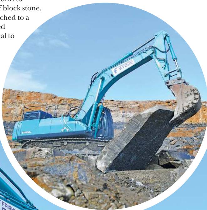
Below and inset: A bucket tooth is worked into a horizontal fracture, gradually widening it until the entire block can be extracted.
