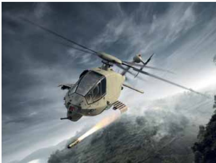
Rear-facing propulsor augments conventional main and tail rotors
