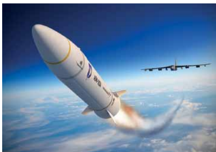
Boost-glide vehicle uses rocket motor for acceleration after release
