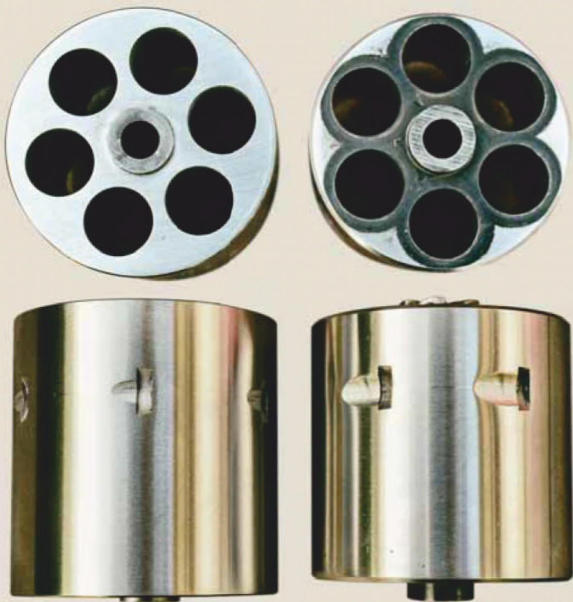
The centerpiece of these builds is the oversized six-shot cylinder, seen here next to a stock Ruger six-shot .45 Colt cylinder.
