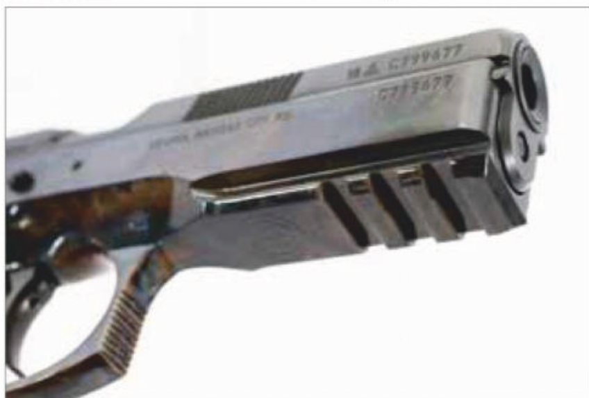
Left: To disassemble the GI CZ-75, unload and line up the two lines—one each on the slide and frame. Then, push the slide stop out.
