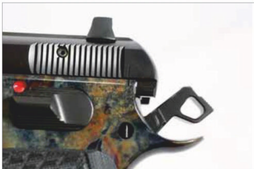
Left: To disassemble the GI CZ-75, unload and line up the two lines—one each on the slide and frame. Then, push the slide stop out.
