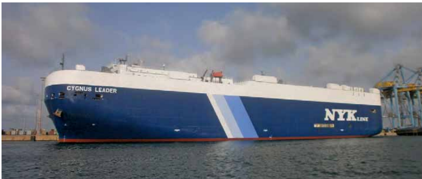
The 61,775gt vehicle carrier Cygnus Leader operates a regular service between the Far East and Europe with a capacity of up to 5,415 cars and 162 trucks
