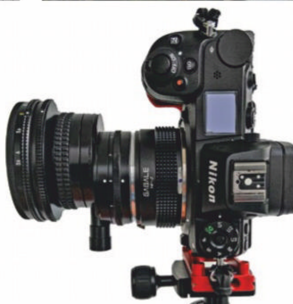
Picture 9: This is the setup that was used to capture Picture 8. The lens, a PC (Perspective Control) Nikkor 28 mm allows shifting (up to 12 mm) for correcting perspective errors. This picture shows the lens with rise movement employed.
