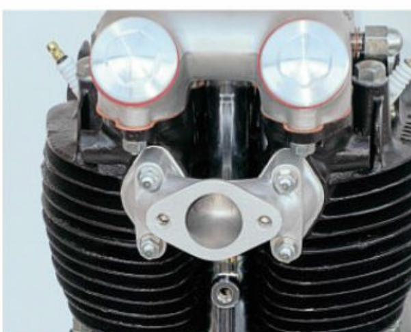
Two into one inlet manifold for the Triumph's single Amal 1 5/16 in 76/132 carburettor, manifold gaskets, studs and nuts. Two of the nuts pictured are slave nuts with which to fit the manifold studs. The carburettor studs will be fitted to the manifold when the carburettor is returned to the engine after its renovation.
