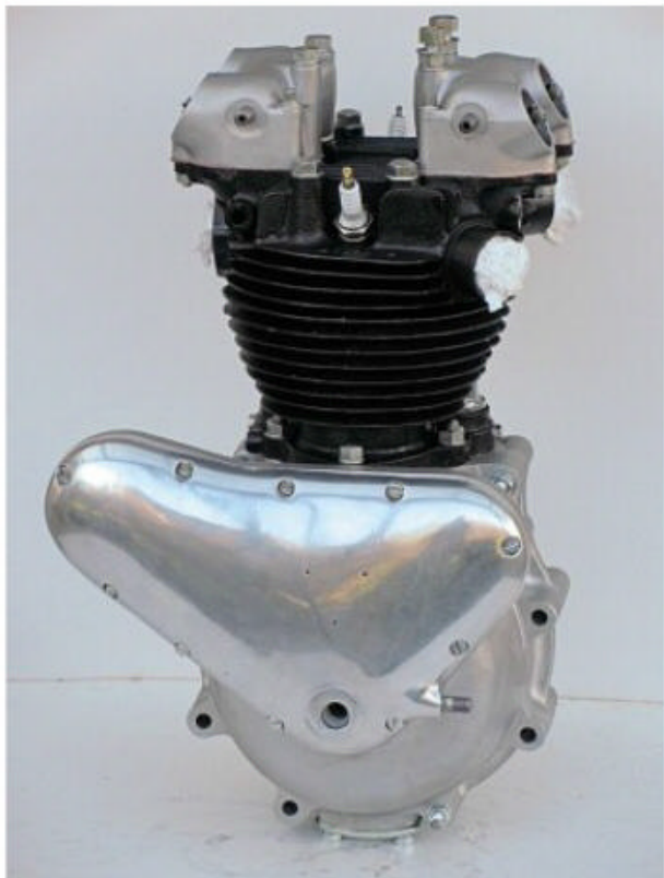
Front and rear rocker boxes fitted and all seals in place. Breather valve and timing chest cover badge to be fitted later.
