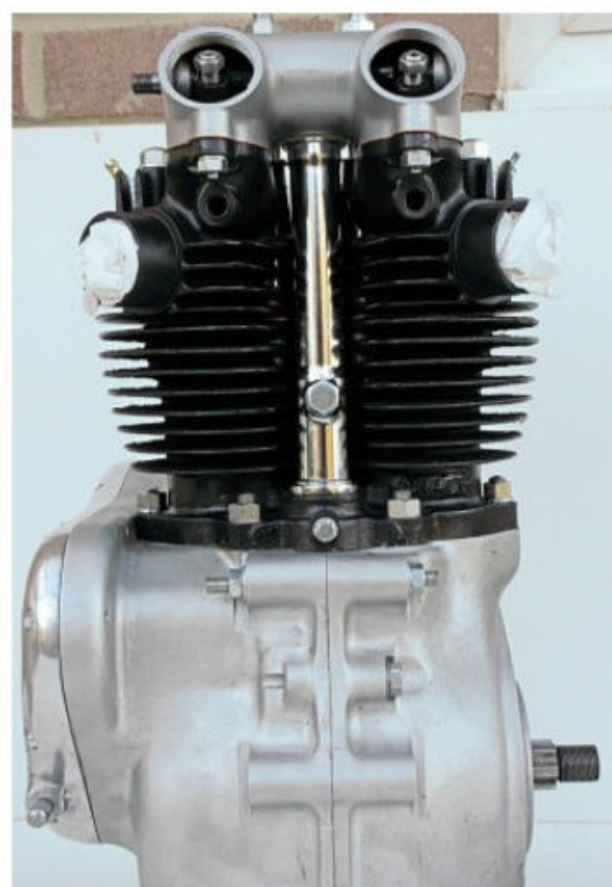
Some eye of faith is needed here. The first photograph illustrates the pushrod tube's rotation to the left as one looks at the engine, while it has been squared before the second picture and final tighten. You will note no mention of fastener torque settings has been quoted here. Two reasons – firstly (and perhaps arrogantly on my part) I rely on tightening by experience for older all iron engines, but always tighten to recommended torque for later units with aluminium cylinder heads and/or barrels if torque settings are quoted, and, secondly, this engine is a total rebuild with all new gaskets, soft annealed cylinder head etc and it will settle and need further appropriate tightening before starting, during running in and on completion of running in. ▶
