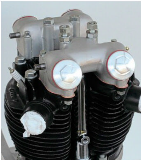
Tappet adjustment caps and sealing fibre washer. Some rebuilders prefer thin 'O' ring seals. The choice is yours, but on removing caps it's often a sound idea to replace the seals, as they seat and often you won't return the fit to the seat.
