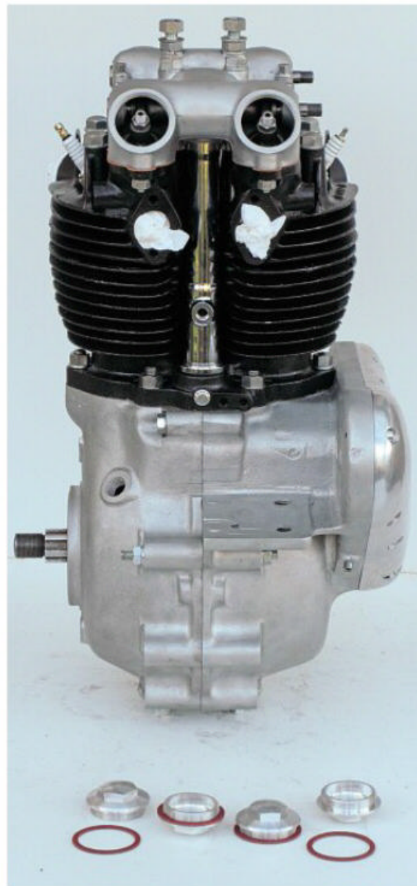
Tappet adjustment caps and sealing fibre washer. Some rebuilders prefer thin 'O' ring seals. The choice is yours, but on removing caps it's often a sound idea to replace the seals, as they seat and often you won't return the fit to the seat.
