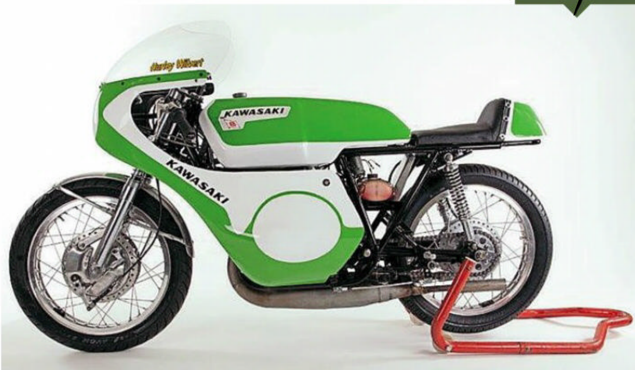
Brought back from NZ in 2009, in October 2012 full restoration of this 1966 Kawasaki A1R started. The machine appeared to be all there but on closer inspection the engine had no internals; bits were sourced in the US and Fahren Engineering made up new cylinder liners and reworked the cylinder heads. To be sold at the Classic TT auction.
