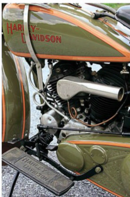
The rocking heel and toe clutch lever. The clutch can be set with a touch of slip, making riding in traffic easy.
