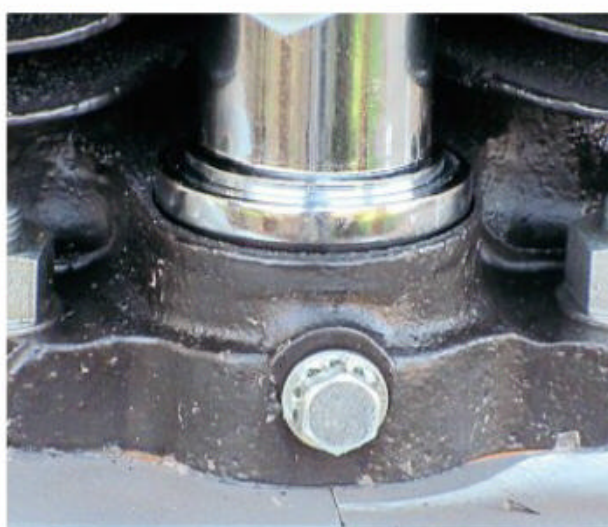
Bottom pushrod seals nicely compressed in situ for a sound fit without any of the seal squeezing out. If this happens – and it's apparently often the top one which causes problems – it's a case of try, try again.
