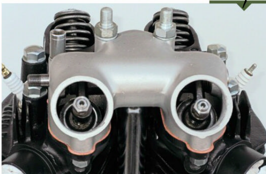
Front rocker box fastened. The two front rocker cover through fasteners also accept the head steady once the engine is installed in the frame. Oddly, the parts list we have show these as one per rocker cover, which doesn't seem correct, but as the rebuilt engine will be fitted to the rolling chassis as part of the final dry build procedure, we can remedy this if we are wrong.
