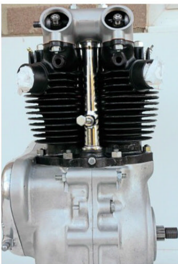
Some eye of faith is needed here. The first photograph illustrates the pushrod tube's rotation to the left as one looks at the engine, while it has been squared before the second picture and final tighten. You will note no mention of fastener torque settings has been quoted here. Two reasons – firstly (and perhaps arrogantly on my part) I rely on tightening by experience for older all iron engines, but always tighten to recommended torque for later units with aluminium cylinder heads and/or barrels if torque settings are quoted, and, secondly, this engine is a total rebuild with all new gaskets, soft annealed cylinder head etc and it will settle and need further appropriate tightening before starting, during running in and on completion of running in. ▶
