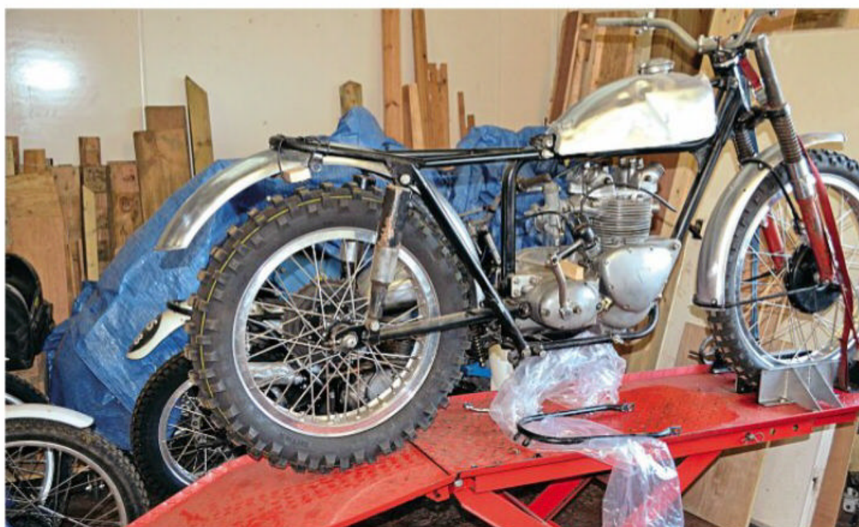
The new alloy guard is wired in place.
