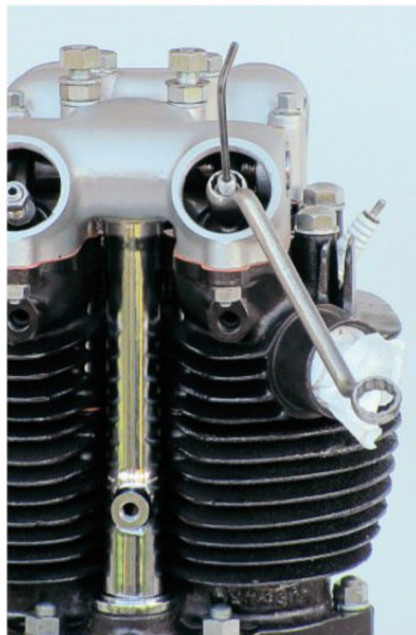
Valve clearance adjustment. With piston on compression stroke, both valve clearances for that cylinder are set. The Triumph instruction book states: "The adjustment is made when the engine is cold and it is advisable to ensure there is the slightest up and down shake on the rocker arm, which will give the approximate clearance of 0.001in." These replacement tappet adjustment screws have Allen key heads, not to everyone's taste, but I like them.
