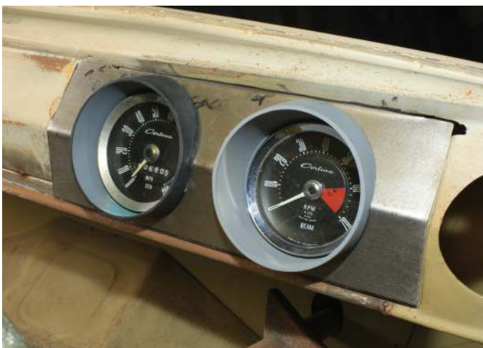
...and close up, demonstrates, I've swapped that cluster instrument for a GT rev counter; complete with matching Cortina script – the guts have been ripped out and an electronic unit's been slotted in place to cope with my V8!
