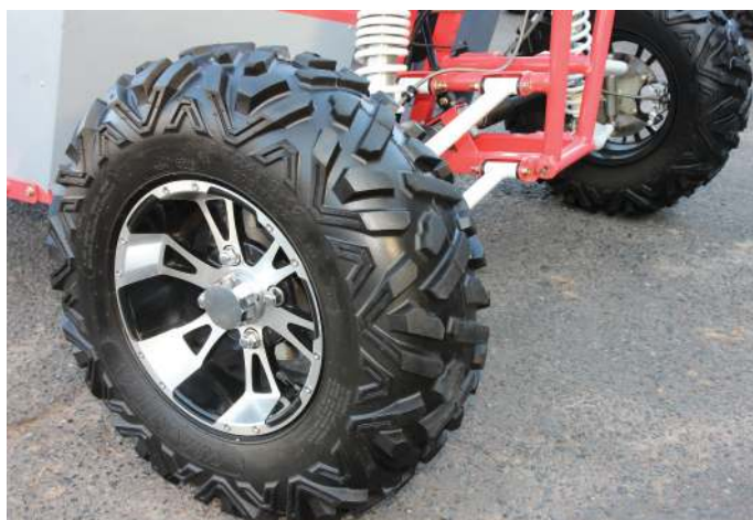
All-terrain balloon-tyres help to soak up the lumps and bumps, along with the suspension
