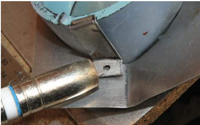
Allowing it to be plug-welded to the back face – might be wise to remove the plastic pod for this to prevent heat damage!
