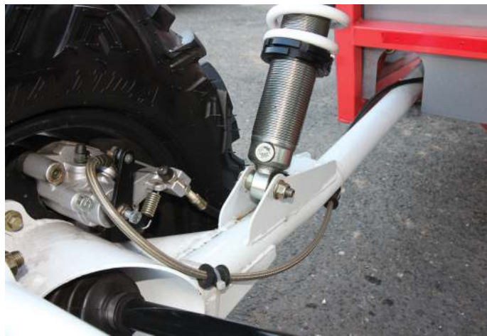
Long rear trailing arms help to provide plenty of suspension travel, essential for driving off-road
