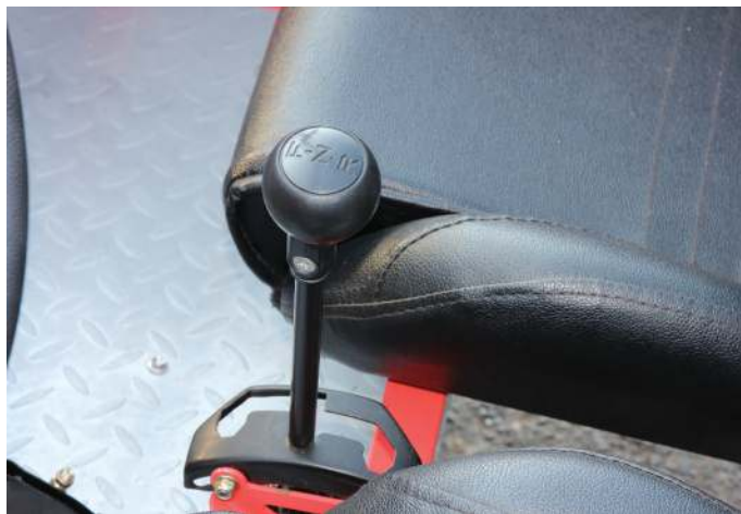
Gearstick controls a CVT gearbox with forward and reverse
