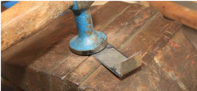
...you can use this to form fairly wide sections but you do risk hammer marks so a clean vice and hammer face plus care is needed. In truth, we should have left the strap longer, then trimmed it to length!
