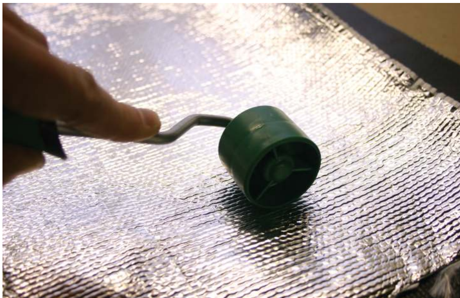
Self-adhesive heat cloth can be quickly applied to protect glassfibre panels from heat sources. The roller helping to eliminate any pockets of air
