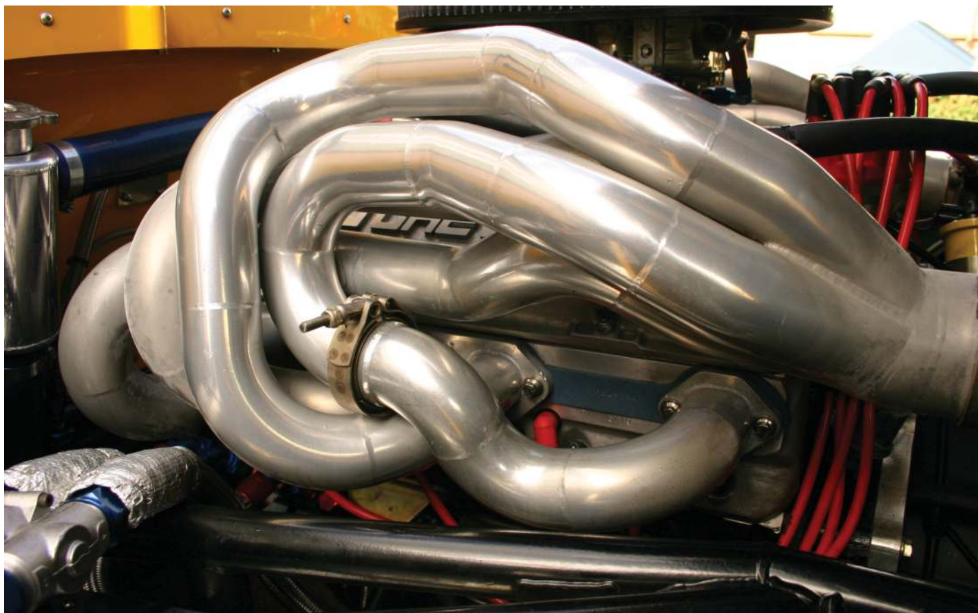
Ceramic-coated headers; another way of keeping your engine bay cool
