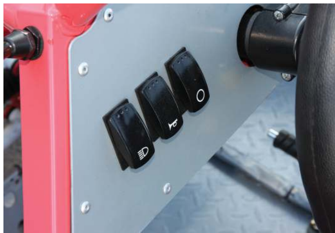
Simple switches. These three are for full beam, the horn and starter motor
