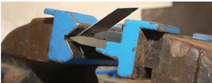
We slotted our strap into the brake and folded the steel along the required line...
