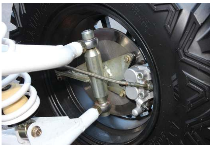
Traditional kingpin design for the upright helps to keep components straightforward to maintain. Braking employs discs all round
