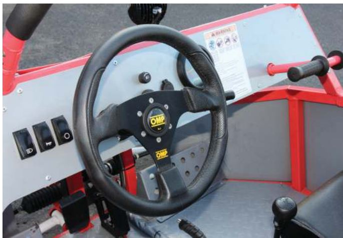
Left-hand-drive steering can be switched to the right
