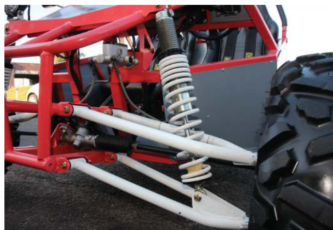
Front suspension adopts a well-proven design with double upper and lower wishbones and an outboard-mounted adjustable coilover from Gaz
