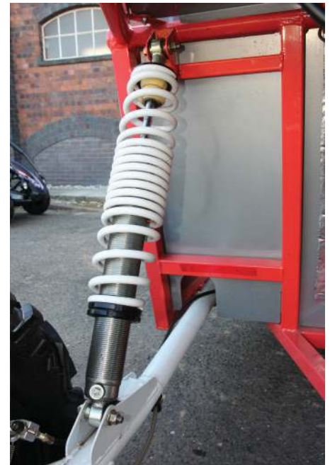
Remember the GTM Libra and its long rear-mounted coilovers angled at 45 degrees between the body and rear hubs? The DX10 has a similar design
