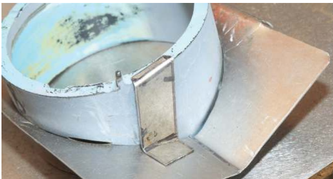
This is our strap, which should hold the plastic pod in place; which I'll replicate on each pod, to give three-to four points of contact. Not sure how I'll fix the back edge in just yet – maybe bond it or physically fix it with mechanical fixings – that's to be determined....
