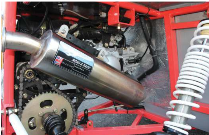
Sophisticated UK-manufactured exhaust system contains lots of packing to help keep the noise levels down and prevent your ears from ringing
