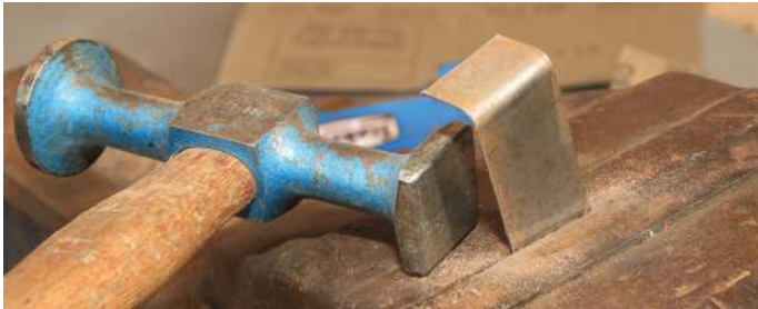
....although we need a much smaller fold at the top; and angled at that. OK, we made a cock up – but it highlights another method - most of these bending machines are not good at very small folds so, what you can do is use the good old vice and a body hammer method; to tap the fold over...
