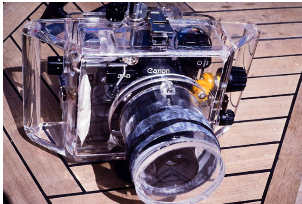
The housing for the Canon F1n and Speedfinder, here with a macro lens
