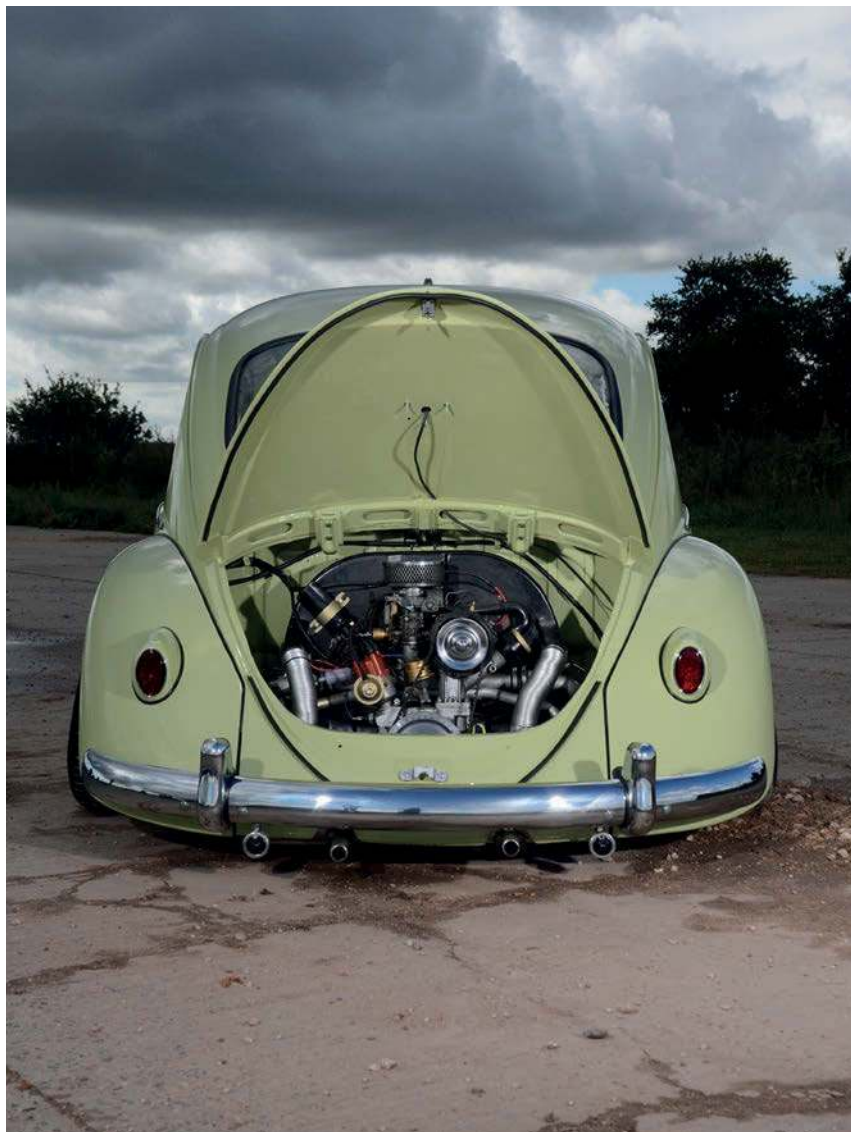
✓ Original 1300's been replaced by a rebuilt twin-port 1600
