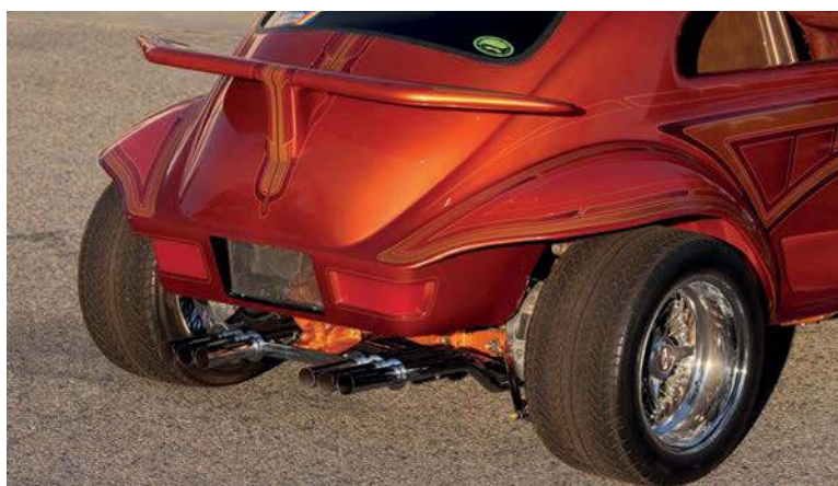
▲ Welded to the 'shell, the engine cover merges with the sloping contour of the custom rear wings
