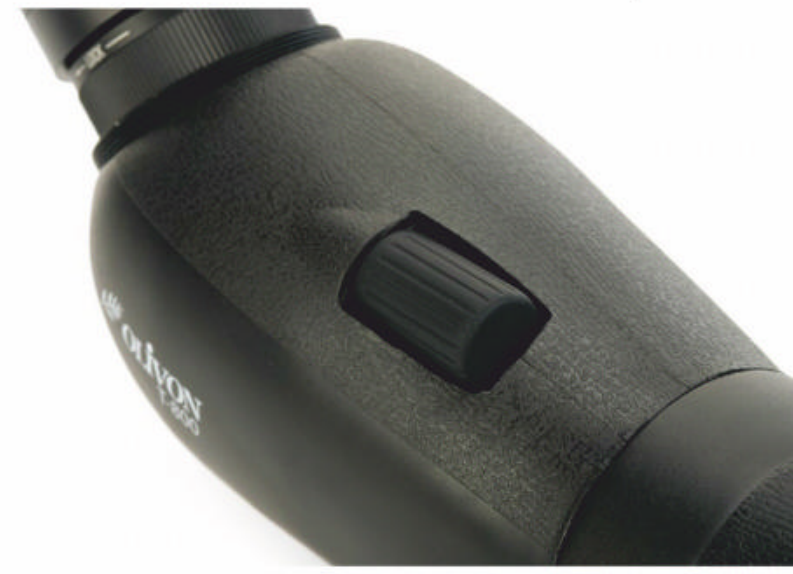
Above: The Olivon T800's 1.25" eyepiece holder accepts astronomical eyepieces, making it ideal for observing bright night-sky targets
