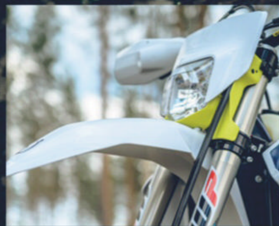
Brake hose now runs behind headlight shroud
