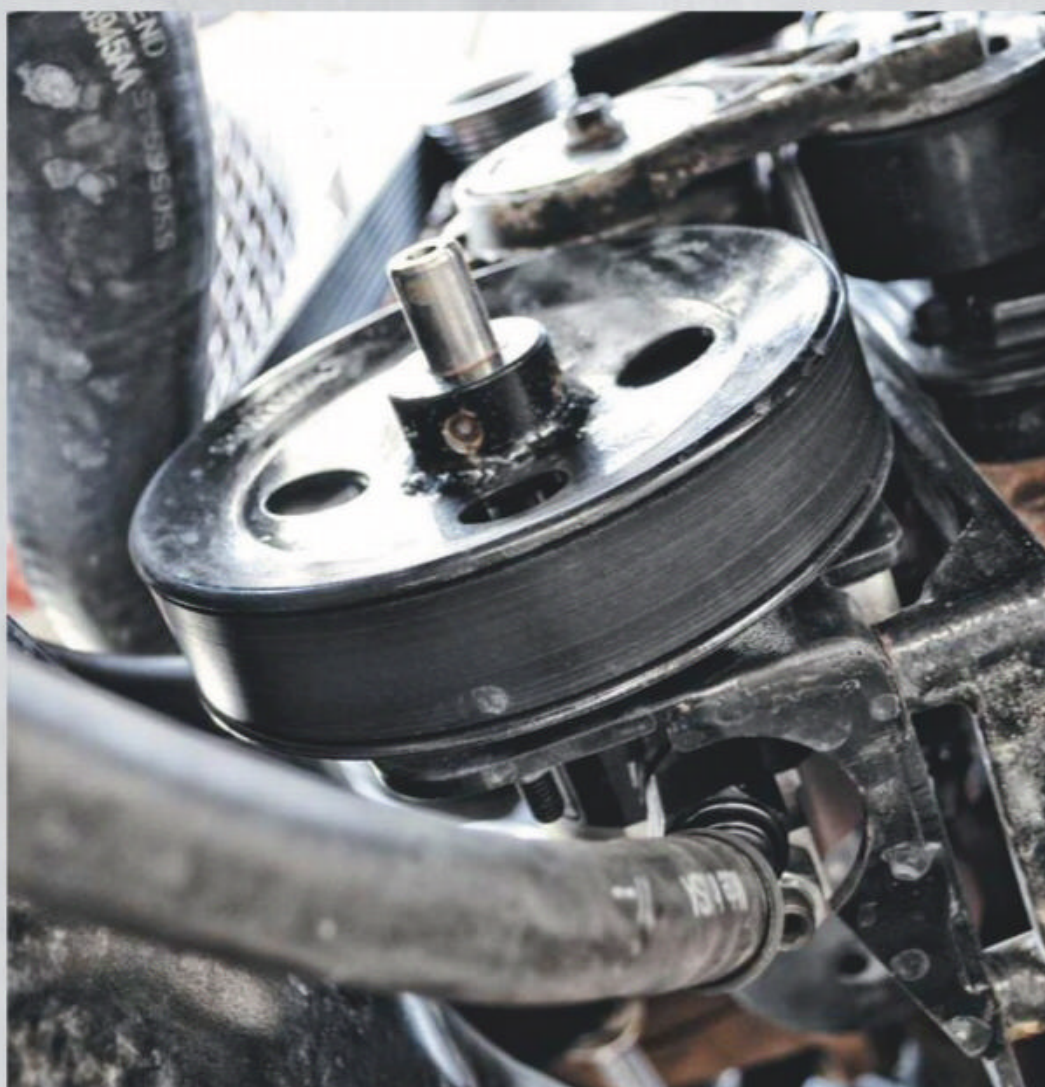
▲ One area where Mitch departed from the norm was the lift pump. Instead of running a traditional electric pump, Mitch runs a belt driven Aviaid pump that he uses as a lift pump. The system is set up at 17 psi, and has worked flawlessly so far.
