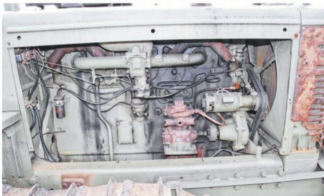
▲ The IH 691ci 6-cylinder diesel debuted about the same time as the TD-18. It was a part of International's second generation family of diesels and they pushed them in a big way. It had a 461ci, 68 brake horsepower, four-cylinder little brother with the same bore and stroke that was used in the TD-14 crawler and other applications. The 691 saw use in a great many applications beside the crawler, including marine and stationary operation. It was a wet-sleeved, indirect injected, seven-main bearing six and weighed in at 2805 pounds. At 1400 rpm, it made 103 hp. It was rated at 84.66 belt horsepower by IH and 80.44 at Nebraska in a 1938 test but in civilian use, they only ran them to 1200 rpm. The engine was revised several times in its long life, to about 1958, and was listed at 125 hp at 1600 in 1958. Like all the period IH diesels, it started on gasoline and then was switched over. It had a direct driven air compressor used for an air brake system for trailed equipment.
