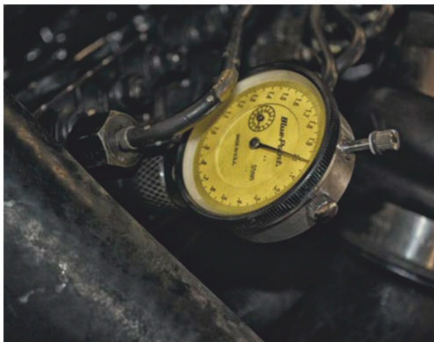
▲ Back up on the top of the pump, we put the dial indicator at a high number and rotated the engine backwards until the pointer stopped dropping. This meant the dial indicator is at the back of the pump cam lobe. From there, we zeroed out the dial indicator at 0.0 to find timing via plunger lift.
