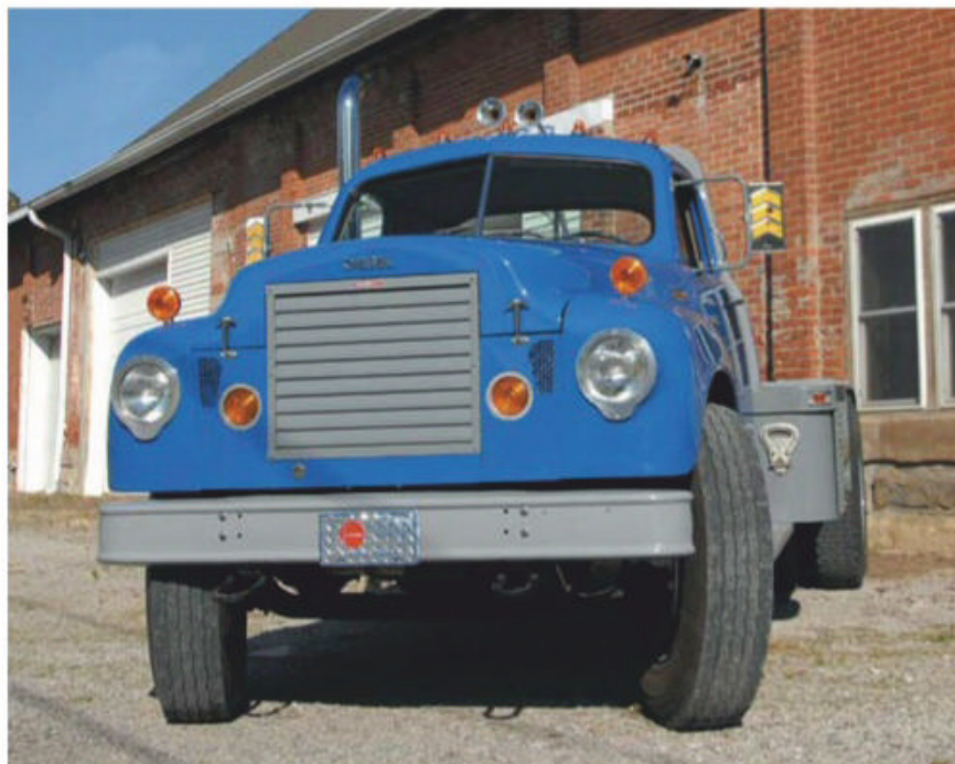
▲ The 96BBC truck, the “BBC” for “Bumper-to-Back-of-Cab,” was a revision to the standard Studebaker front end that lopped 10.5 inches from the length of the truck. After studying available documents, Marv estimates under 50 were built. All the diesel trucks had the thermostatically controlled Kysor shutters, though on the standard Transtar they were behind the grille. This prevented overcooling under light loads or cold weather
