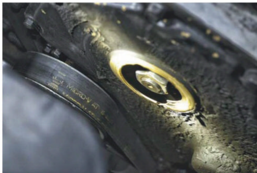
▲ After we found TDC, the oil filler was taken off, which gave us access to the large timing pump gear nut.
