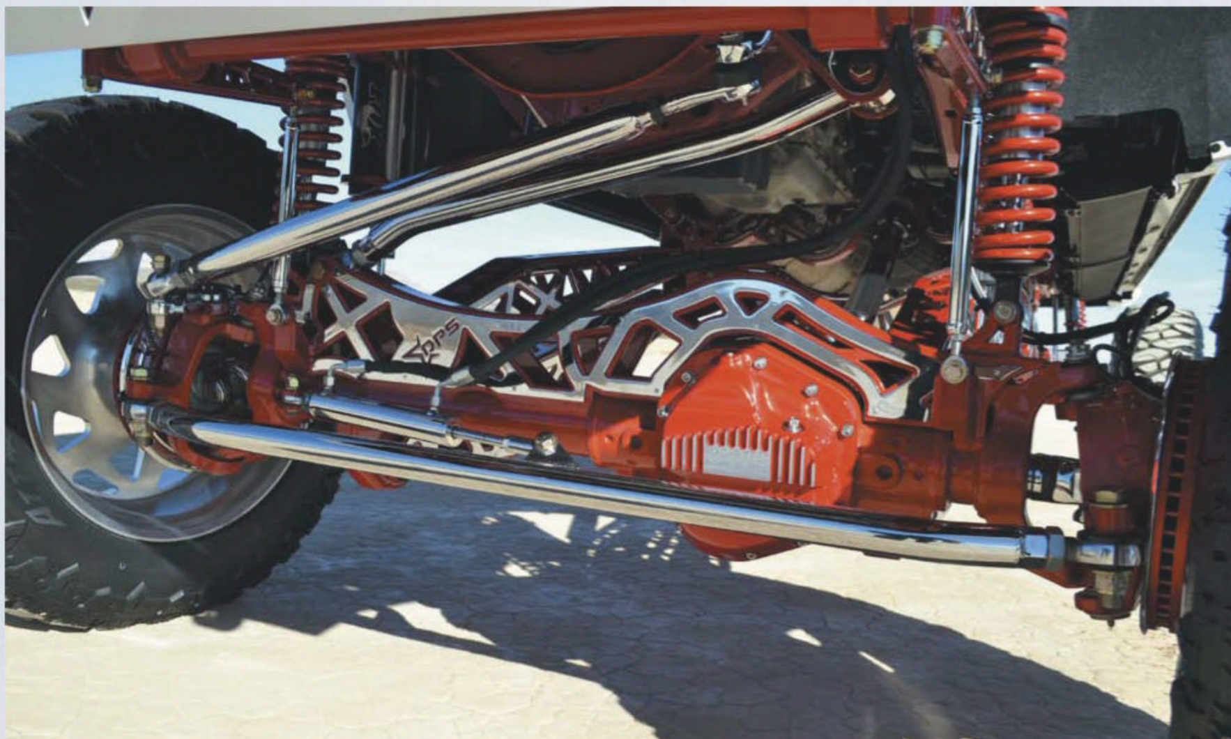
▲There's a lot going on in the front of the Excursion. The Dana 60 has been fitted with 4.88 gears and a Mag-Hytec differential cover. The truck also features a custom hydraulically assisted steering setup, because the length of the truck involves a lot of lock-to-lock steering.
