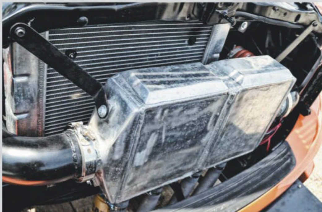
▲ Twin Frozenboost intercooler cores were welded together to make one single large unit. The pumps to circulate the water (as well as the fuel tank) are located in the weight box.
