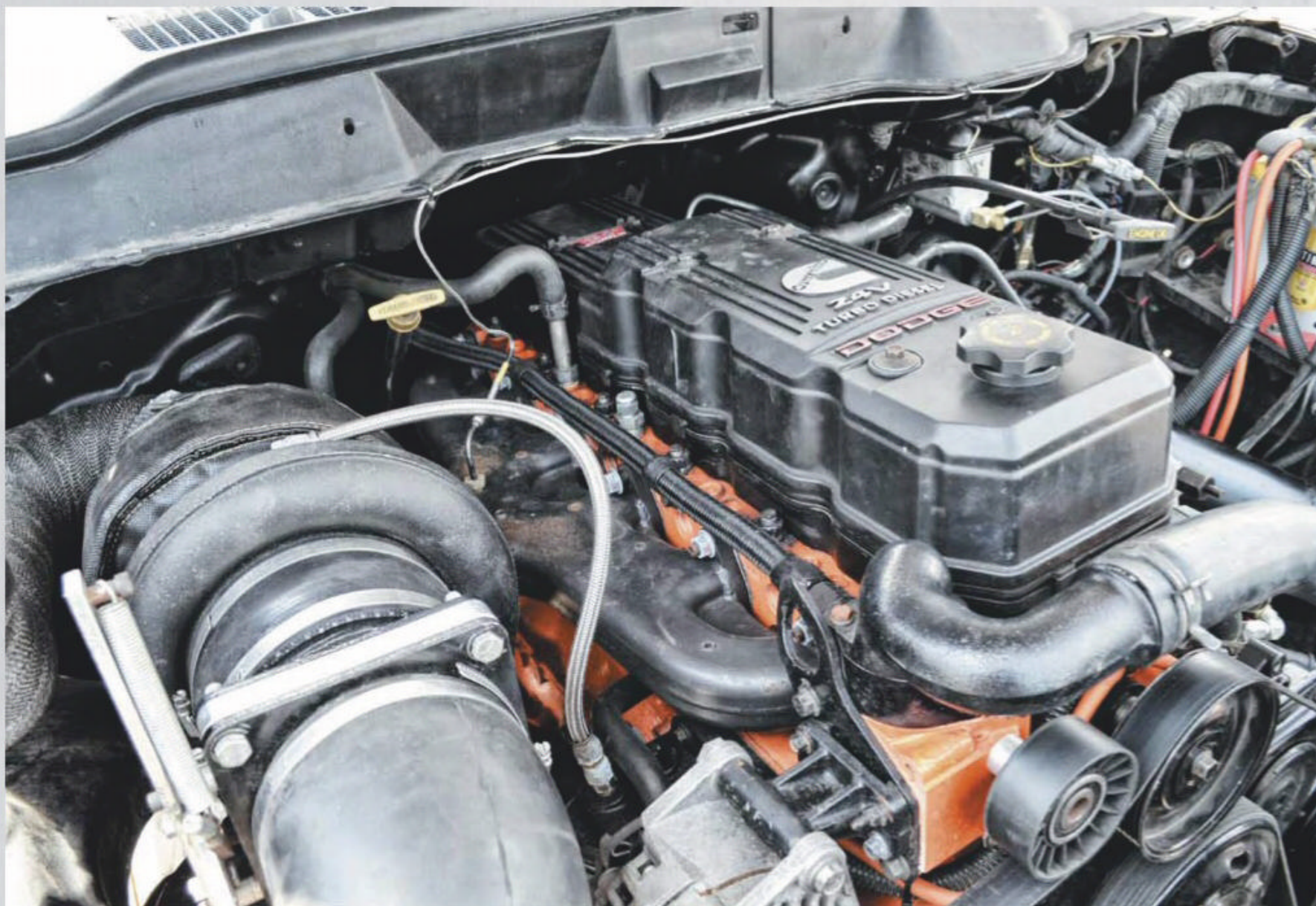
▲ Mitch Meinhart took great pains to ensure that his 5.9L would perform extremely well, and also look the part. Although it's never been on a dyno, Mitch estimates horsepower at about 1,200 hp.
