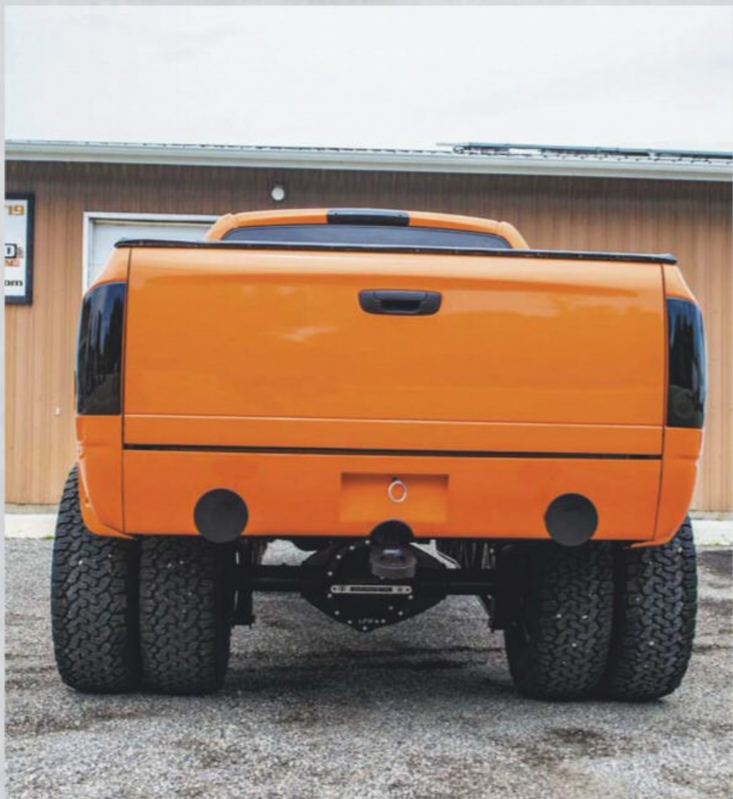
▲ Mitch put a lot of time and money into strengthening and modifying the rear axle of the truck, from the reinforced differential cover, to the 38 spline axles, to the pinion brake which you can see peeking out on the bottom right corner.
