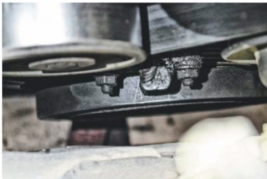
▲ We marked TDC on the balancer on either side of the crank sensor with a screwdriver for future reference, and to see how much the damper would turn when our pump was re-timed.
