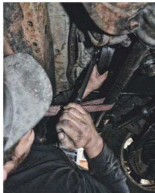
▲ When we got close to TDC, we took the valve cover off the number 6 cylinder and had one mechanic go under the truck and turn the engine slowly by the flywheel teeth until the rockers crossed over. This meant cylinder number one would be on the top of the compression stroke. Other popular methods of finding tdc are pushing on the timing pin right below the injection pump, or using a dial indicator set to the piston on the number 1 injector hole.
