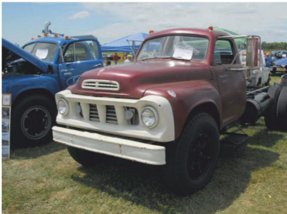
▲ A standard Transtar diesel, like Rick Meadows’ ‘62 shown here, looked more like the standard Studebaker truck of the given year. You can see the Kysor shutters behind the grill. This truck was also sold as a tractor.
