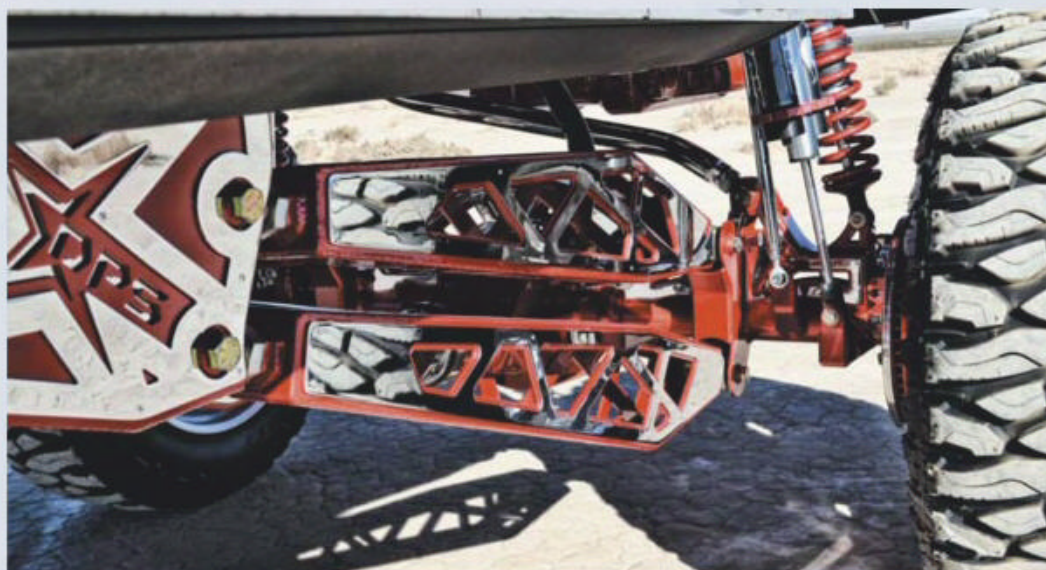
▲A stock Excursion uses leaf springs on the rear, but that wasn't an option at the lift levels that DPS wanted. Again the company turned to Fox Racing, and they built a rear suspension setup that matched the front, along with the huge Fox coil-over shocks.
