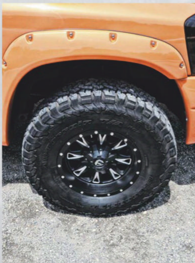
▲ Under the bright orange paint up front are 35x12.50 BFGoodrich All-Terrain tires, which are mounted on 17x9-inch Fuel Throttle wheels.
