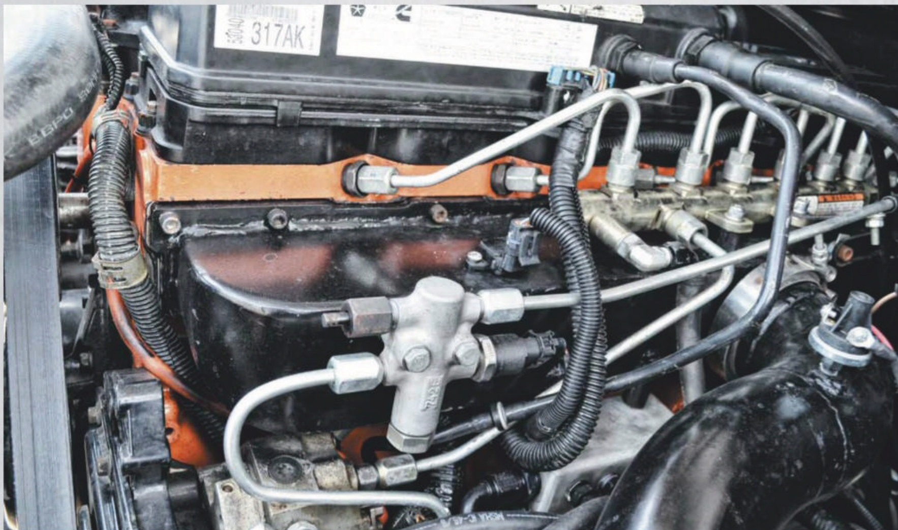
▲ From the camshaft on up, Mitch did all he could to improve airflow throughout the engine. One of the most time-consuming but worthwhile steps was building the side-draft intake for the 5.9L engine.
