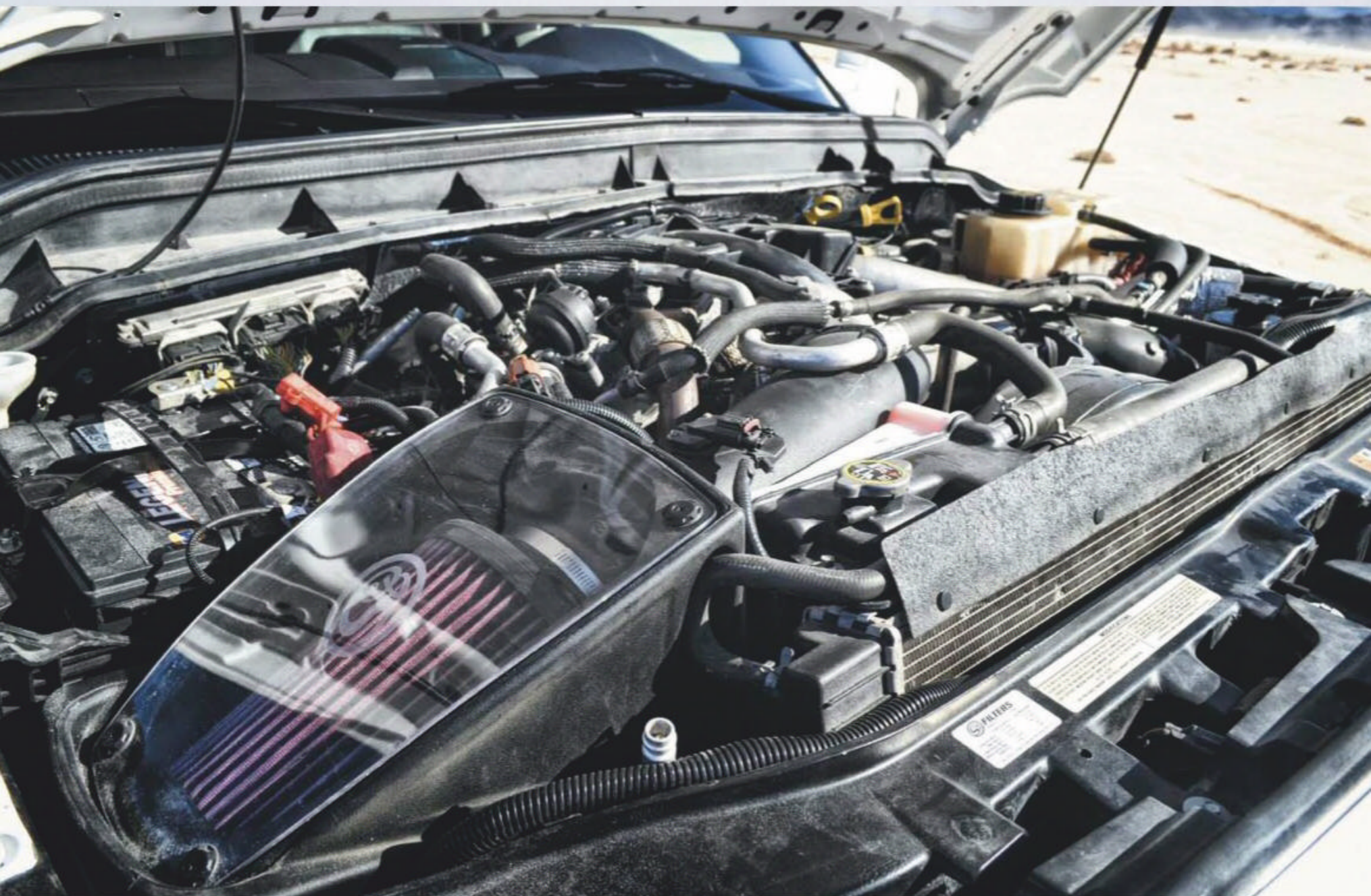
▲Other than an S&B intake, the 6.7L Ford engine is pretty much stock, and at 440 hp and 860 lb-ft, is nearly double the 250 hp that the Ford Excursion had when it was released.
