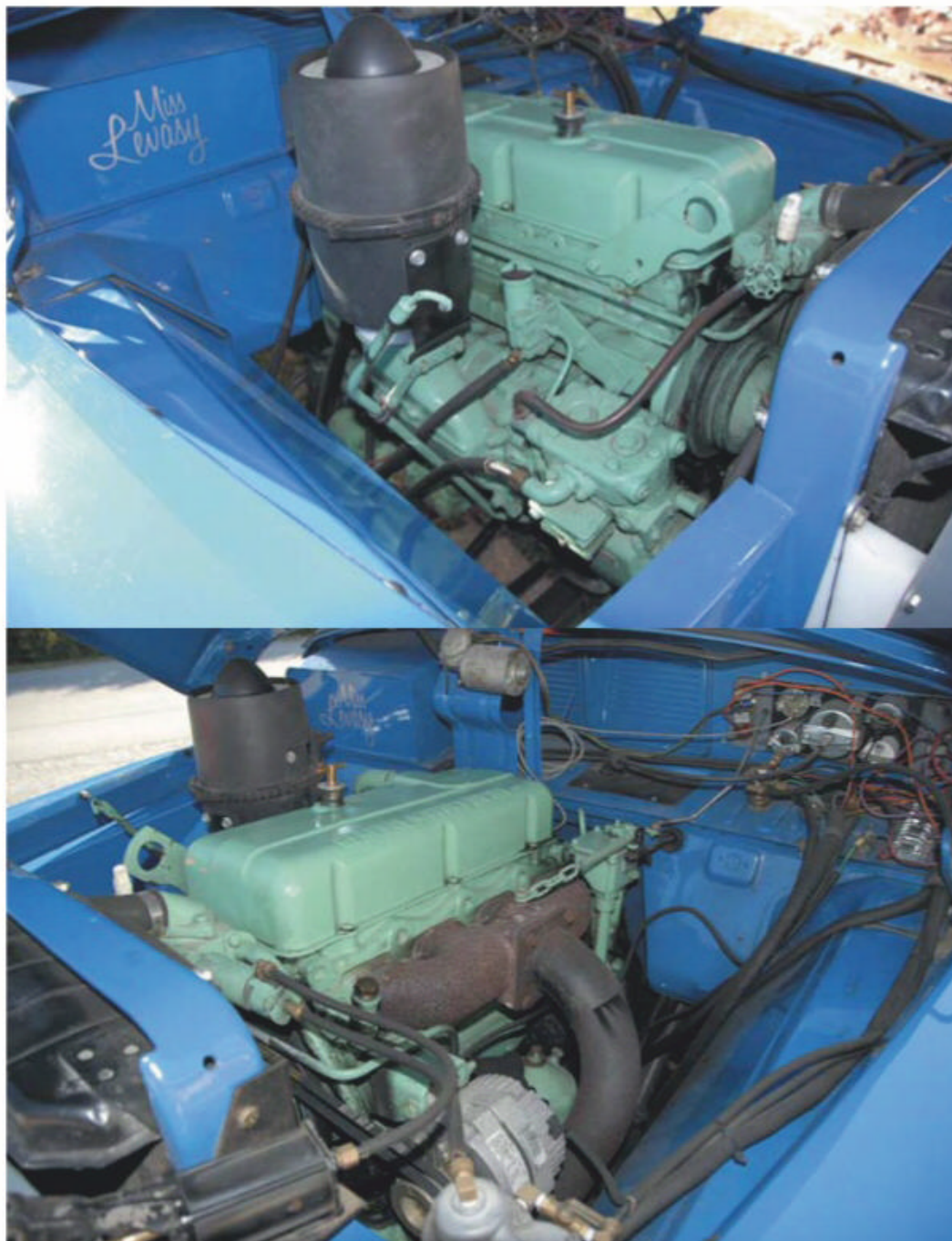
▲ The Detroit 4-53 two-stroke is modest in displacement but big in physical size, tipping the scales at 1,095 pounds. At 212 cubic inches (from a 3.875 x 4.50 bore and stroke), the output varied according to application. In the Studebakers, it was rated for 130 gross horsepower at 2800 rpm and 271 lbs-ft at 1500 rpm. Compression ratio was 17:1. Considering the 42,000 combined gross weight, gearing is paramount. With a load, Marv reports he’s working the levers constantly to keep the truck in the power band. Solo top speed is 72 mph, with the Jimmy screaming like a Banshee.
