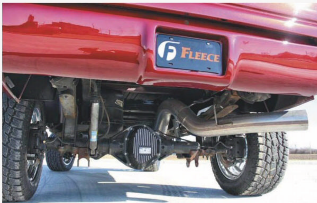
▲A Dana 80 resides in the rear, and it's been beefed up courtesy of Yukon 35-spline axle shafts and a spool. Both the Dana 80 and front Dana 60 are equipped with a 3.73 ring and pinion from Yukon as well.
