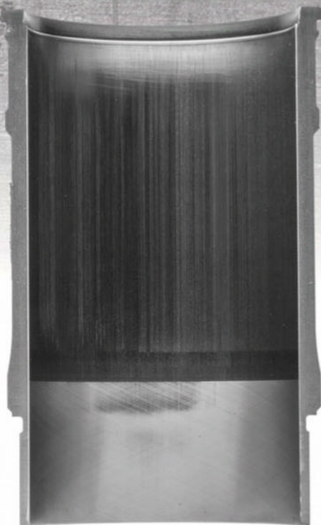
Severely Scuffed Liner After 44 Hours of Testing
