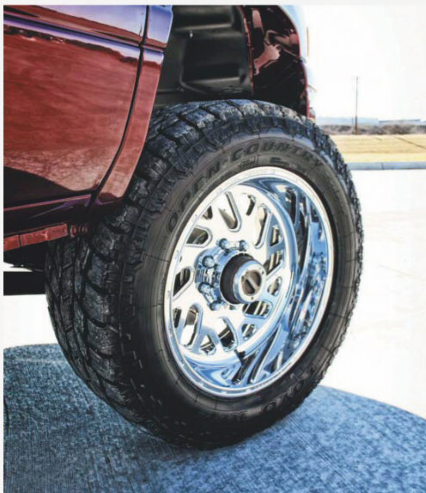
◀Polished, 20x10 Fuel Forged FF29's set the truck's appearance off in a subtle way, while 305/55R20 Toyo Open Country A/T's work to find traction. Also notice that the factory unit bearing setup has been ditched in favor of a Dynatrac free-spin hub conversion, complete with Dynoloc manual locking hubs.
