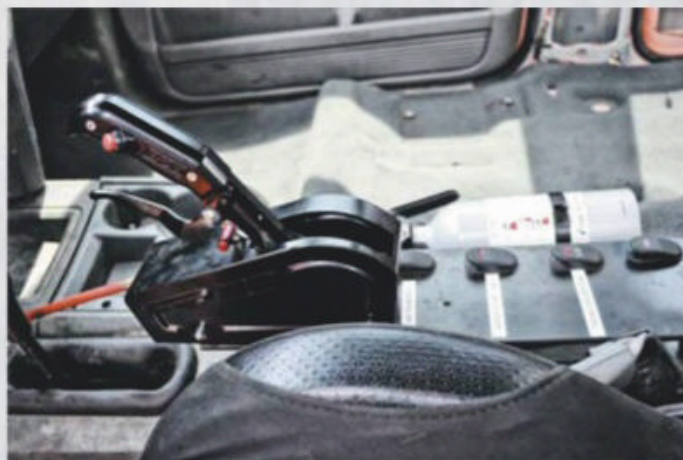
▲ So there's no mix-ups, Mitch relies on a B&M Stealth shifter for the correct gear, and also for lock-up, which is activated with a button on the side.
