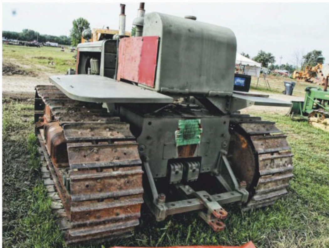
▲ Adam is missing the original PTO drive for the front winch but the original swinging drawbar is still there, less the military pintle hitch. A second fixed pintle hitch mounted above the swinging drawbar. Adam reports the running gear is fairly tight but that it needs new tracks.
