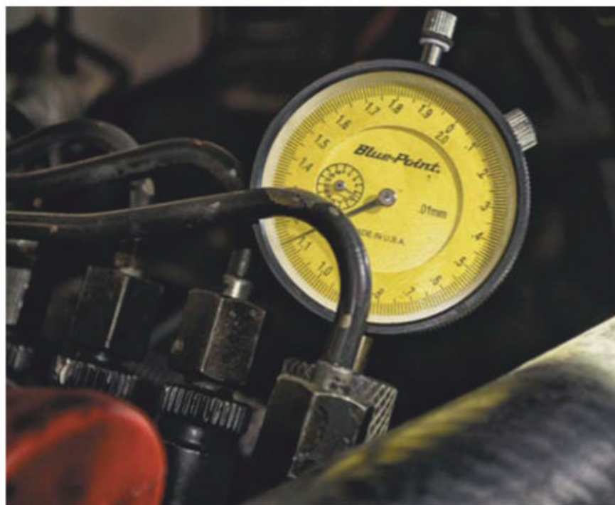
▲ From 0.0 lift, we rotated the engine forward until it reached TDC, which was measured at 5.6mm of lift, or about 12 degrees. Since factory timing was listed at 12.5 deg on our truck, we knew we were very close to TDC.
