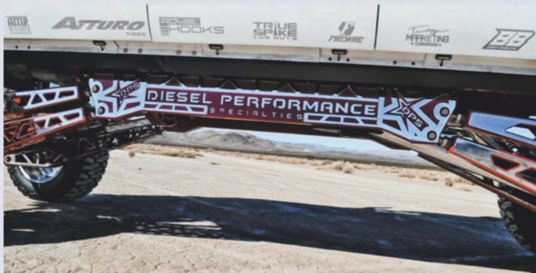
▲A complete suspension substructure was integrated into the factory frame(s), and provides a mounting point for the suspension links. Like everything else on the truck, the under-frame section received full powder coat and chrome, along with a "Diesel Performance Specialties" etching.
