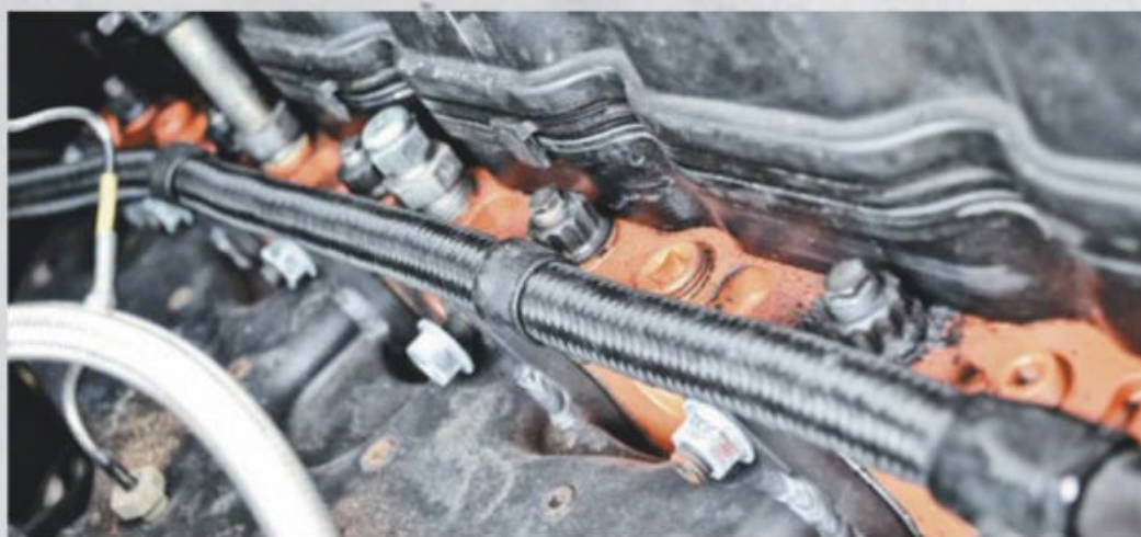
▲ Mitch wasn’t taking any chances and performed a full rebuild on the Cummins, including a set of ultra-tough head studs from Extreme Studs.
