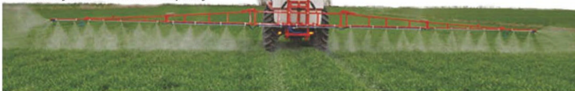
Mounted Boom Sprayer Semi Hydraulic 1000 Litre capacity
