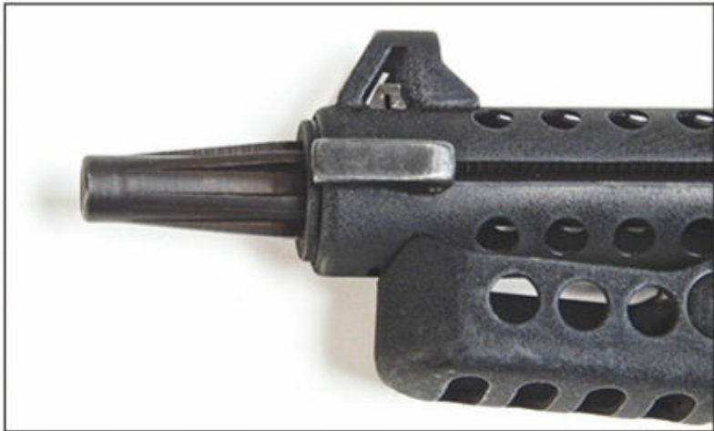
The Z-70's non-reciprocating cocking handle folded forward; also visible is the muzzle and the butt stock in the folded position.
