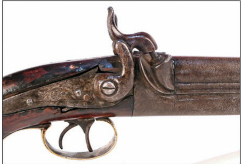
Each nipple is obviously plumbed to a different barrel.
