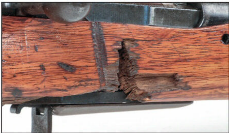
This shot-up Type 99 rifle caught two .30-caliber rounds directed from the top. The resulting damage tells a story.
