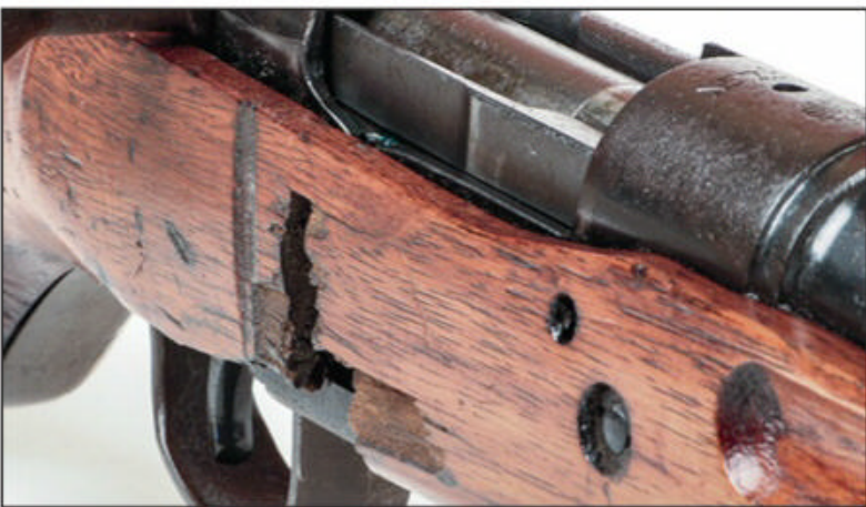
This shot-up Type 99 rifle caught two .30-caliber rounds directed from the top. The resulting damage tells a story.
