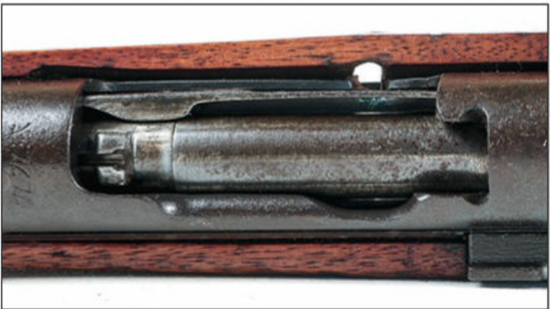
The geometry of the bullet track would have taken it through the rifle's extractor. The lack of associated damage leads me to believe it was hit with the bolt open. When I bought the gun it did not have a bolt.
