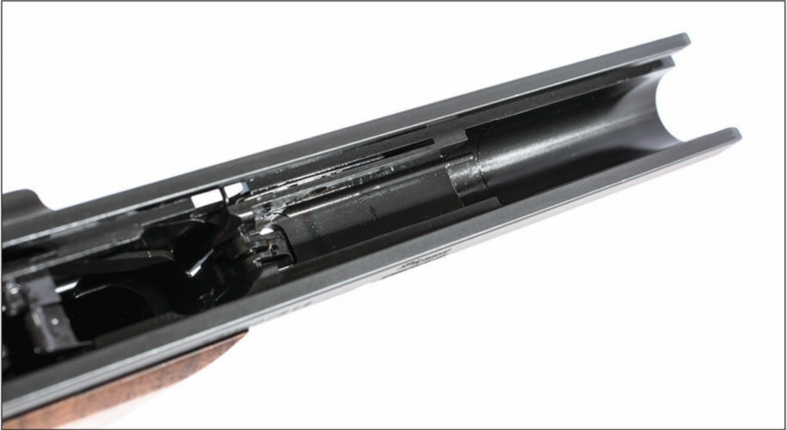
The frame rails go the full length of the frame and its dustcover.
