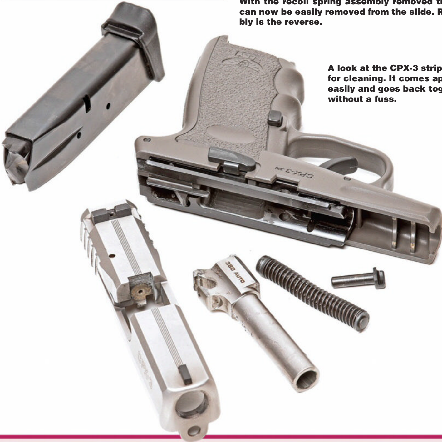
3 Turn the slide over and remove the captured recoil spring assembly.
