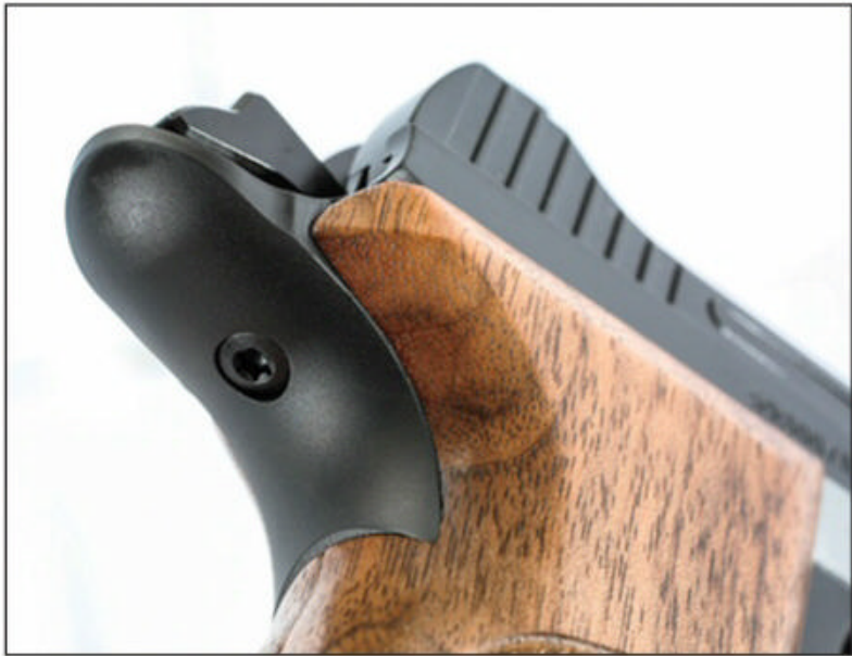
Here is the screw holding the trigger packet assembly in the frame. No need to do anything with this at all.
