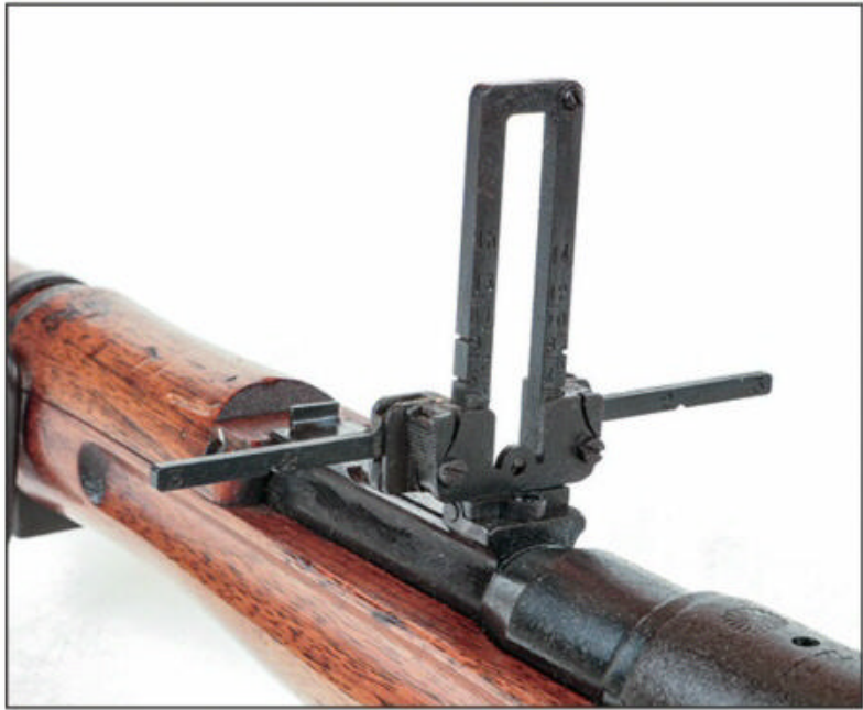
Early Type 99 rifles included a delightfully complicated anti-aircraft sight that was supposed to aid in determining lead on a moving aircraft.
