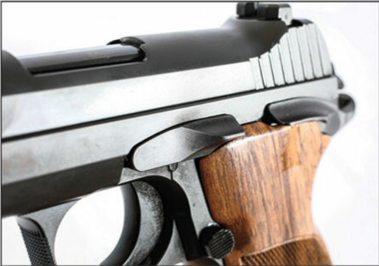
The P210 thumb safety and slide stop are machined to a different contour than that of the originals.
