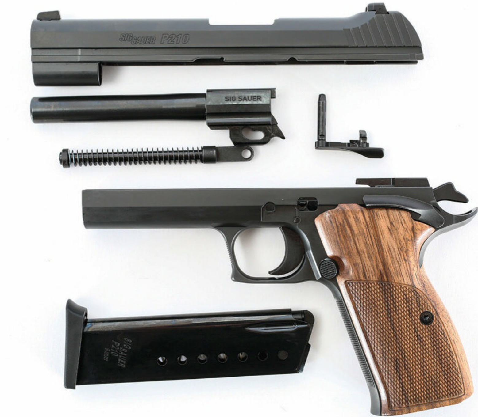
This is where you need to get to, to do basic cleaning. You can remove the grips if you feel the need.
