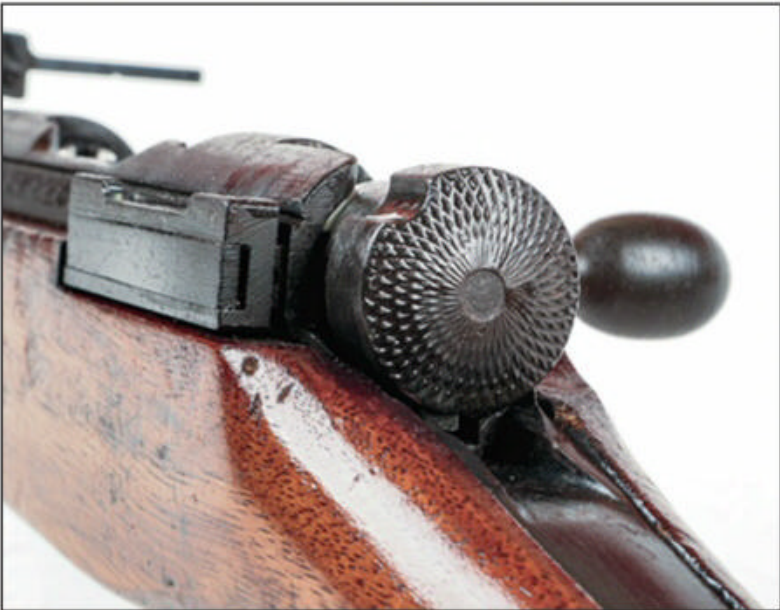
Before the war turned against the Japanese they invested remarkable resources in producing their weapons. The complex knurling on the safety knob of this Type 99 is a good example.
