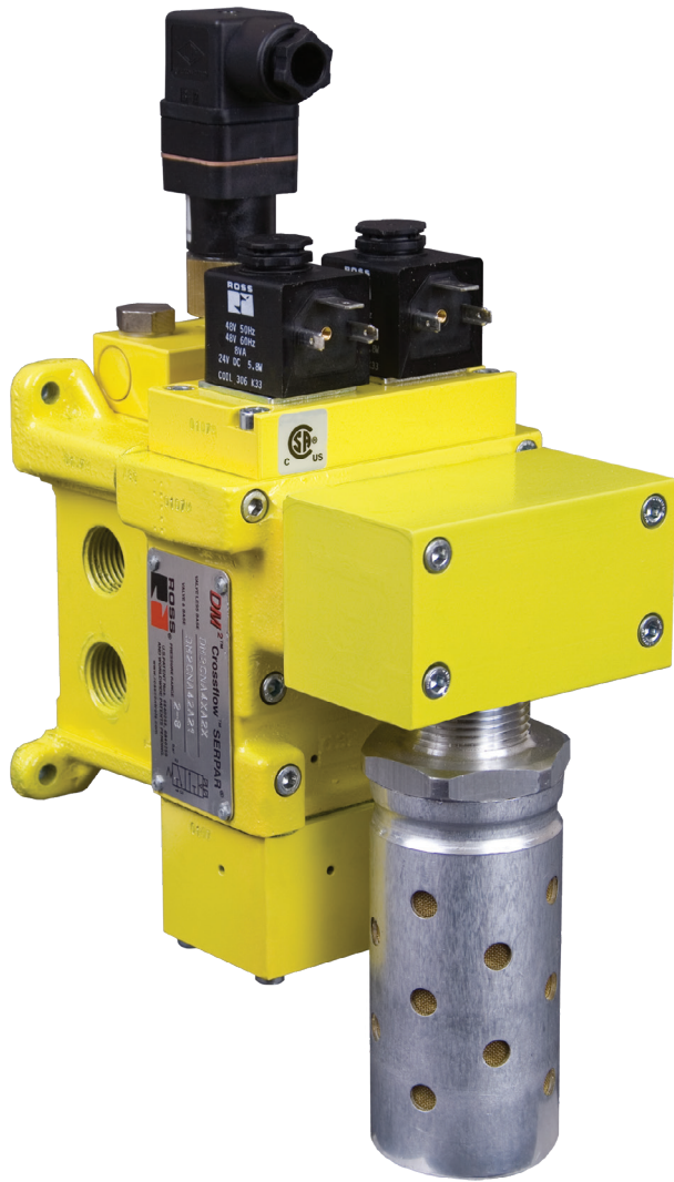
Figure 1. The DM2 series valve from Ross Controls is a 3-way, 2-position normally closed valve that blocks primary inlet pressure from reaching downstream, while ensuring that downstream pressure is vented to atmosphere.
