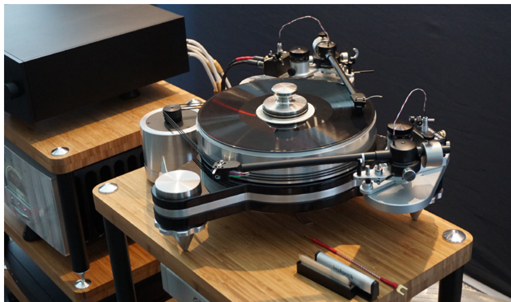
VPI's new belt-driven Avenger turntable uses multiple drive belts to share the platter-spinning workload
