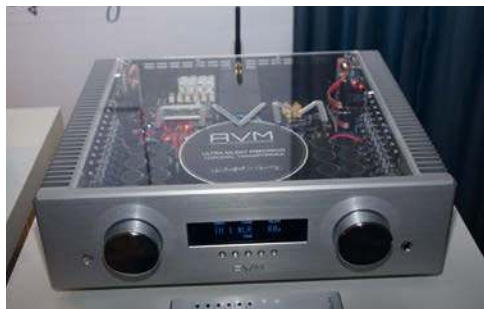
AVM's $17,390 A8.3 integrated amplifier is capable of delivering 200W per channel, sports analogue, digital, and next-gen Wi-Fi audio inputs, and even features a custom-made Class A headphone stage.
