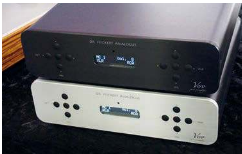
Dr Feickert Analogue's new Ver0 phonostage (€4900) features two completely independent analogue circuits, one optimised for moving coil cartridges and the other for moving magnets.
