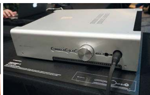
Schiit Audio's $1,499 Ragnarok 2 headphone amp delivers 60 Wpc @ 8 Ohms or 100 Wpc @ 4 Ohms! The amp features a revised differential gain stage and optional DAC/phono modules.
