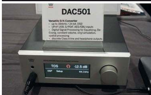
Weiss demonstrated both its DAC501 ($8,000) and DAC502 ($9,000) DAC/headphone amplifiers. These support PCM to 384kHz rates and DSD to DSD128, and feature clever DSP for headphones.
