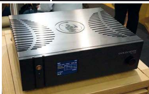
Analogue specialist Gold Note debuted its flagship PH-1000 phonostage (€5900), which offers three cartridge inputs, 12 EQ curves, and multiple impedance settings—all via remote control.
