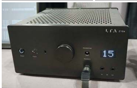
The $6,950 Linear Tube Audio Z10e is a 12 Wpc electrostatic headphone amplifier that is also capable of driving virtually any dynamic or planar magnetic headphone, and even some speakers!
