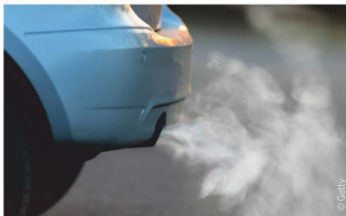
The product of a car's combustion engine is around 13% carbon dioxide, 13% water and 73% nitrogen
