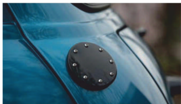
Boot features a Concept 7-gallon tank.
