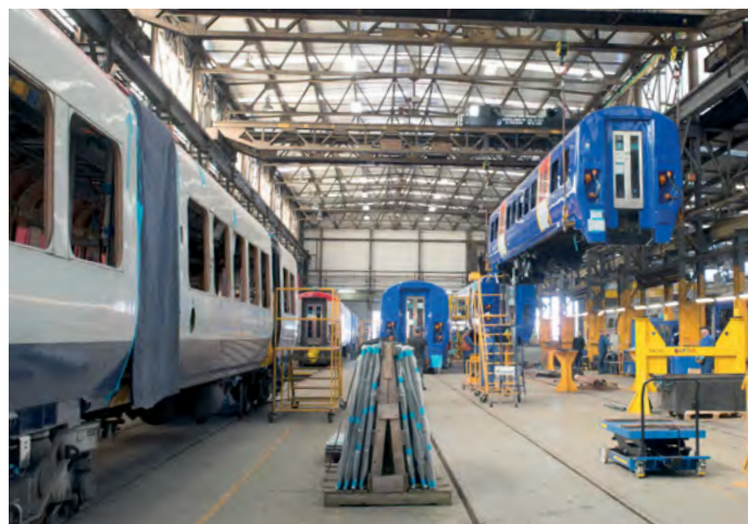
Destined for a new route: Class 460 units, previously used on the Gatwick Express service, are pictured during conversion to Class 458/5s at Wabtec Rail Doncaster in April 2013. Richard Tuplin
