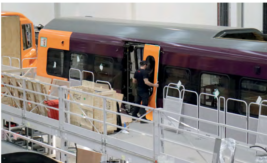
Door fitment: this is part of the second stage in the assembly process.
