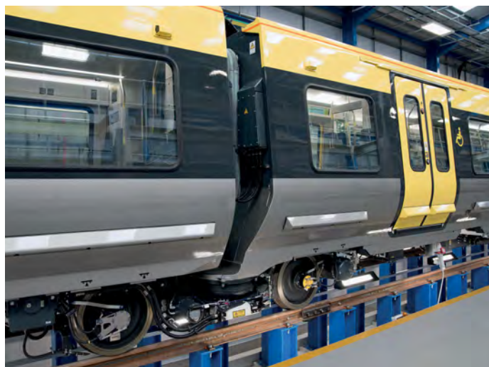
Articulated vehicles: note also the bodyside deflector designed to prevent people becoming trapped between the train and platform. Tony Miles
