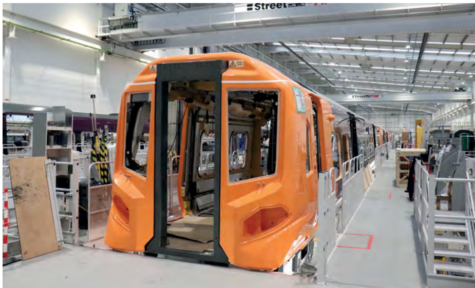
Assembly underway: a Class 196 bodyshell in the first of the five zones in the production process. The '196s' are the first trains built by CAF for the UK to have corridor connections between units.
