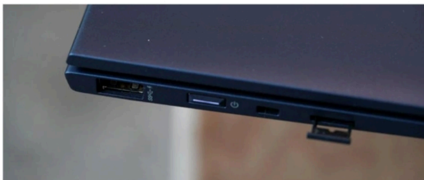
The Elite Dragonfly's left side features a USB Type A port, a power button, a lock port, and a SIM slot.
