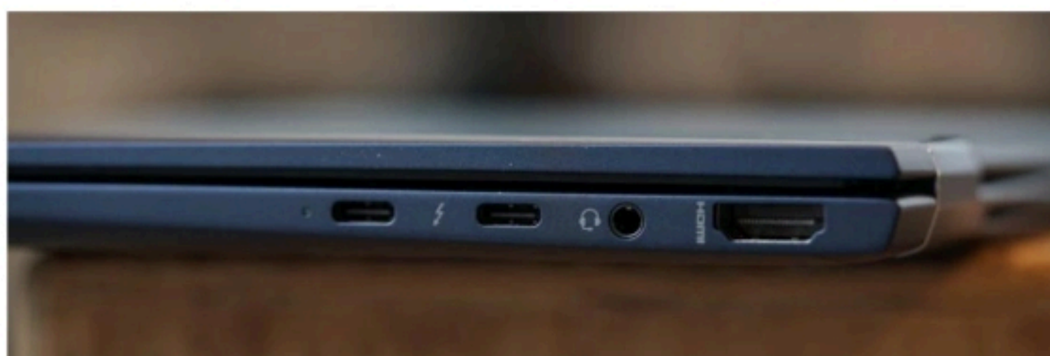
Despite its relatively thin body, the Elite Dragonfly still features USB Type A and full-size HDMI ports, along with two Thunderbolt 3 ports.
