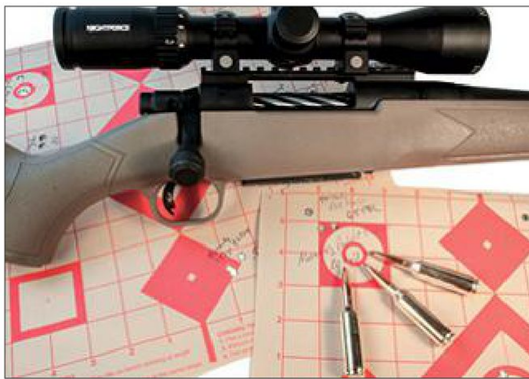
The Patriot Predator averaged sub-m.o.a. with all ammo at 100 yards and carried that accuracy to 200—as evidenced by this 0.8-inch group (shown with cartridges).
