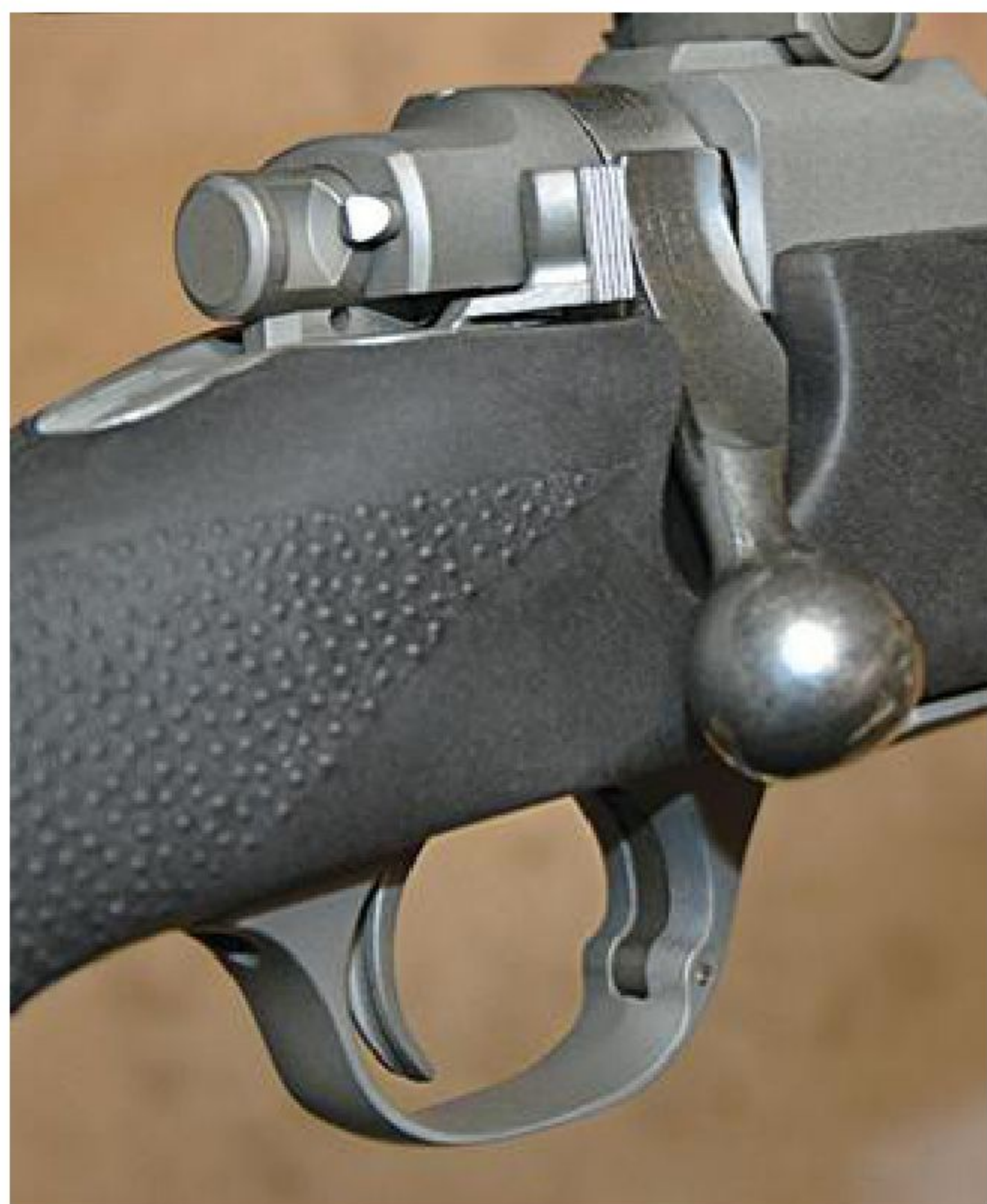
Pulling the Hawkeye's safety all the way to the rear for Safe cams the small pin protruding from the rear of the bolt shroud forward to prevent the bolt from rotating.
