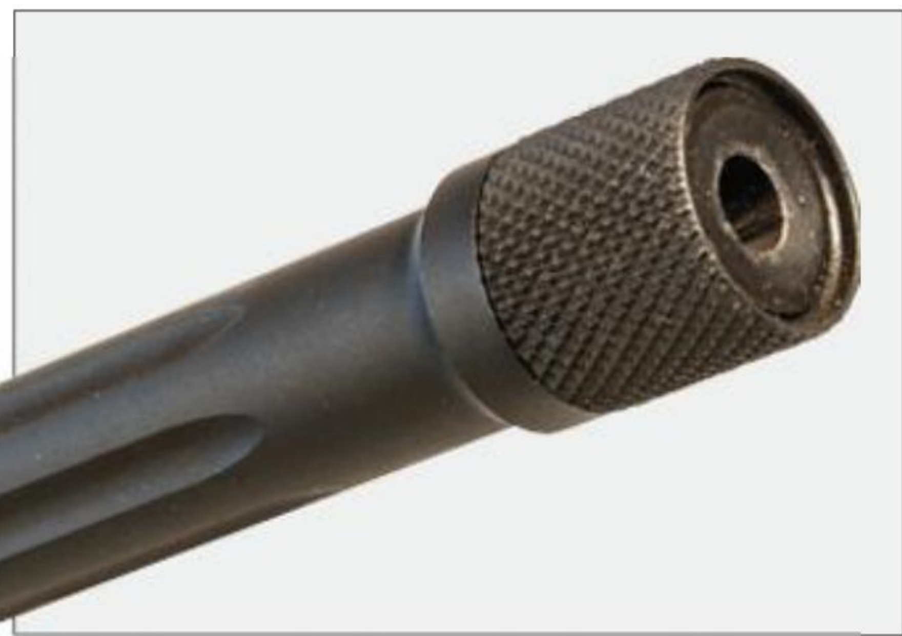
The 22-inch barrel is fluted, and it's threaded 5/8x24. The muzzle looks a bit ungainly, but the design allows for a slimmer barrel and therefore a lighter gun.
