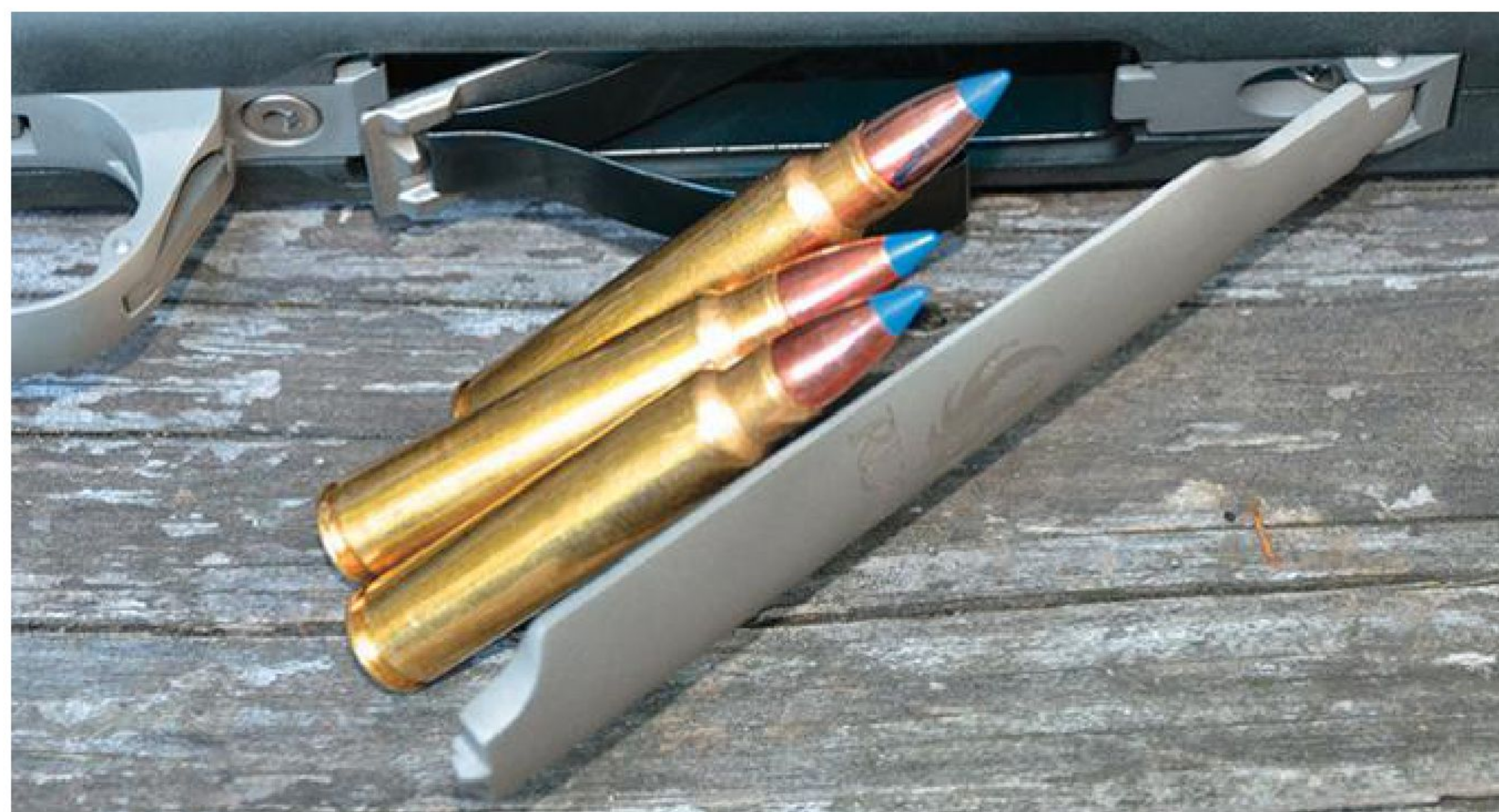
The magazine holds three .375 Ruger cartridges, and its floorplate release fits flush with the front of the trigger guard.
