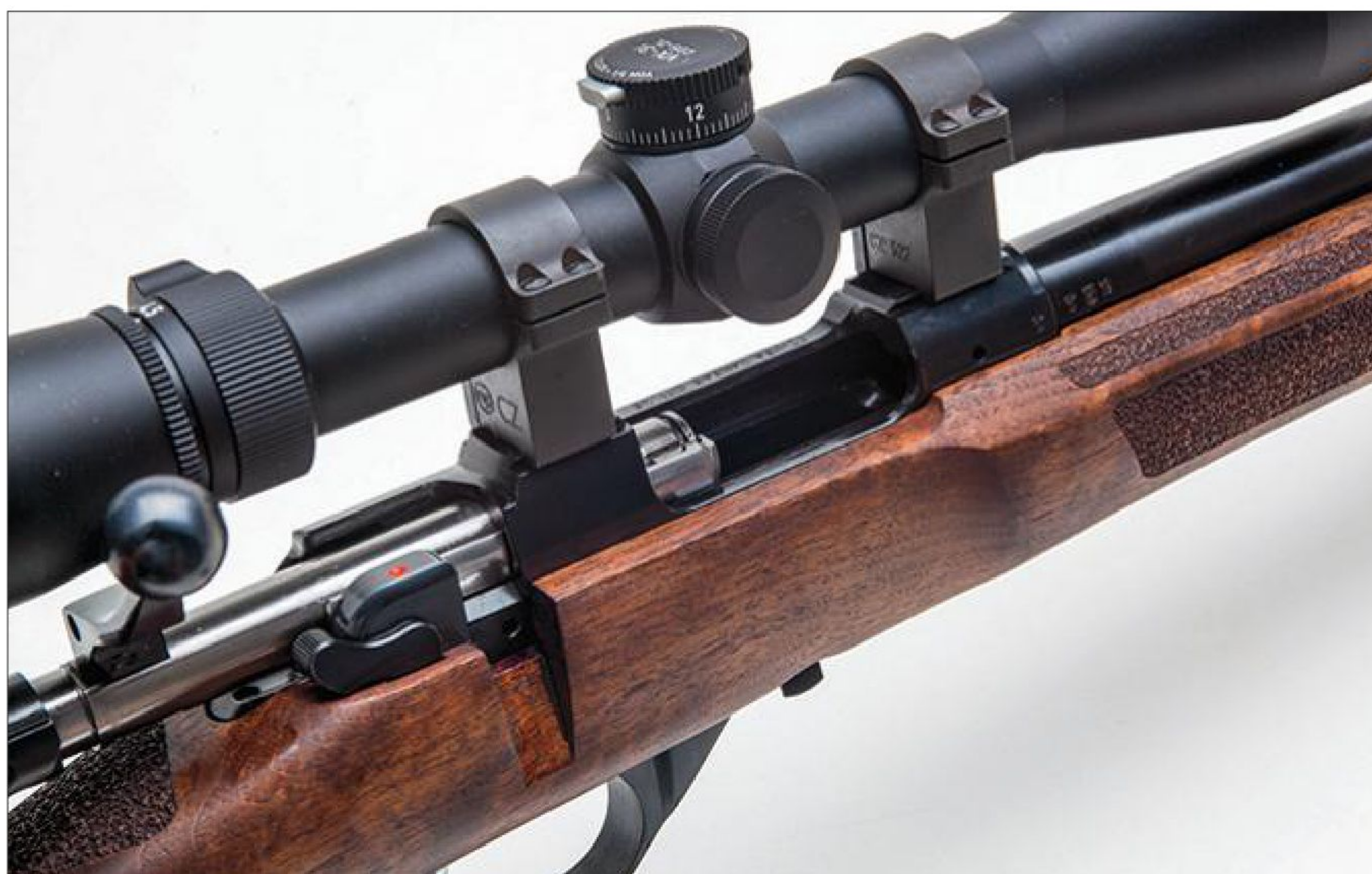
The 527 uses a micro-Mauser action with a true controlled-round-feed bolt and fixed ejector. The top is grooved 16mm for dovetail scope mounts.
