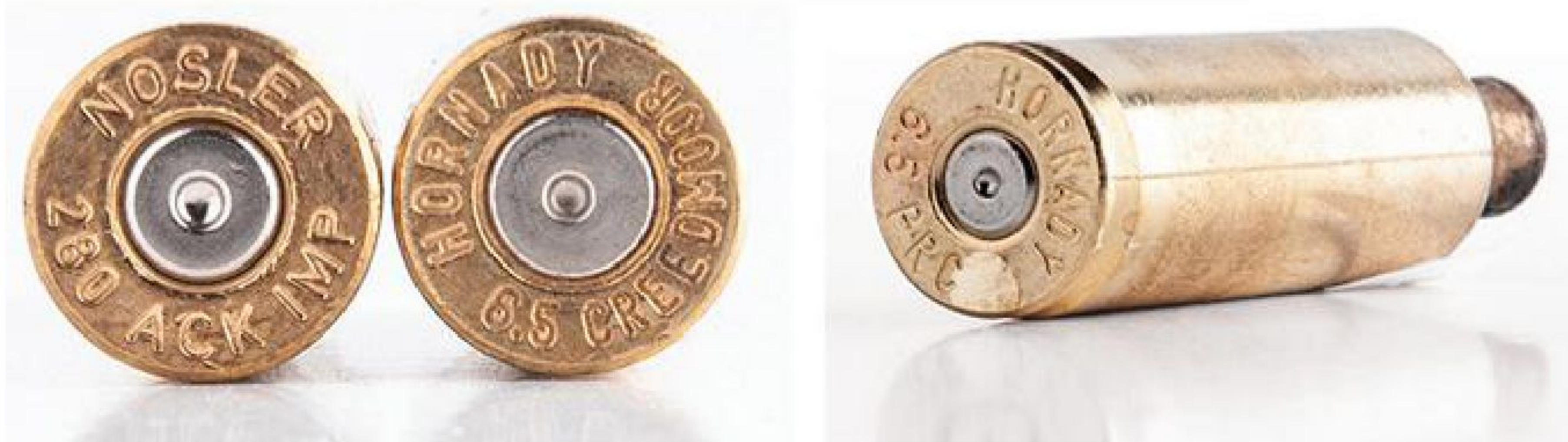
(Top) Sticky bolt lift results from over-expansion of a fired case. (Bottom l.) The primer on the left is normal, while the one on the right is flattened. (Bottom r.) An extractor smear is a sure sign of an over-pressure load.
