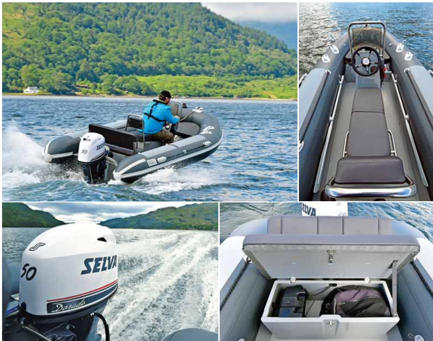
1. A great, fun little boat. 2. Simple, neat layout. 3. With the Selva rigged the 4.5m Fjordstar gave us 29 knots. 4. The aft locker is a complete box, so the interior remains dry.
