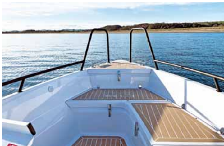
Deck lockers are secured with adjustable catches.
