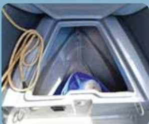
Note the flange around the chain locker to keep water out.
