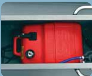
25-litre fuel tank fits in the jockey with room for another 12 litre tank and gear on top.
