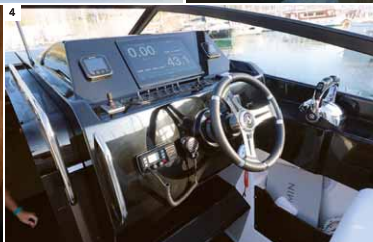
3. The fore V-berth is large and there is more storage than you might expect. 4. Wheel and throttle lie to hand. Huge MFD is glorious. Note left-hand thruster joystick.
