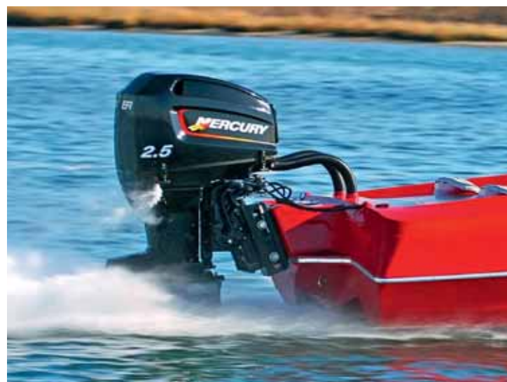
Fig 5: Engine height can play a key role in mitigating chine walking.
