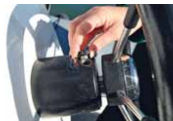
Hydraulic fluids may need topping up
