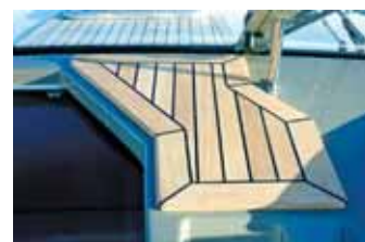
Boarding platform, foredeck, cockpit sole and steps are capped in teak.
