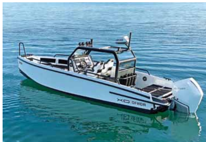
Even with side screens removed, the wheelhouse cage provides good protection.
