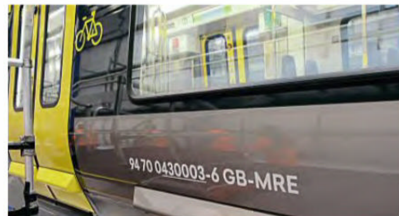
The individual vehicles feature full UIC numbering - here driving car 430004 is prefixed by the type code 94 (EMU) and country code 70 (UK), and is followed by check code 6. GB-MRE is the keeper code for Merseyrail
