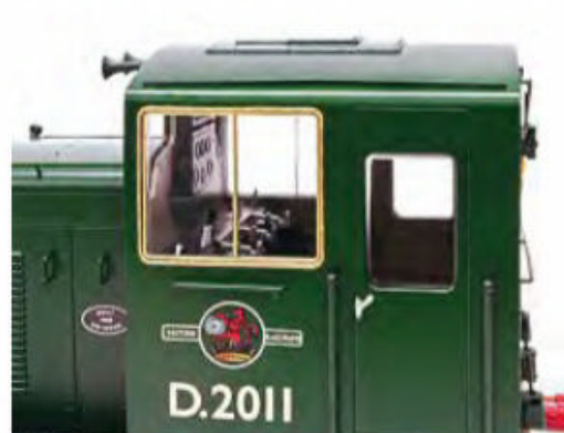
Clear flush glazing is applied to the cab, which allows a good view of the driving desk detail inside.
