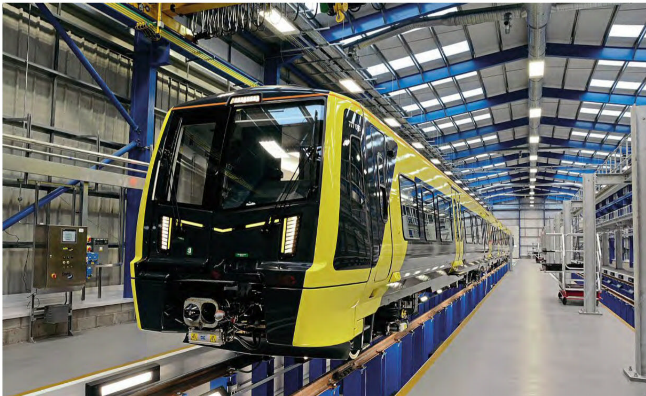
Four-car No. 777003 is the first of the 52-strong fleet to arrive on Merseyside, and is pictured inside Kirkdale depot for commissioning work. Note the unit number is above the cab side window. All photos taken on January 28 by Paul Bickerdyke
