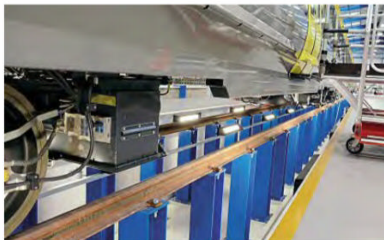
There is room under one of the driving cars for traction batteries to be fitted in the future if required.
