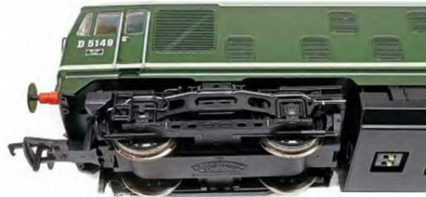
Bogie frames are very crisply moulded and enhanced with separate parts for sand boxes, sand pipes, brake details and the speedometer cable. Weight-saving holes are present in the equalising beam and wheels, a feature of the Class 24s.
