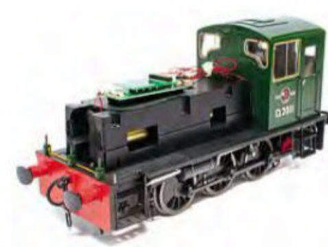
The mechanism is confined to the front of the locomotive, leaving the cab clear for detailing. A 21-pin DCC interface socket is fitted.
