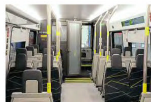
The passenger saloon behind the cab. The doorway should usually feature clear glass to give passengers a forward view, although electronics allow it to be made opaque by the driver if required.
