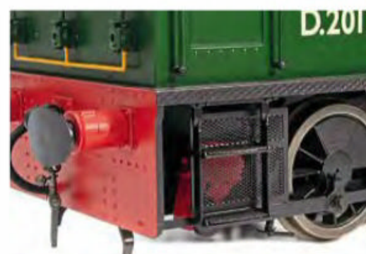
A view of the footstep, safety screen and the crank located behind the screen, all neatly assembled.
