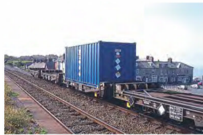
Square NUPAK containers have been used to carry intermediate-level nuclear waste to Sellafield from several locations, including Berkeley, Drigg, and Dungeness. These containers sit on their own bespoke carrying frame that is used when transferring them by road to and from a railhead, and PFA No. DRSL 92723 was carrying two NUPAKs when spotted at Sellafield bringing up the rear of the local trip from Drigg on April 12, 2005.
