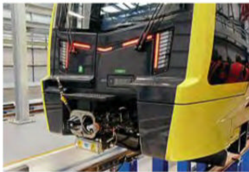
A close-up on the automatic coupling. The emergency exit door is above to the left.
