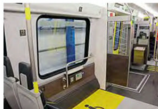
There is space for two wheelchair users, while the gangway is wide enough for prams and wheelchairs to pass.
