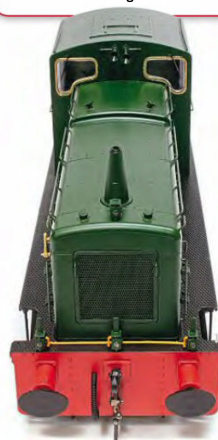
Fine wire hand rails and an etched radiator grille are neatly applied to the injection-moulded plastic bonnet.
