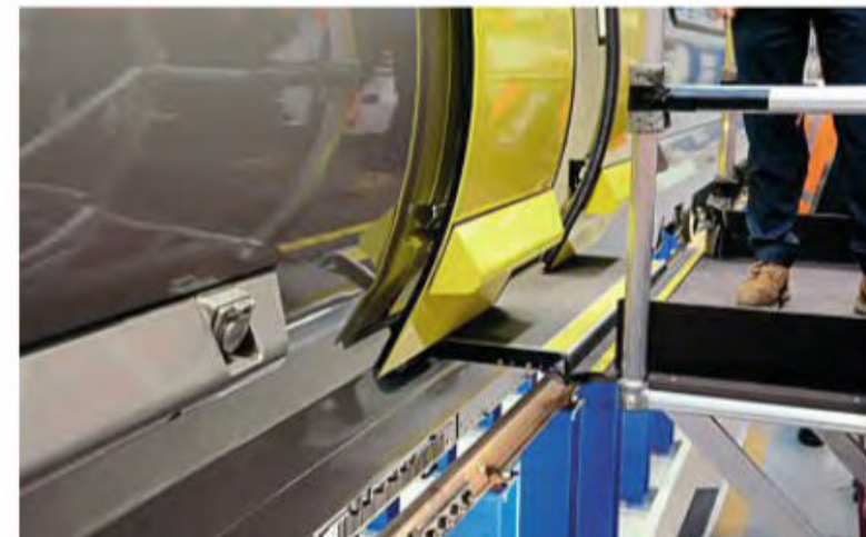
A quick-action ramp slides out at platform stops before the doors open. This gives level access for wheelchairs and prams.
