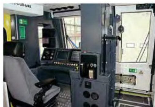
The cab with driver's position to the left, which offers more room than the current Class 507/508 units, and the emergency exit door to the right.
