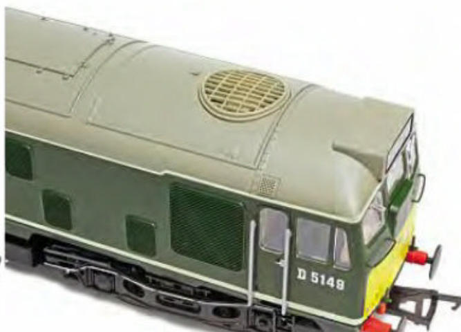
The No.1 end roof fan grille which is a separate plastic moulding.
