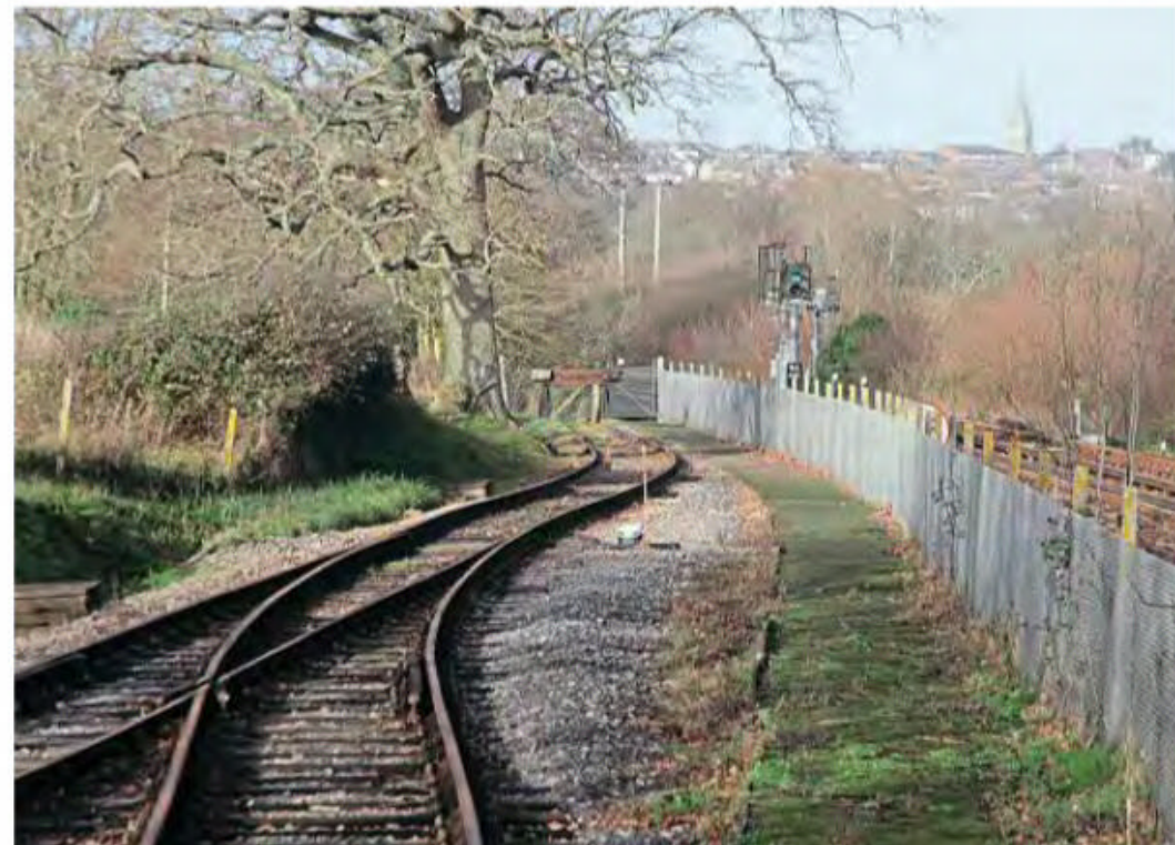
Looking north at the former Smallbrook Junction on December 21, 2018, where a connection could be reinstated between the Isle of Wight Steam Railway (left) and Island Line (right) to make stock movements and engineering trains possible.
