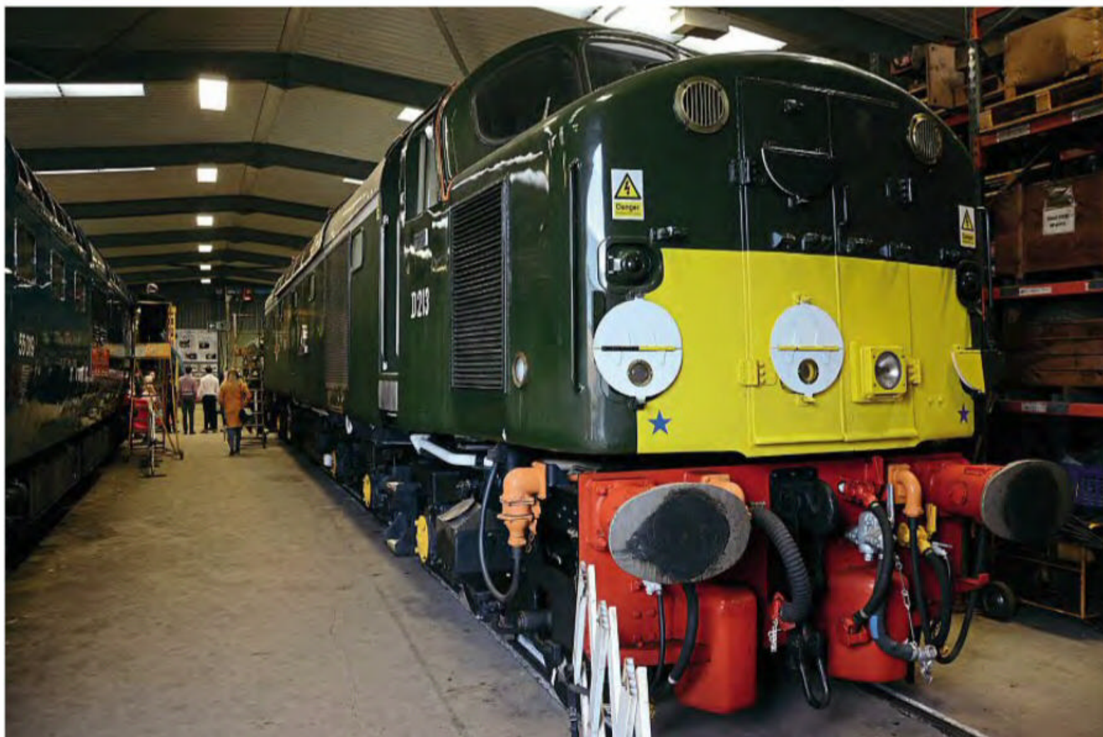
'WHISTLER' REPAIRS: Class 40 No. D213 Andania , which is on hire to Locomotive Services, has undergone a power unit strip at Barrow Hill following a big-end bearing failure that was discovered during an inspection. Repairs are also being carried out to a bent crankshaft. It is hoped that the loco will be back in working order in the spring. The '40' is pictured in the Deltic Preservation Society's shed at Barrow Hill on December 6, 2019. Paul Bickerdyke
