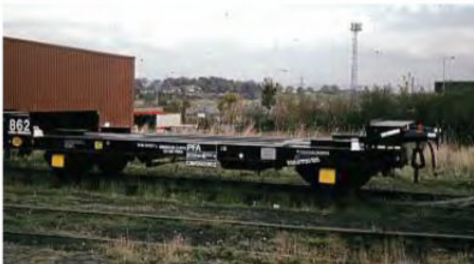
The wheel protection sections welded to the wagon floor are evident in this view of empty PFA No. CAWD92862 seen at Heywood in October 1987.
