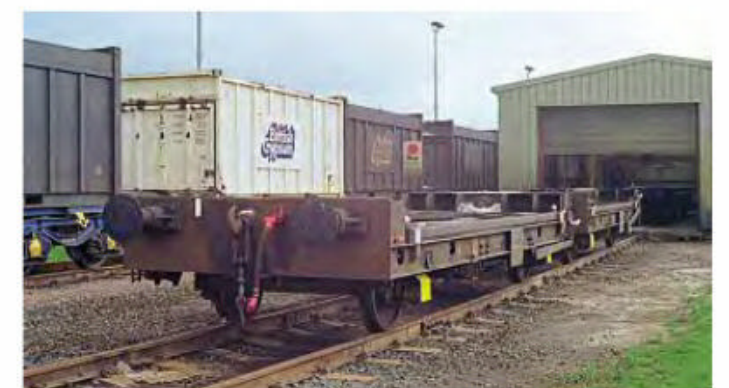
To effectively raise the floor height to permit the carriage of flat bottom containers, British Gypsum fitted their wagons with a framework as illustrated by this view of Nos. BGL95338 and BGL95349 at Newbiggin in July 1997.
