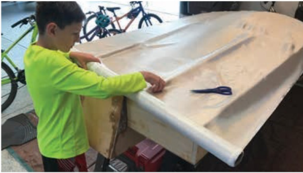
Rolling out fiberglass to reinforce the bottom of the boat.
