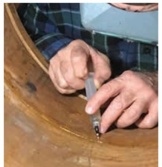
WEST SYSTEM 105/205 was injected directly into the crack and clamped to cure.
