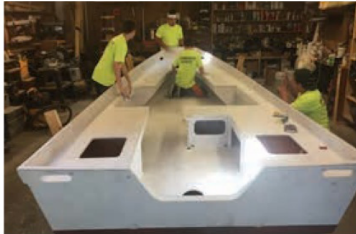
Primer being sanded before final coating.
