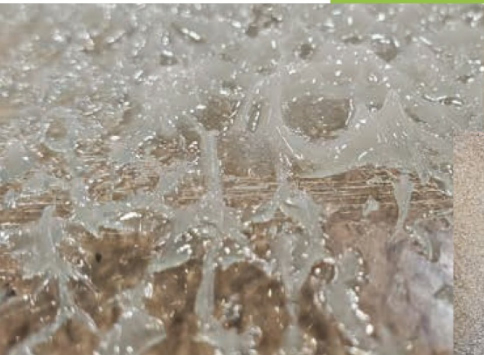
Texture built with a roller cover for aggressive nonskid.
