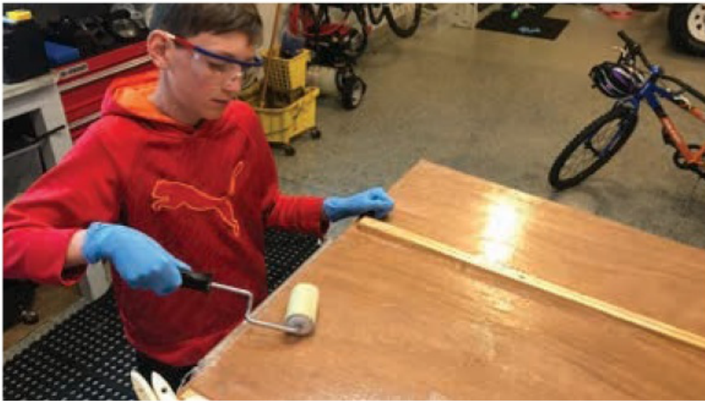
Epoxy was rolled on to wet out the fiberglass reinforcement.
