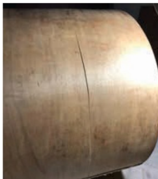
The drum had a severe crack a third of the way around the drum on the grainline.
