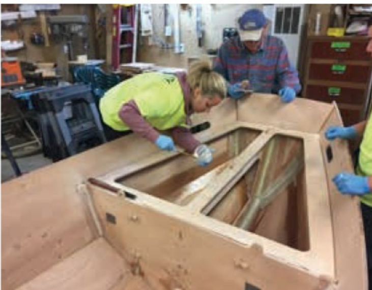
Fillets were applied along the joints along with 17 oz. fiberglass tape for reinforcement on major joints.
