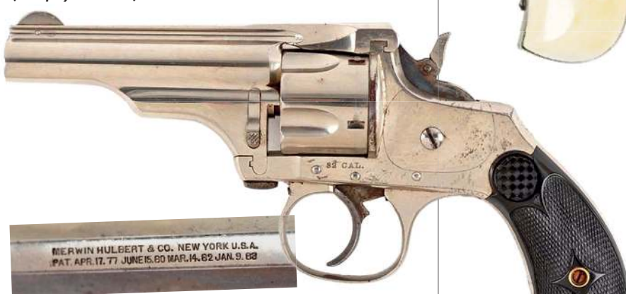
Marks found on the barrel of a Merwin & Hulbert show the earliest date on which the gun could have been made - that of the latest patent (Morphy Auctions)
