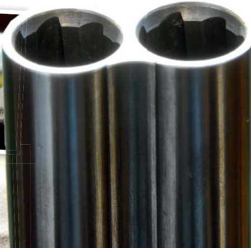
Muzzle details showing the distinctive Paradox rifling of rifle 15708
