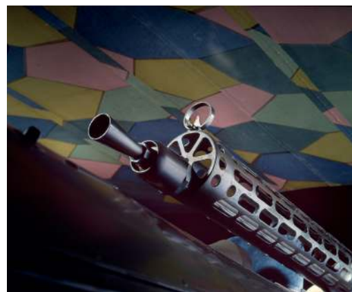
One of two deadly machine guns mounted on the D.VII. By the time this plane came out all of the problems with the synchronised interrupter gear had been solved ( National Air and Space Museum )
