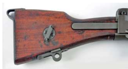
The butt of the Mk II Bren, showing the shoulder rest made simply by folding a sheet-steel plate, and the bracket for the rarely issued monopod ( Morphy Auctions )
