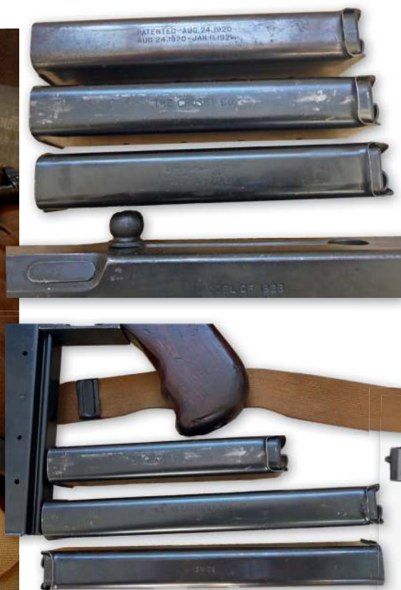
Above: SWCO, Crosby and Seymour, (fitted to M1A1), 30-round XXX magazines, with a 20-round XX magazine for comparison
