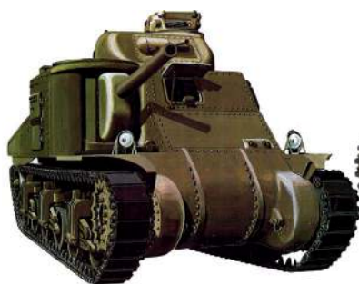
M3 Lee-Grant Tank, obsolete in Europe by 1944, but still formidable in SE Asia, with a 75mm gun in the hull and a second 37mm gun in the turret (Purnell Publishing)
