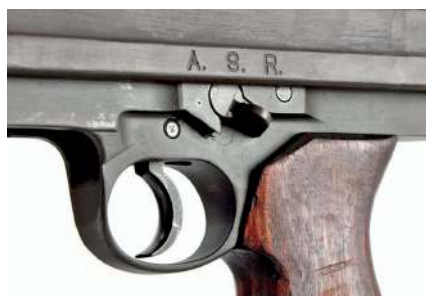
The fire-selector of the Bren - 'A.', automatic fire; 'S.', safe, and 'R.' for repetitive (single-shot) fire ( Morphy Auctions )
