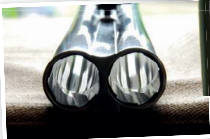
Muzzle details showing the distinctive Paradox rifling of rifle 15708
