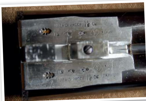
The barrel flats showing the London proof marks for rifle No. 15708
