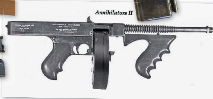
The second version of the Model of 1919 Annihilator II, fitted with the 50 round L drum
