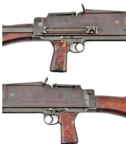
The body of the Mk II Inglis Bren, showing the fixed charging handle on the right and the selector on the left side above the trigger ( Morphy Auctions )
