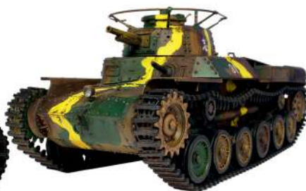
Japanese Type-97 Chi-Ha Medium Tank, the mainstay of Japanese armour with a 37mm gun, 7.7mm machine gun and crew of only two (dragonmodels.com)
