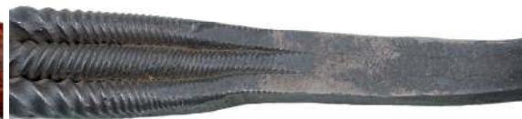
The twisted bars are hammered to form a single strip or riband
