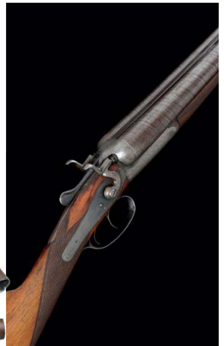
A.W. Gamage. A plain quality 12-bore hammer gun, c. 1900, with plain finish and plain laminated Damascus barrels
