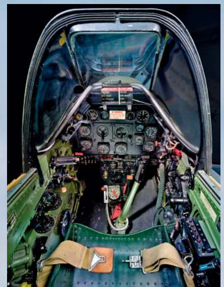
The cockpit of a Mustang left no room for anything not absolutely necessary for the operation of the fighter ( National Air and Space Museum )
