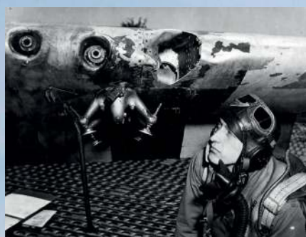
Howard Spaulding of the 375th Fighter Squadron inspects the battle damage to the left wing of his P-51B
