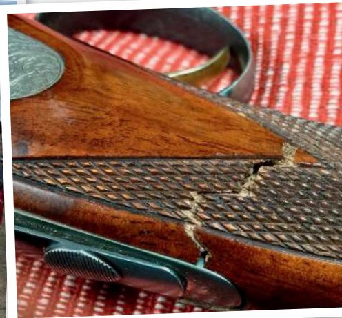
A cracked wrist such as this will require skilled work from a gunsmith to repair. This can cost many hundreds of pounds
