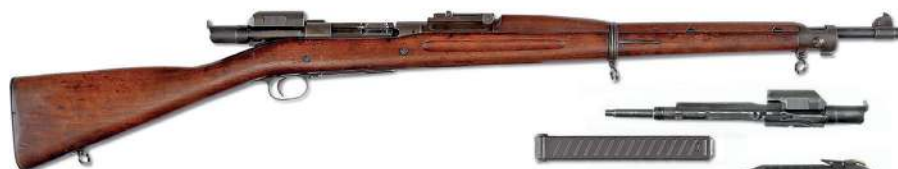
The Pedersen Device, or US Automatic Pistol, Caliber .30, Model of 1918, was effectively a pistol replacing the M1903 rifle bolt (Morphy Auctions)
