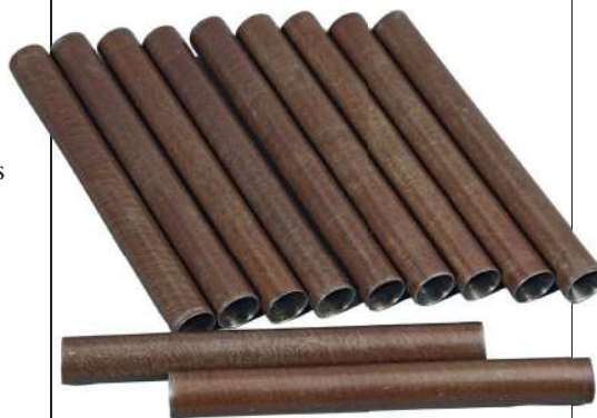
A set of gunmakers sample tubes, showing the different styles and patterns of Damascus tubes available
