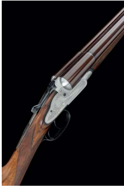
W.H. Monks. An unusual 12-bore sidelock non-ejector gun with Monoblock Damascus barrels, c. 1880, the two stub twist tubes sleeved in to the solid Damascus breechblock
