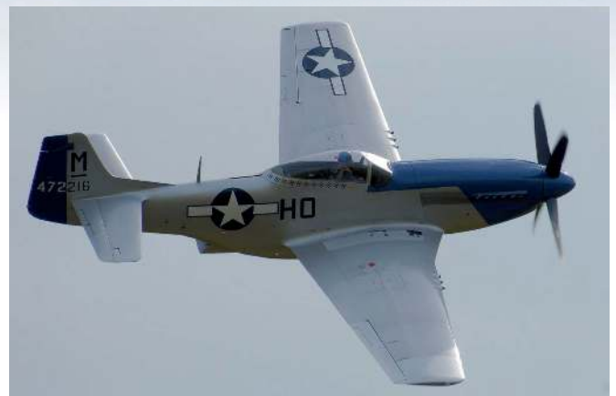
A beautifully refurbished P-51D with the bubble canopy and dorsal fin modifications soars in all her glory
