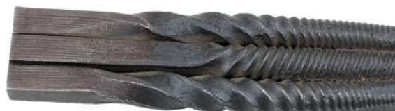
The three stubs clearly showing the iron and steel layered construction as they are twisted together
