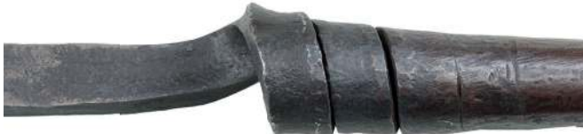
The riband is twisted around a mandril and welded together to merge the finished tube
