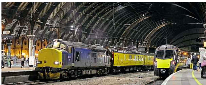
Class 37 No. 37612 works in top-and-tail mode with 37610 on a Derby to Scarborough track-recording train on February 10. It is seen under the roof at York station as a Grand Central Class 180 waits to go south. ANDREW JEFFREY
