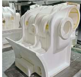
One of the two sacrificial polystyrene patterns for No. 4709's new cylinders sits at Premier Patterns on February 7. 4709 PROJECT
