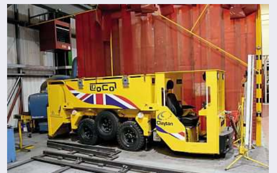
RD001 Diane , spotted in Clayton Equipment Ltd's Burton-on-Trent works on January 28, is a low-cost, 2ft-gauge mines demonstration loco. Its rubber tyres provide increased adhesion compared with conventional steel railway wheels. ALISTAIR GRIEVE
