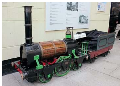
One of the larger locos on show at Brass, Steel and Fire is this 12¼in-gauge 2-2-2, on loan from the Head of Steam Museum, Darlington. It carries a builder's plate reading 'Leatham & Co, Engineers, Heath near Wakefield'. Extensive research into the loco and its origins by Richard Ellam concluded it was probably completed by a young Albert Leatham in the late-1830s or early-1840s. Picture: PETER NICHOLSON
