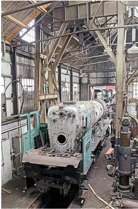
With the boiler back in the frames, work can begin to rebuild the rest of the loco.
