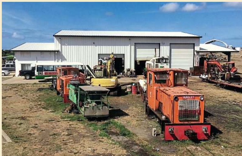
The two Hunslet locos at the wonderfully named Needsmust depot, both in orange livery. On the right, 160HP loco No. 15 (Hunslet 9086/1982) and on the left out-of-use 101 HP loco No. 14 (Hunslet 5218/1958). One of the mainly white-liveried Romanian-built locos used for passenger trains can be seen in the background. ANDREW GARRETT
