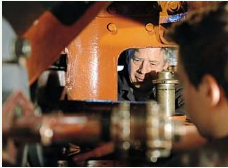
Above: The valve and cylinder liners, shrunk in liquid nitrogen, are fitted to the cylinders of 'Pendennis', with staff making the motion adjustments after fitting.
