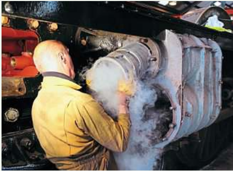
Above: The valve and cylinder liners, shrunk in liquid nitrogen, are fitted to the cylinders of 'Pendennis', with staff making the motion adjustments after fitting.
