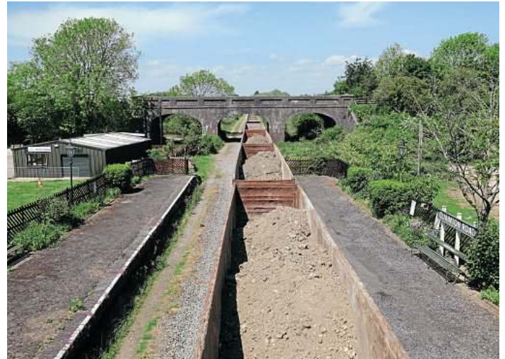
Correctly loaded dry spoil train passing Quainton Road. Wet spoil or overloaded wagons can trigger weigh indicators in the control centre. PHIL MARSH
