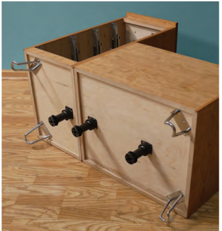
Three black adjustable leveler legs — one under the drawer cabinet and two under the bench — provide added support to the metal hairpin legs/feet when this project is used as a seat.
