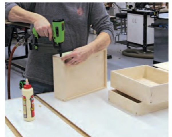
Their butt joint construction makes these four drawers quick and easy to assemble with glue and 1 1/4" brad nails.
