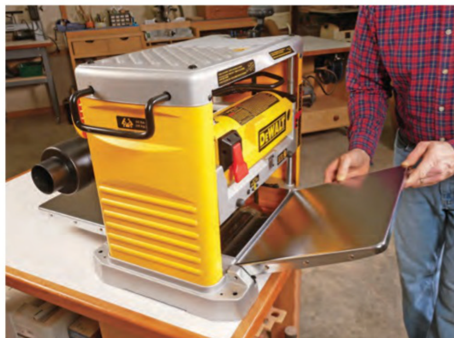
Infeed and outfeed tables provide added support for long stock and help reduce the tendency for them to tip, which can exacerbate snipe. On benchtop models, these tables fold up for more compact storage.
