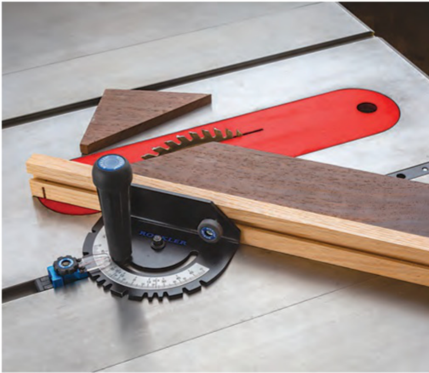
Two round knobs and T-bolts (included) enable scrap fences with T-slots to be installed on the gauge. Aside from their supportive benefits, these scrap fences also help to eliminate blade tearout during cutting.
