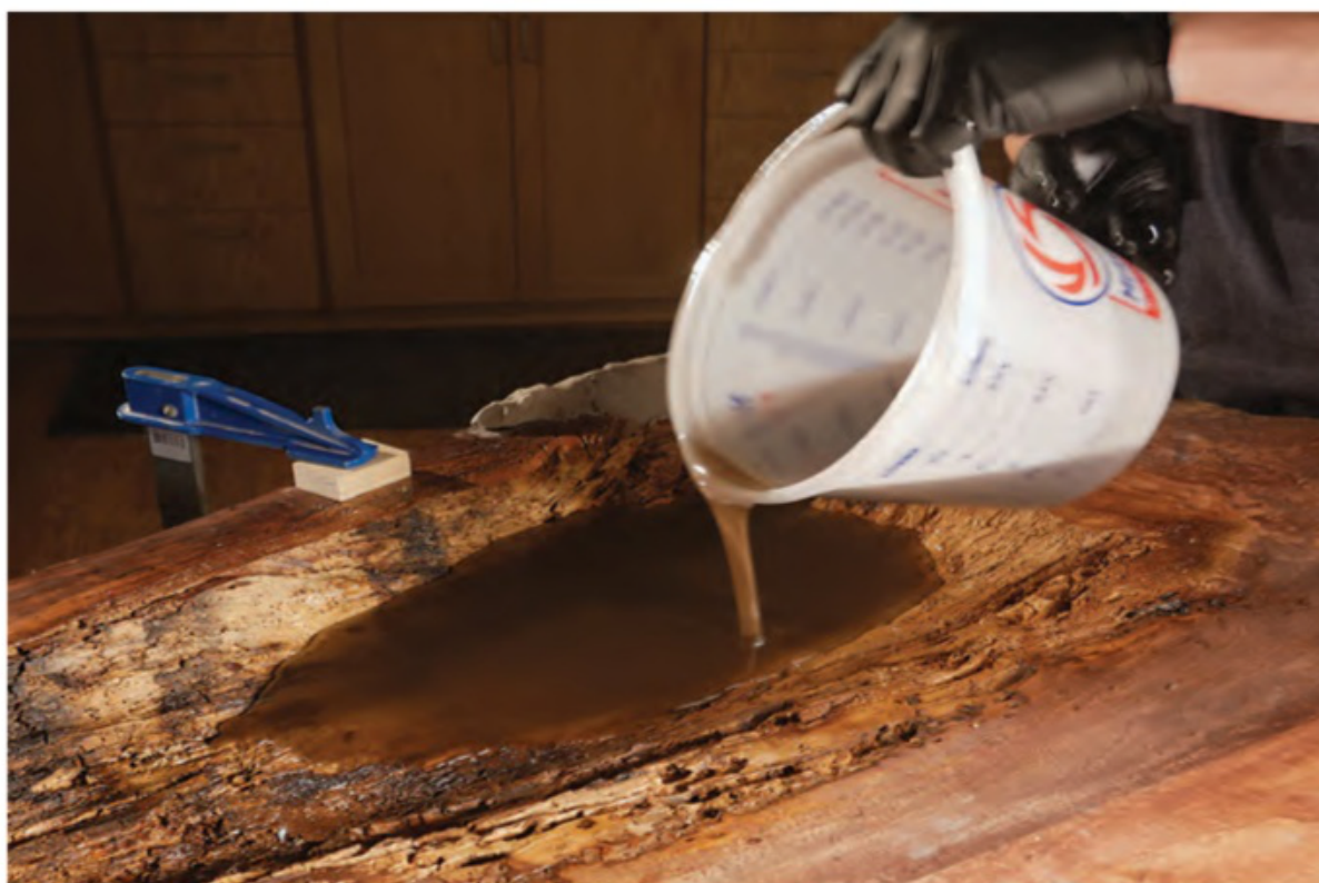
Mixol Universal Colorant was added to the epoxy mixture. The resin takes many hours to cure and even more time if the temperature is low. This long cure allows air bubbles to escape — important when pouring thick layers of resin. The last pour of clear resin, below, sealed in the punky grain.
