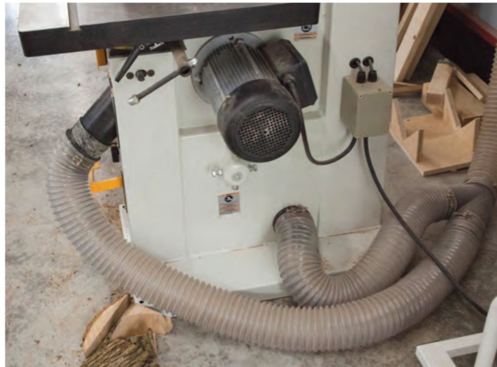
Modern band saws sport great dust collection. It's a big improvement in their design. This machine has two dust collection ports to catch most of the swarf generated below the saw table.
