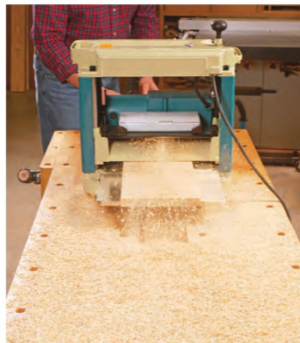
Without a chip hood in place and the machine connected to a shop vac or dust collector, a planer will quickly produce a flurry of chips and dust.
