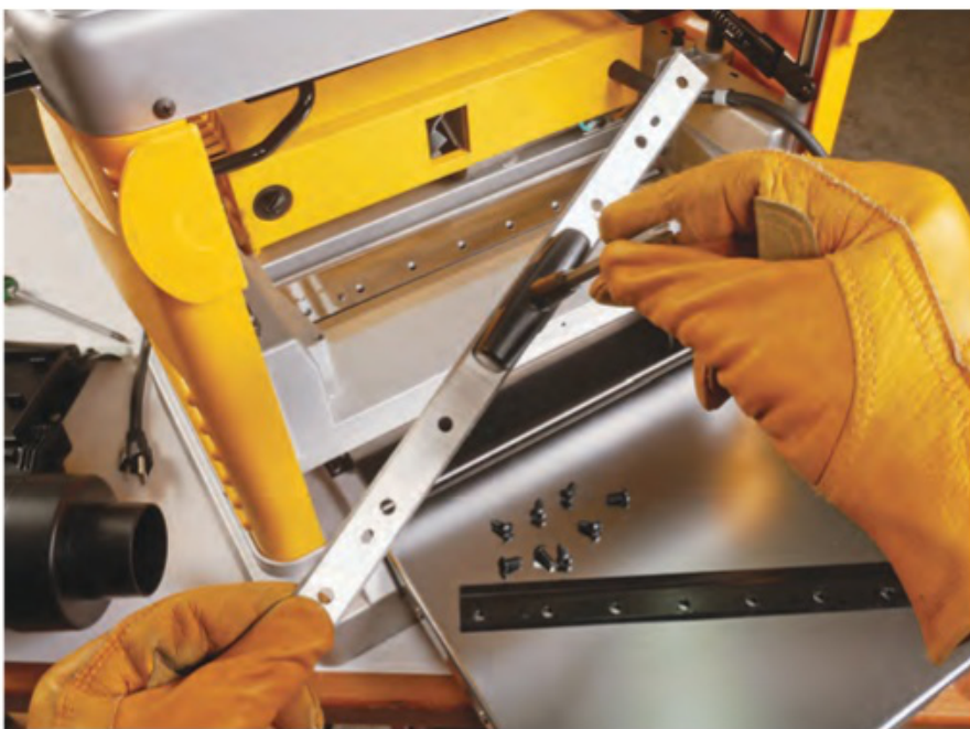
Double-edged disposable knives like these register on pins on the planer's cutterhead. When they dull, switching to the fresh edge is as easy as unbolting, flipping them around and reinstalling them on the index pins.
