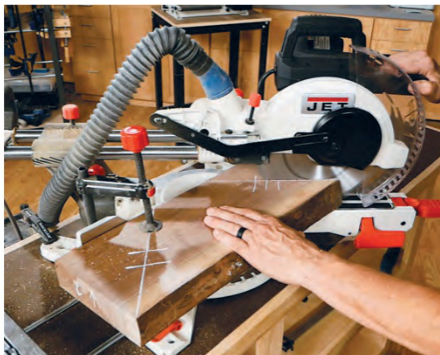
Cutting miter joints requires that the saw be carefully adjusted for accuracy, whether you use a miter saw like this or a miter gauge and table saw.
