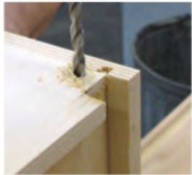
Once the locking devices were installed, marking a centerpoint in the drawer back for the slide's hook was a simple matter of engaging the slide hardware and bumping the hook against the drawer back (top inset). Drill the 1/4"-dia. hook holes 13/32" deep (bottom inset).
