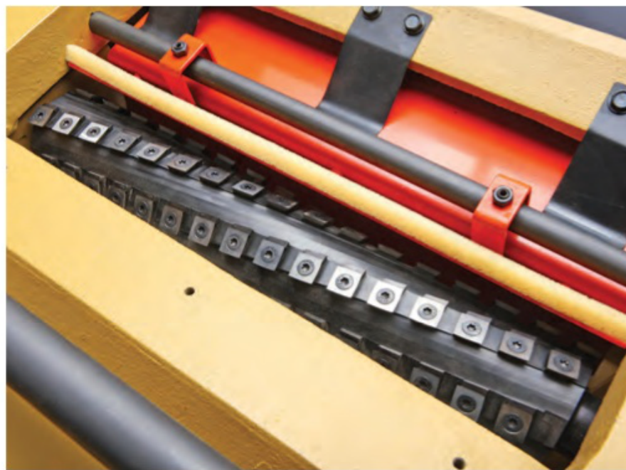
Helical cutterheads, equipped with rows of four-edged carbide inserts, are simple to maintain. Their shear-angled geometry also produces cleaner cuts — a big advantage on figured or interlocked wood grain.
