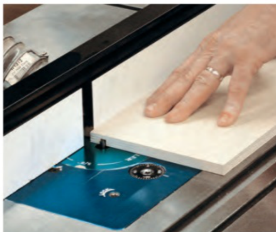
Plow 1/4"-deep, full-length grooves along the inside faces of the drawer front, back and side workpieces to fit the drawer bottoms.
