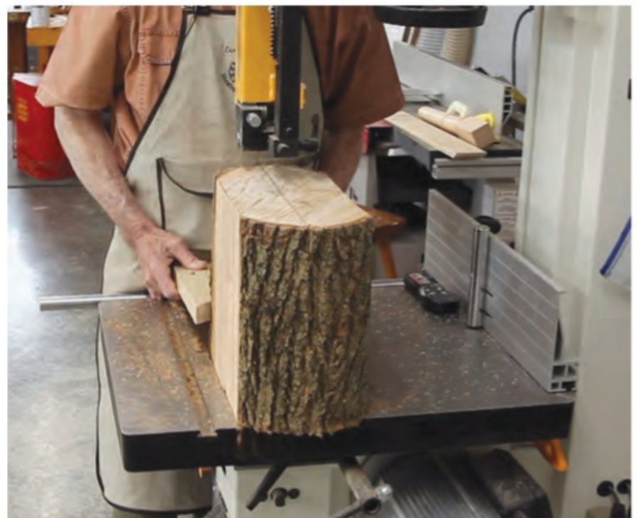
Saws with ample resawing capacity, powerful motors and the correct blade can easily handle the task of cutting a log section into thick planks for woodturning. The author recommends using a "V" push stick for this job.
