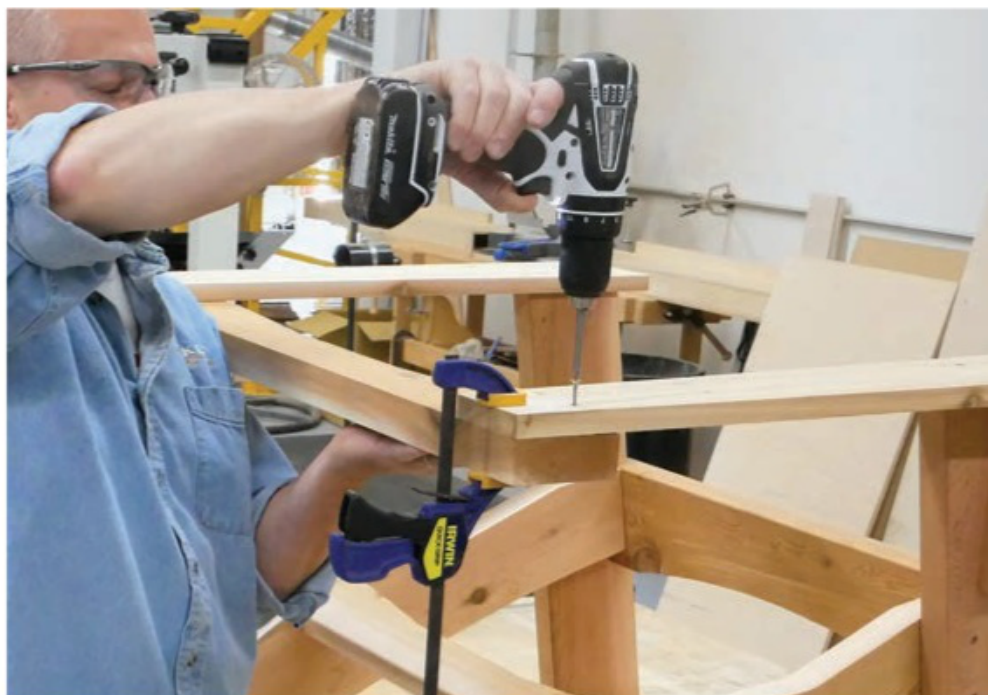
Clamp the middle back brace to the arms to form a subassembly. Drive countersunk screws down through the arms to fasten them to the front legs and arm braces. Once those are secured, attach the arms to the middle back brace with more screws.
