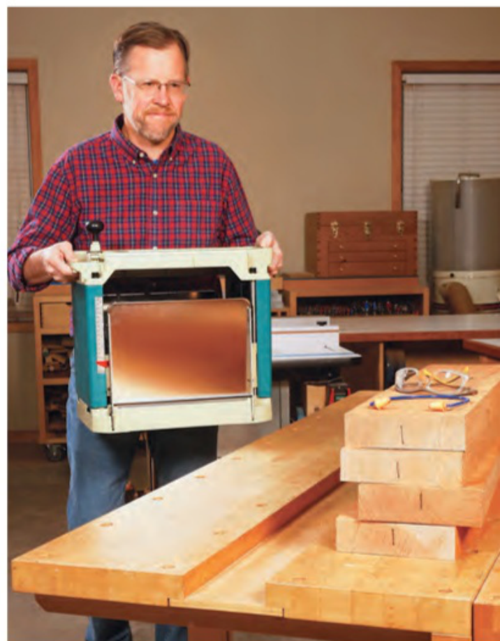
Portable benchtop planers are quite affordable, easy to store and capable of producing smooth, consistent results on both hard and softwoods.
