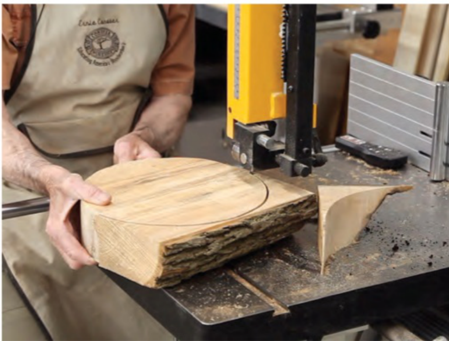
With the top and bottom faces of a plank flattened, a band saw can then make easy work of cutting the slab into round bowl blanks. Here's a task no other woodworking machine can match with equal finesse and safety.
