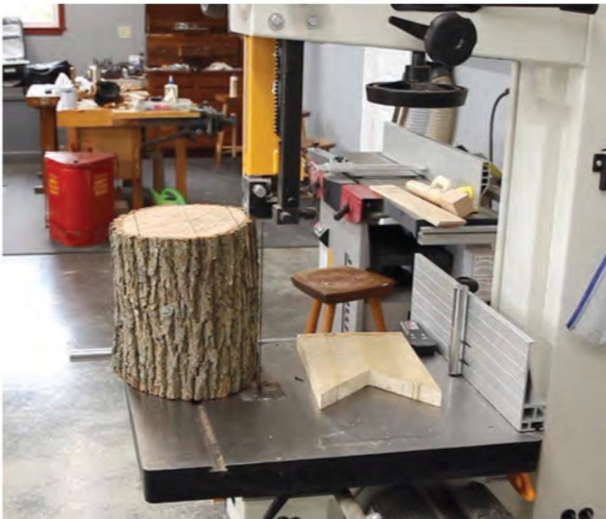
Large depth of cut on the author's RIKON band saw enables him to easily rip planks out of a section of log bucked to slightly longer than the diameter. Note the scrap-wood "V" push stick here.
