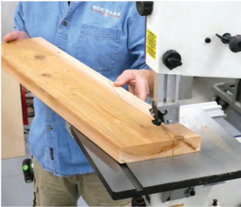
Use templates to trace outlines for the shaped parts onto your workpieces, then carefully cut them out on a band saw or with a jigsaw. Cut just outside of the layout lines.
