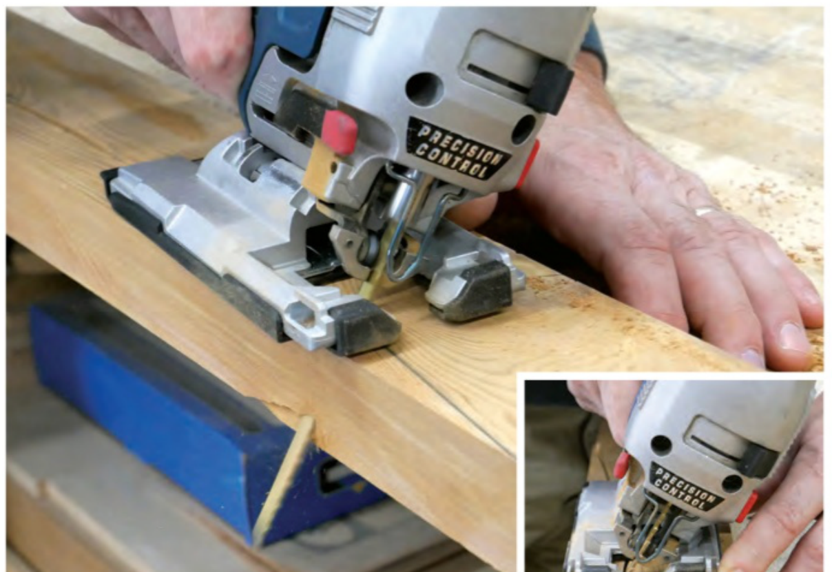
The front shaped edge of the middle back brace needs to be bevel-cut at a 30° angle to match the angle of the backrest. Cut this angled edge with your jigsaw's base tilted to 30° or using a band saw with the table tilted to 30°. Set up the cut so the blade angles out toward the part's front edge.
