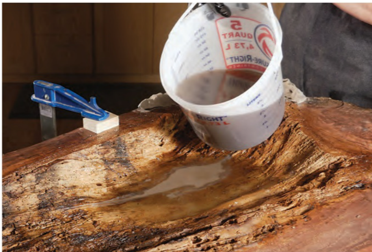
In order to successfully create thick layers of resin, the author chose MAS Deep Pour Epoxy. It allows 1" or even a bit thicker layers to be poured. While pouring the first layer here, a good bit leaked out. The next layers were more successful.
