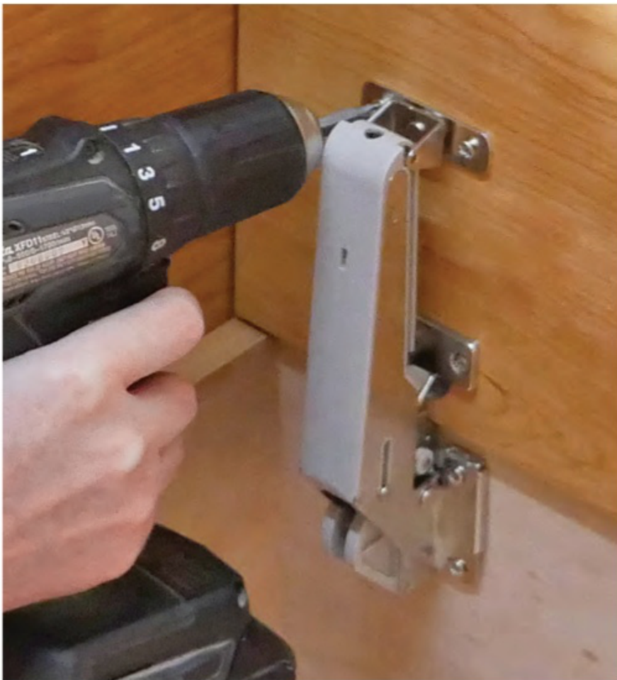
After the Aileron cup-style hinges are installed and adjusted on the chest and seat, a lid stay arm mounts on top of one hinge with a pair of brackets. This arm can be adjusted for the level of soft-close action you prefer.
