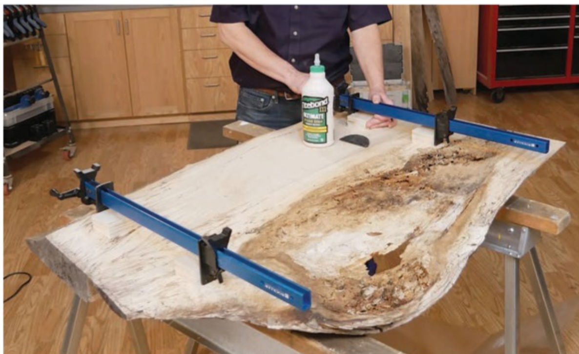
Making use of temporary clamping cauls glued to the tabletop, as well as loose tenons to help align the two pieces, gluing and clamping the tabletop components together was easy. When the glue dried, the author removed the clamping cauls and sanded the tabletop up to 220-grit.
