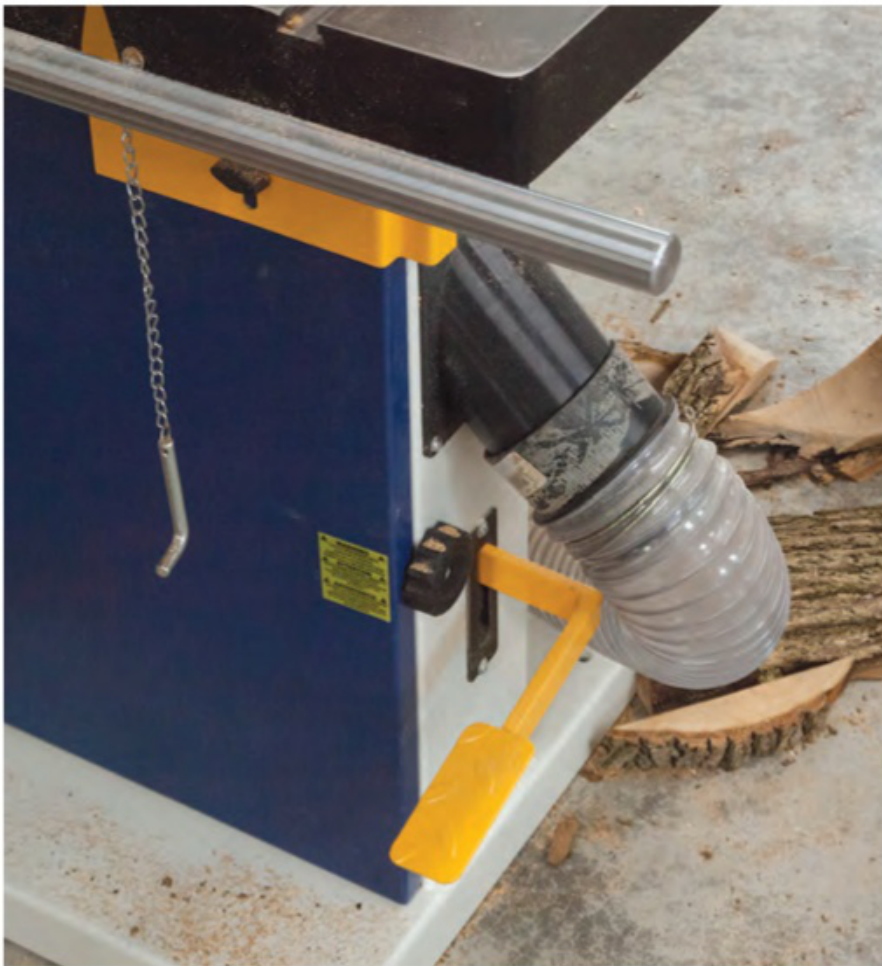
A foot brake near the floor allows the blade to be stopped quickly when needed. It also turns off the motor on most machines with magnetic start.
