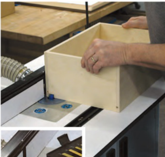
Each slide requires that a notch be cut through the drawer back, adjacent to the drawer side. We milled these left and right notches with a wide straight bit at the router table. Setting the bit and fence spacing accurately was easy, using a 1/2" brass setup bar (inset).
