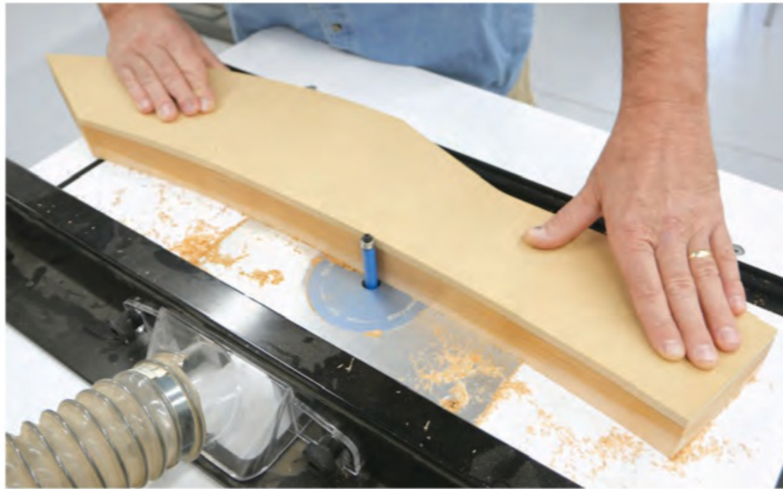
Here, an MDF template is affixed to a back leg workpiece with double-sided tape so the leg can be routed to an exact match with a piloted flush-trim bit. Alternatively, you could sand the chair parts to final shape instead of template-routing them.
