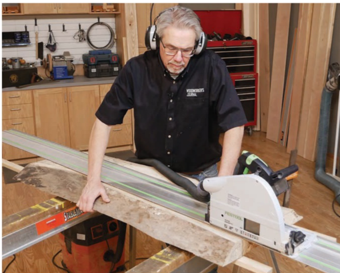
After crosscutting the big slab, the author used various methods to flatten and smooth the top and bottom faces of both pieces. Then, he cut away waste wood to form a center joint for the tabletop using a track saw to rip the edges straight. After this, the edges were further refined on a jointer.
