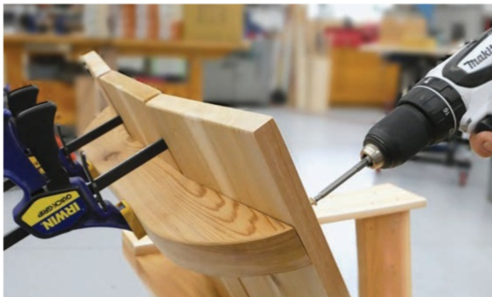
Spread the back slats 3/8" apart. Clamp the upper back brace to them, 3¼" down from their top ends. Secure it with three countersunk 1⅝" exterior screws driven through each back slat and into the brace.
