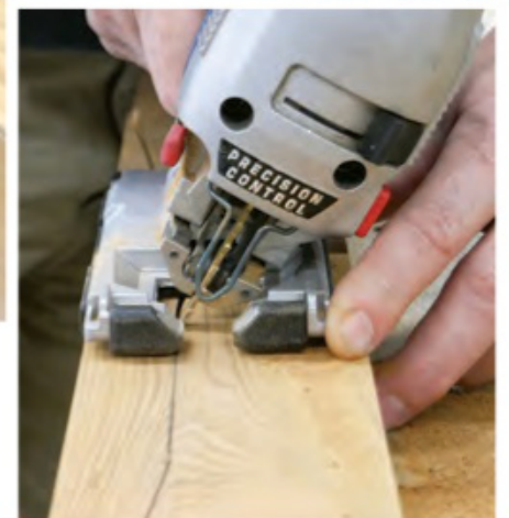
The front shaped edge of the middle back brace needs to be bevel-cut at a 30° angle to match the angle of the backrest. Cut this angled edge with your jigsaw's base tilted to 30° or using a band saw with the table tilted to 30°. Set up the cut so the blade angles out toward the part's front edge.
