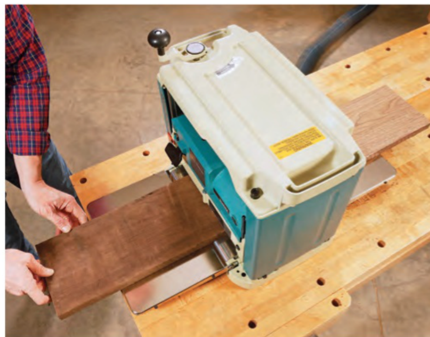
A benchtop or stationary planer enables you to take full advantage of roughsawn lumber options while enjoying its cost savings. It also gives you the ability to reduce stock to any thickness your project requires.
