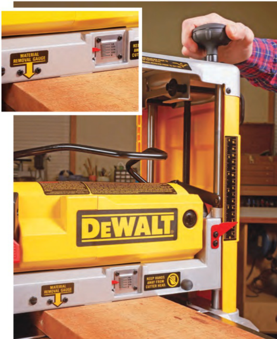
A hand crank dials in cutting depth, which is reported on a large scale on the machine's infeed side. Some planers also have a material removal gauge (inset) that reads cutting depth directly off the workpiece.
