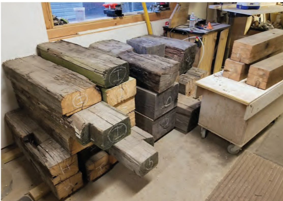
Lockman Hardwoods of Elmer, New Jersey, provided the timbers, which were allowed to acclimate for more than six months in the Random 8 shop. They were extracted from various structures, including a now-raised cathedral, a train station, corn crib and 18th-century home.
