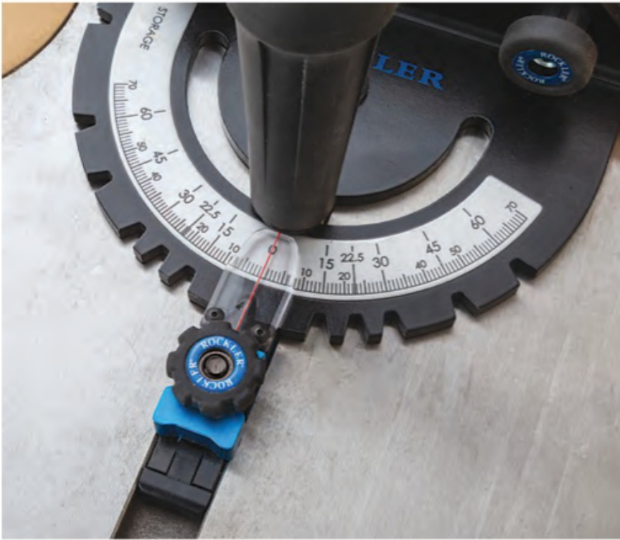
Eleven preset detents lock the gauge to common miter angles. Loosening the round, low-profile knob and pulling it back releases the blue stop for changing settings. A twelfth detent provides for compact storage (below).
