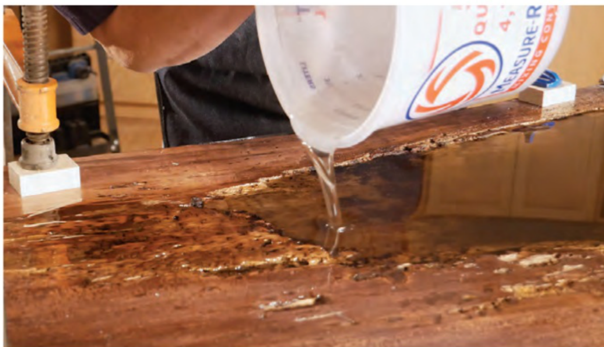
Mixol Universal Colorant was added to the epoxy mixture. The resin takes many hours to cure and even more time if the temperature is low. This long cure allows air bubbles to escape — important when pouring thick layers of resin. The last pour of clear resin, below, sealed in the punky grain.
