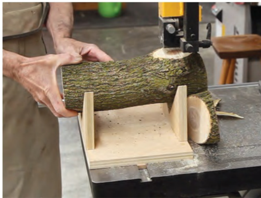
A shop made V-block sled, which rides on a rail in the saw's miter slot, immobilizes logs for crosscutting into round sections. This is the only safe way to crosscut round stock on a band saw. Make one for your saw.
