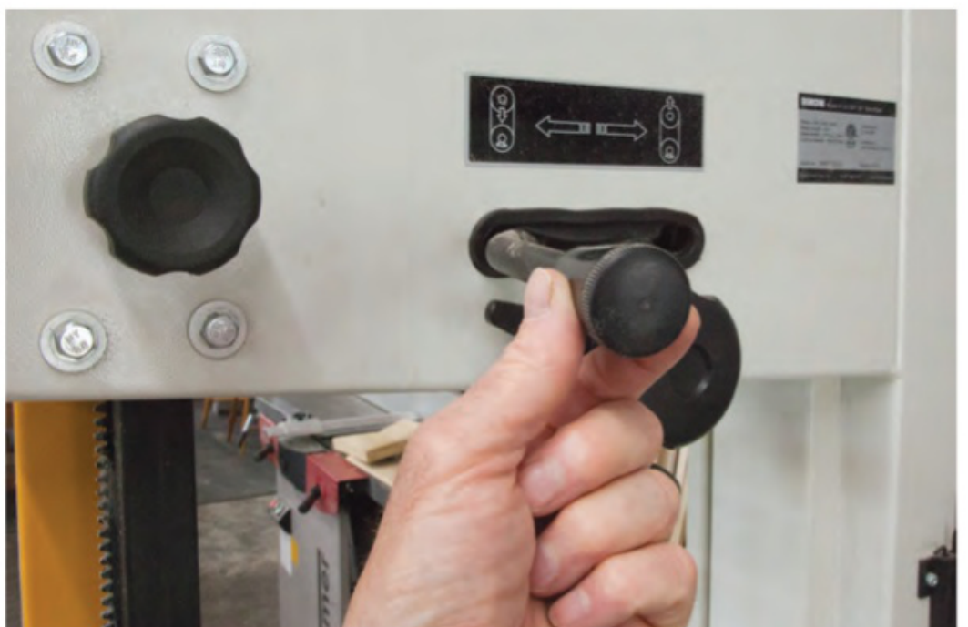
A de-tensioning lever releases blade tension, thereby extending the life of the tires and making blade changes a breeze. It's become a common feature on newer band saws.
