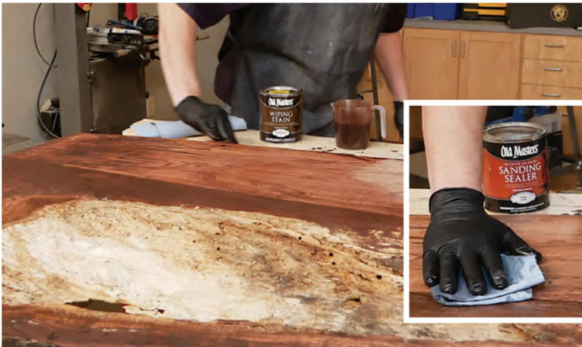
The first finishing step involved wiping the maple with thinned stain. Notice how the stain absorbed differently on either side of the center glue joint. Glazing the top with full-strength stain over a base coat of polyurethane solved this color mismatch.
