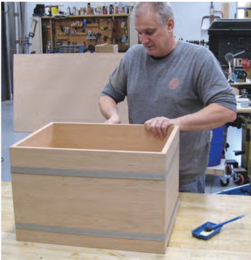
Glue and clamp the chest's front, back and side panels together with the bottom in place. For this glue-up, strap clamps will keep the bevel joints from slipping out of alignment while under pressure.
