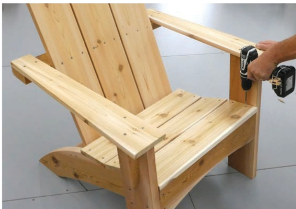
Install the three seat slats on the back legs. Position the front slat so it overhangs the front cross brace by about 1/4", and spread the other two slats evenly apart. Attach the seat slats to the back legs with 1⅝" screws, using two screws per joint.
