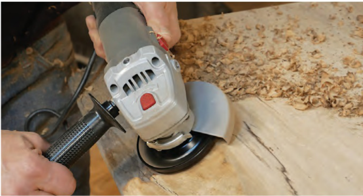
Removing darkly weathered wood fibers from the tabletop's wane edge produced a better surface for finishing while also adding texture. A power-carving blade made short work of the effort. It was also used to shape the front edges to match.
