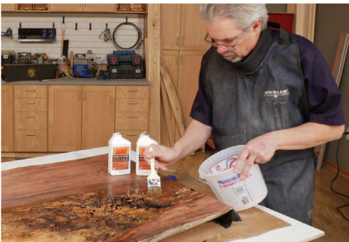
MAS Penetrating Epoxy Sealer was applied to the punky grain and all around the exposed fibers of the "pond." It was important to seal both faces of the tabletop with this product to reduce resin leakage later on.
