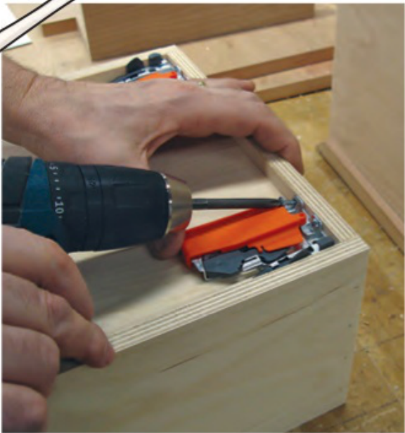
A pair of plastic and metal locking devices fit behind the drawer fronts and against the bottom panels. Attach them with short screws.
