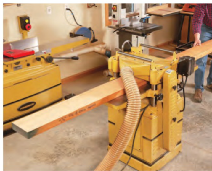
Thanks to their mass and power, floor-standing stationary planers are ideal for surfacing long, heavy material, like this plank of 8/4 mahogany.
