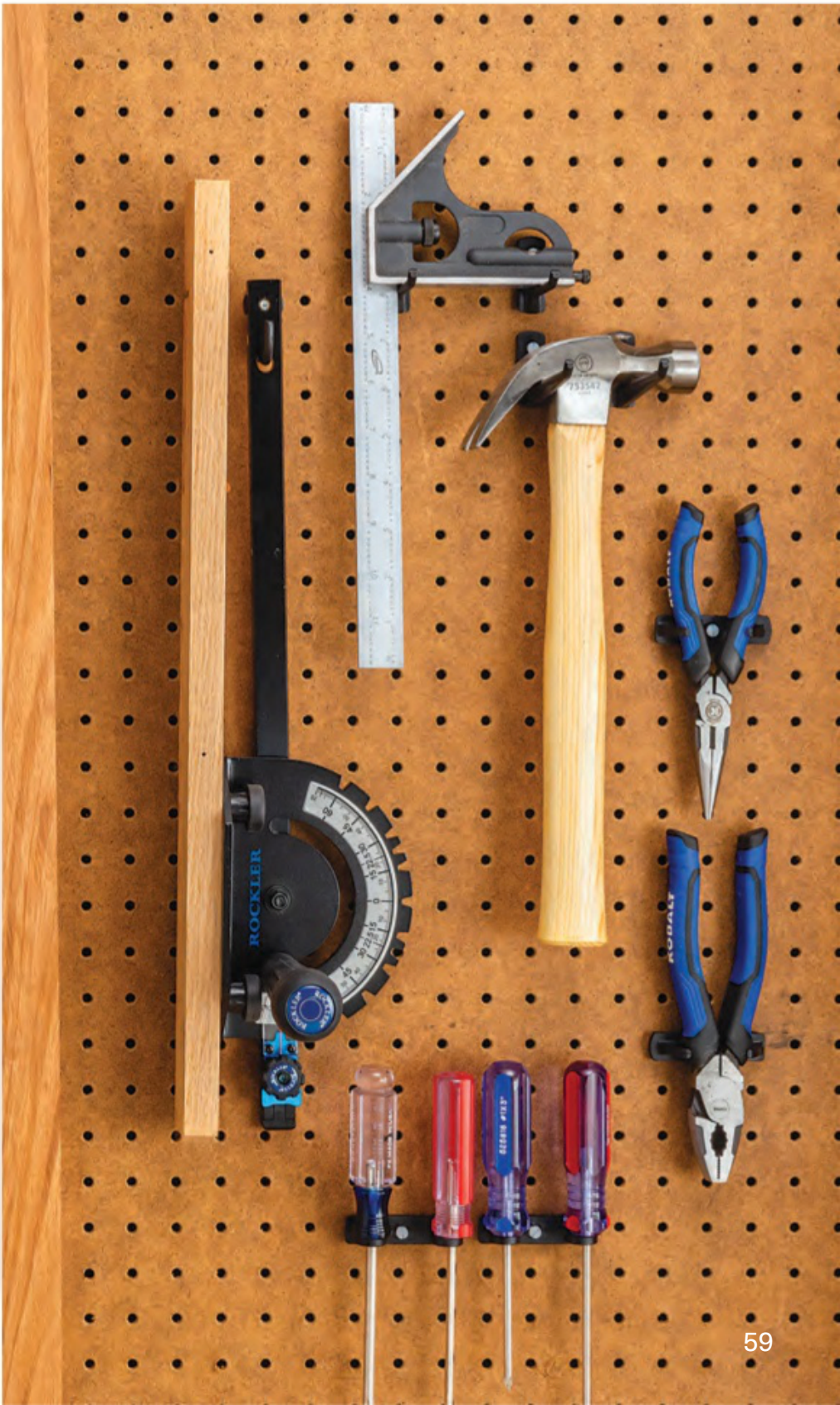
Eleven preset detents lock the gauge to common miter angles. Loosening the round, low-profile knob and pulling it back releases the blue stop for changing settings. A twelfth detent provides for compact storage (below).
