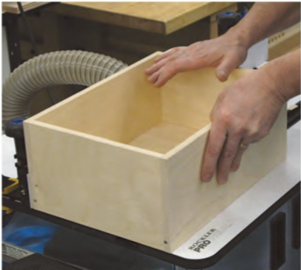
Each slide requires that a notch be cut through the drawer back, adjacent to the drawer side. We milled these left and right notches with a wide straight bit at the router table. Setting the bit and fence spacing accurately was easy, using a 1/2" brass setup bar (inset).
