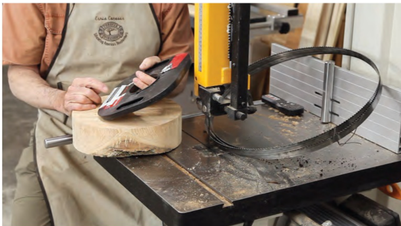
A 3/4"-wide by 3 tpi blade (coiled at right in photo) is ideal for resawing. For general cutting, however, the author buys 100' coils of 3/8"-wide, 4 tpi blade stock and brazes it into 162" lengths for his 18" RIKON band saw.
