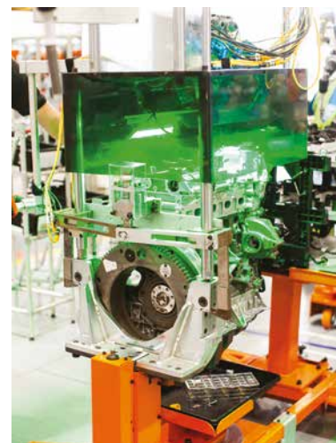
Opposite page: A Ford diesel engine slowly starting its way down the assembly line. Left and above: Ford's Struandale plant is full of sophisticated, high-tech equipment, ensuring every engine is built to the highest standards. Below: In order to cold test an engine, all of these connections had to be plugged into every unit that came down the line.
