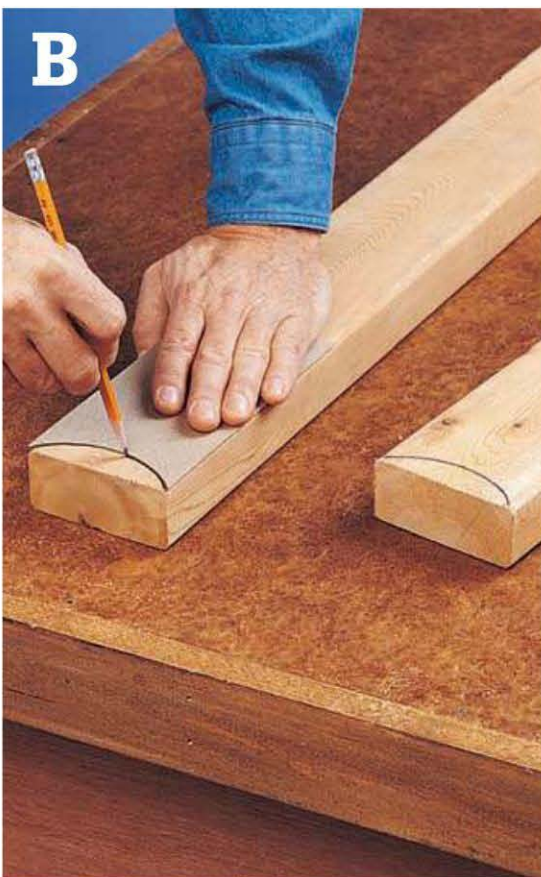
A piece of cardboard acts as a template when you trace the outline for the arc on the cross beams.
