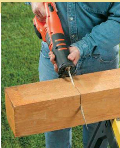
A reciprocating saw with a long, woodcutting blade makes it easy to cut through posts in a single pass. Be careful to keep the saw steady and level to ensure a straight cut.
