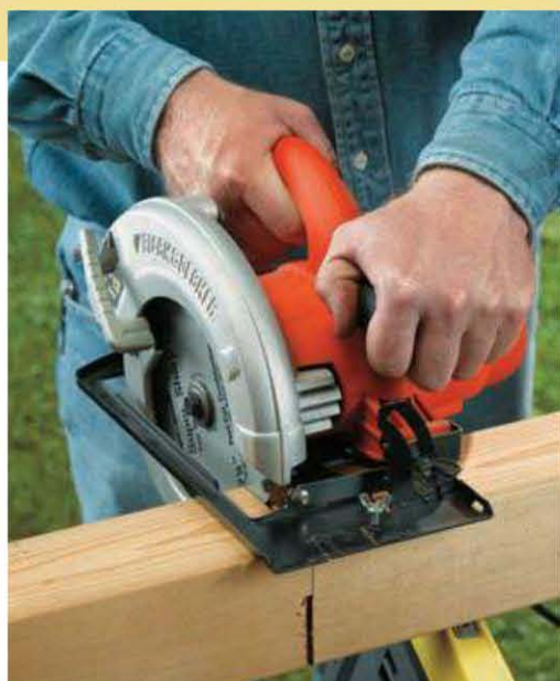
When cutting with a circular saw, set the saw blade to maximum depth. Cut all the way around the post, moving from one side to the next. Be careful to stay on your cutting lines, so the cut surface will be flat. On a 6 × 6, you can cut all four sides, then finish off the center with a handsaw. Because a handsaw blade is thinner than a circular saw blade, keep the handsaw flat against the wood as you cut.
