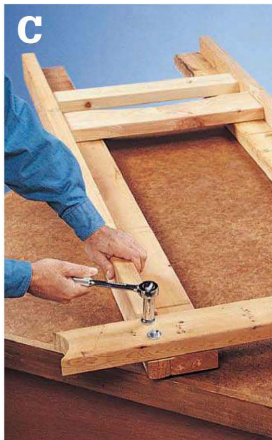
Lag-screw the cross beams to the legs, and fasten the spreaders and rails with deck screws to assemble the side frames.
