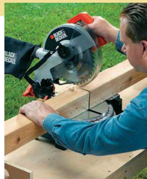
Power miter saws are the easiest tool for cutting 4 × 4s on a workbench and don't require a continuous cutting line. To cut a 6 × 6—if your saw can accommodate one—set up a stop block. This allows you to evenly rotate the post, cutting from all sides.
