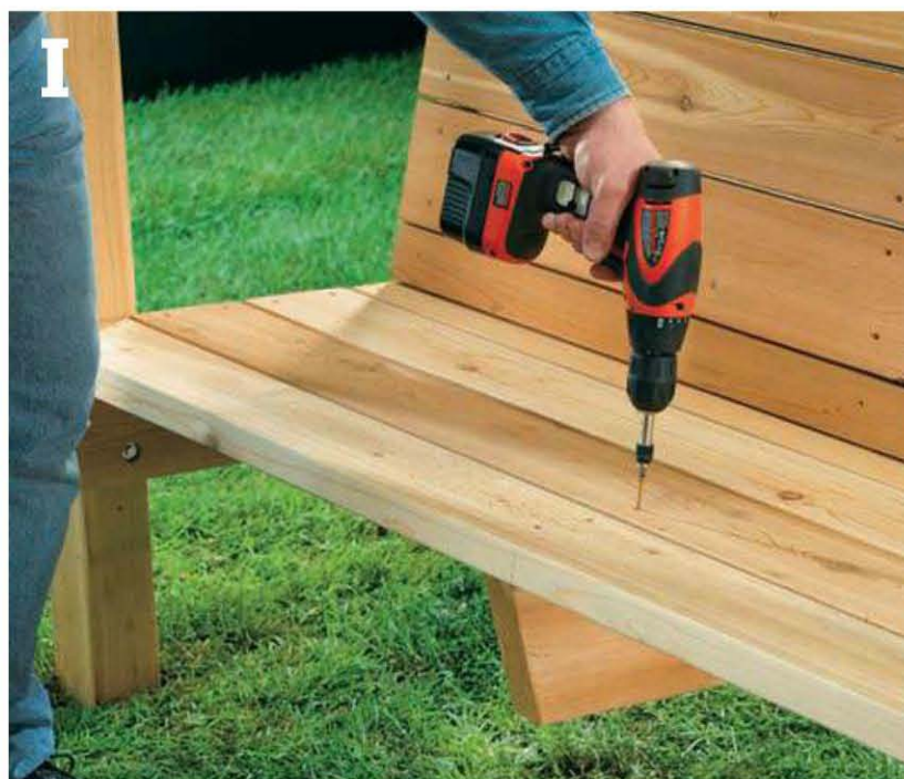
Install the center support so it's centered along the length of the seat slats.
